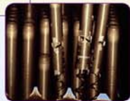
Fuel Assembly Damage due to Baffle Jetting
