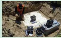
Fig. 1 - Excavation of test pit at Falls City. Fig. 2 - Profile of materials in a test pit and test of radon flux from the underlying mill tailings. Fig. 3 - Flux data for the four sizes of flux chambers at each test pit at Falls City. Fig. 4 - Four flux chambers of different sizes. (counter-clockwise from top left)
