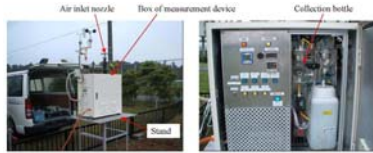
Outside view Inside view Size(Box of measurement device): 700 × 700 × 400mm Weight: 60 kg Power supply: 100V (20A)
