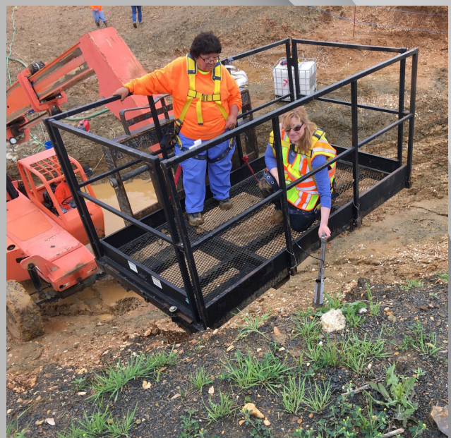
Region IV Health Physicist Linda Gersey (right) conducts radiological surveys and collects soil samples at the Sequoyah Fuels plant near Gore, Oklahoma. This site is undergoing decommissioning.
