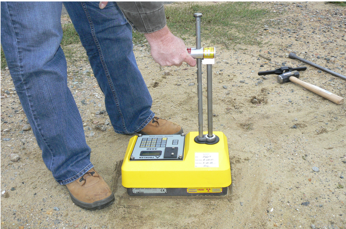
A moisture density gauge indicates whether a foundation is suitable for constructing a building or roadway. Courtesy of APNGA
