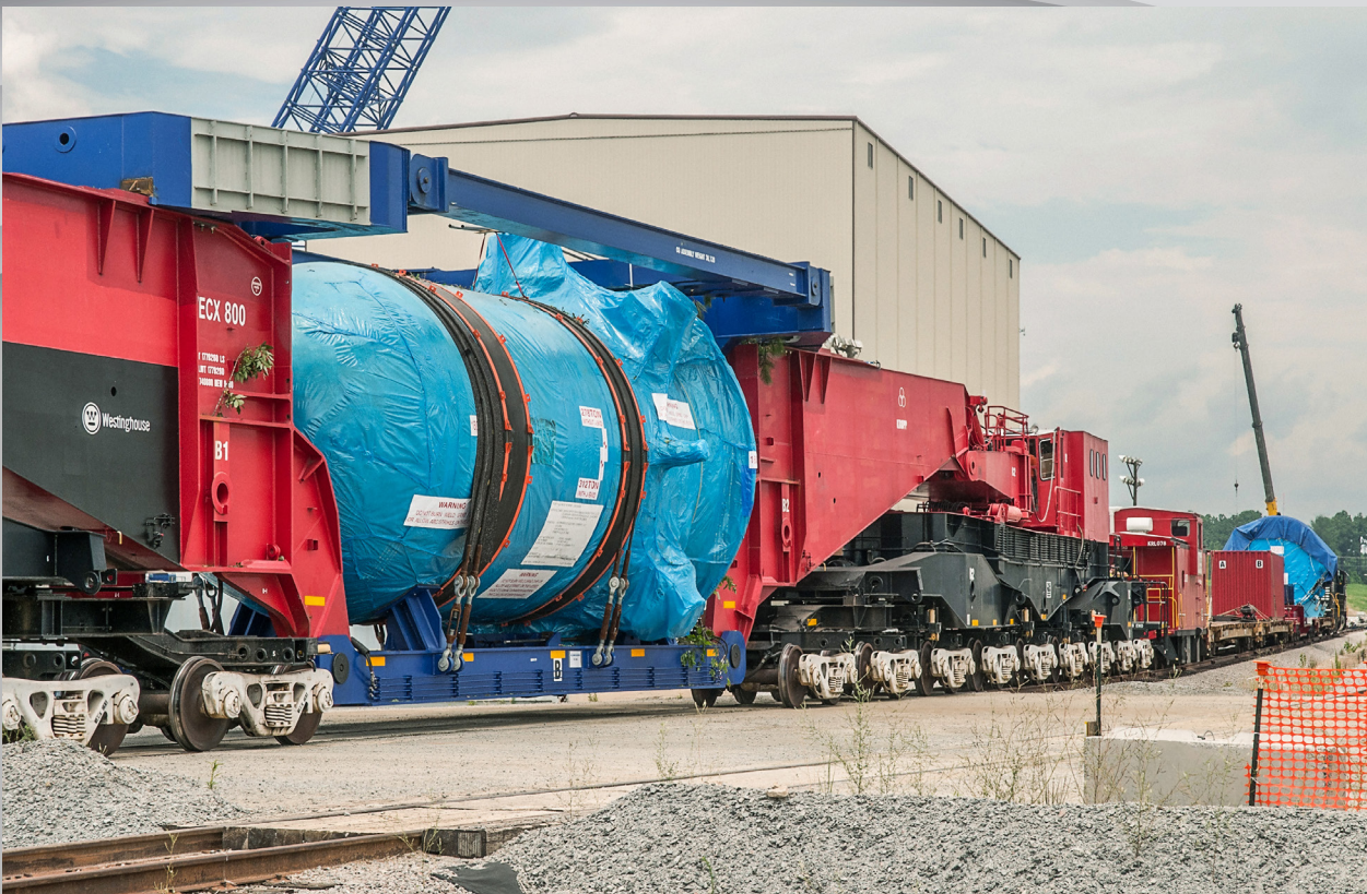
The reactor vessel and vessel head arrive at the V.C. Summer site South Carolina. The parts traveled by rail from the Port of Charleston by rail and on a Schnabel car—a specialized freight car designed to carry heavy and oversized loads. Courtesy of SCANA/SCE&G.
