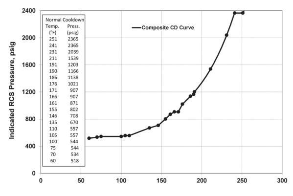
The regions of acceptable operation are below and to the right of the limit curves. Margins are included for the pressure differential between point of system pressure measurement and the pressure on the reactor vessel region controlling the limit curve. Margins for instrument error are not included.
