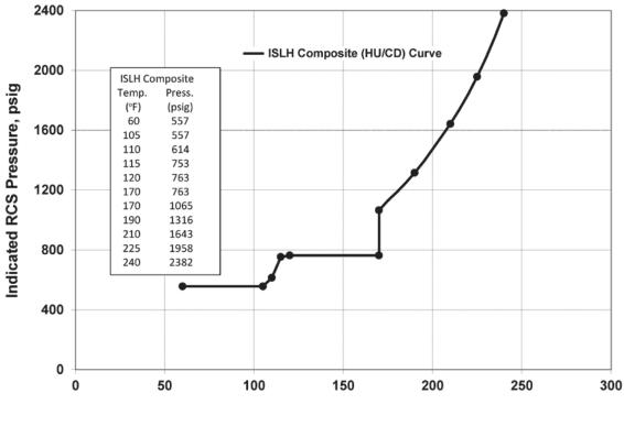
The regions of acceptable operation are below and to the right of the limit curves. Margins are included for the pressure differential between point of system pressure measurement and the pressure on the reactor vessel region controlling the limit curve. <u>Margins for instrument error are not included</u>.
