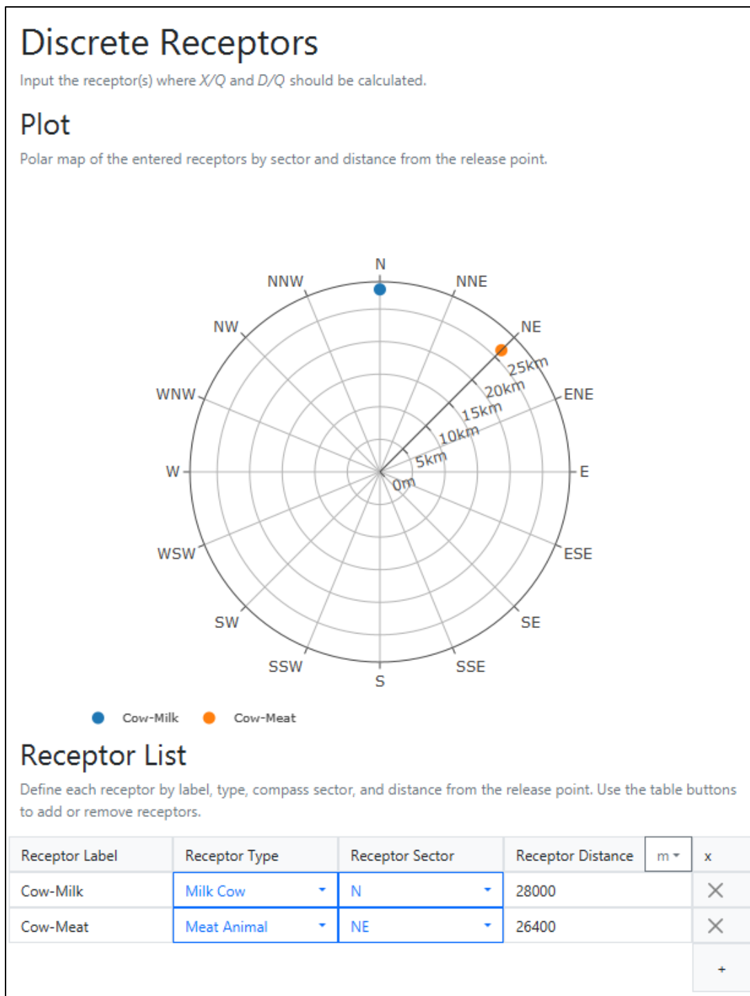
Figure 7-4. Managing discrete receptors for Routine Release module.
