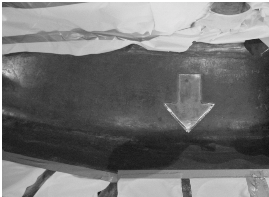
Figure 4 Photograph showing alignment arrow for setting head on vessel - arrow is machined into scan area of head adjacent to weld.
