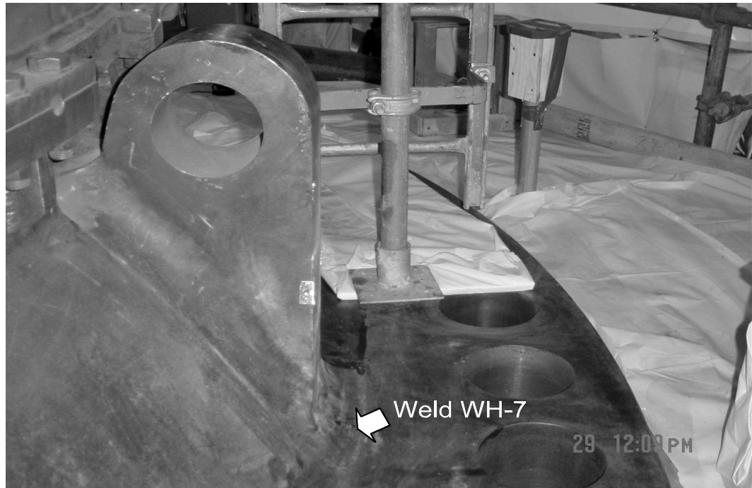
Figure 3 Photograph showing how lifting lugs limit ultrasonic scans from head side of Weld WH-7.
