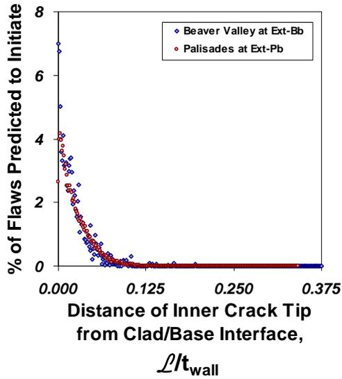
Figure 4-3 Distribution through-wall position of cracks that initiate
