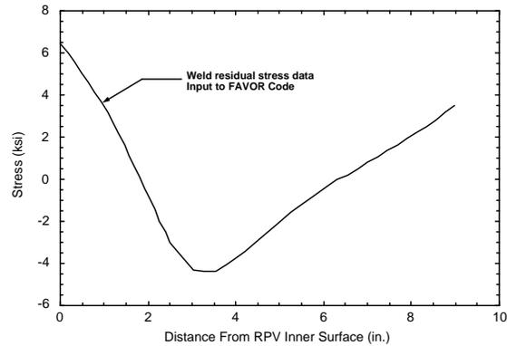
**Figure 4-7 Through-thickness weld residual stress profile assumed by FAVOR**
