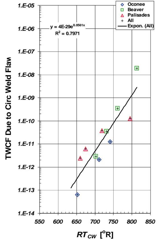
Figure 2-1 Correlation of through-wall cracking frequencies with reference temperature metrics for the three study plants ( $^{\circ}R = ^{\circ}F + 459.69$ ) reported in NUREG-1806 [20]
