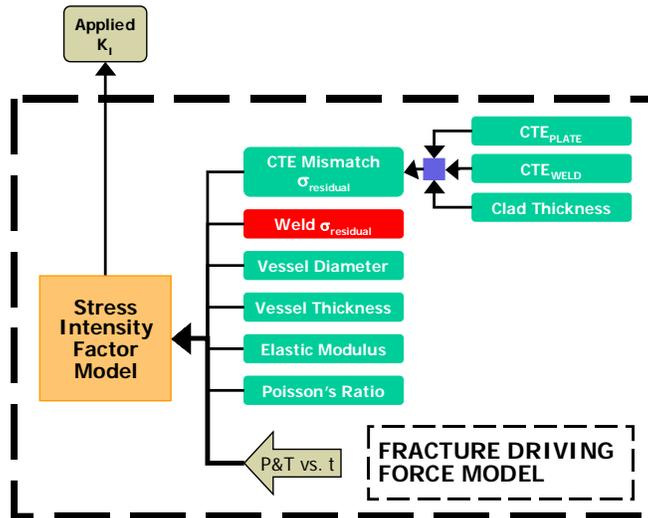
Figure 4-11 Crack driving force model for through-wall cracking
