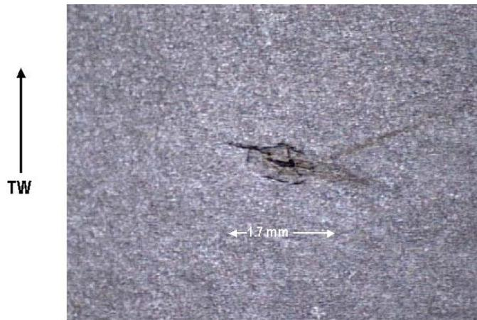
**Figure 1 Small Flaw in Plate Material**
