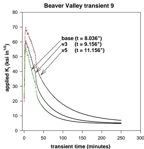
**Figure 5-2 Effect of vessel wall thickness on the variation of applied- $K_I$  vs. time for a 16-in. diameter hot-leg break in Beaver Valley. The flaw has the following dimensions:  $L=0.35$  in.,  $2a=0.50$  in.,  $2c=1.5$  in.**
