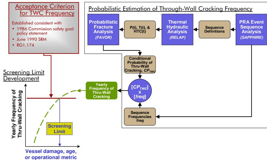
**Figure ES-2 Schematic showing how a probabilistic estimate of through-wall cracking frequency (TWCf) is combined with a TWCf acceptance criterion to arrive at a proposed revision to the PTS screening limit**
