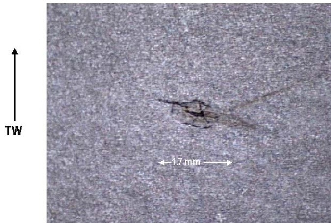
Figure 1 Small Flaw in Plate Material
