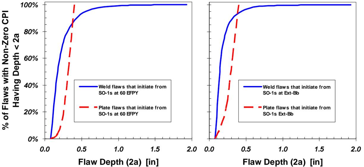
**Figure 4-5 Flaw depths that contribute to crack initiation probability in Beaver Valley Unit 1 when subjected to medium stuck-open valve transients at two different embrittlement levels**
