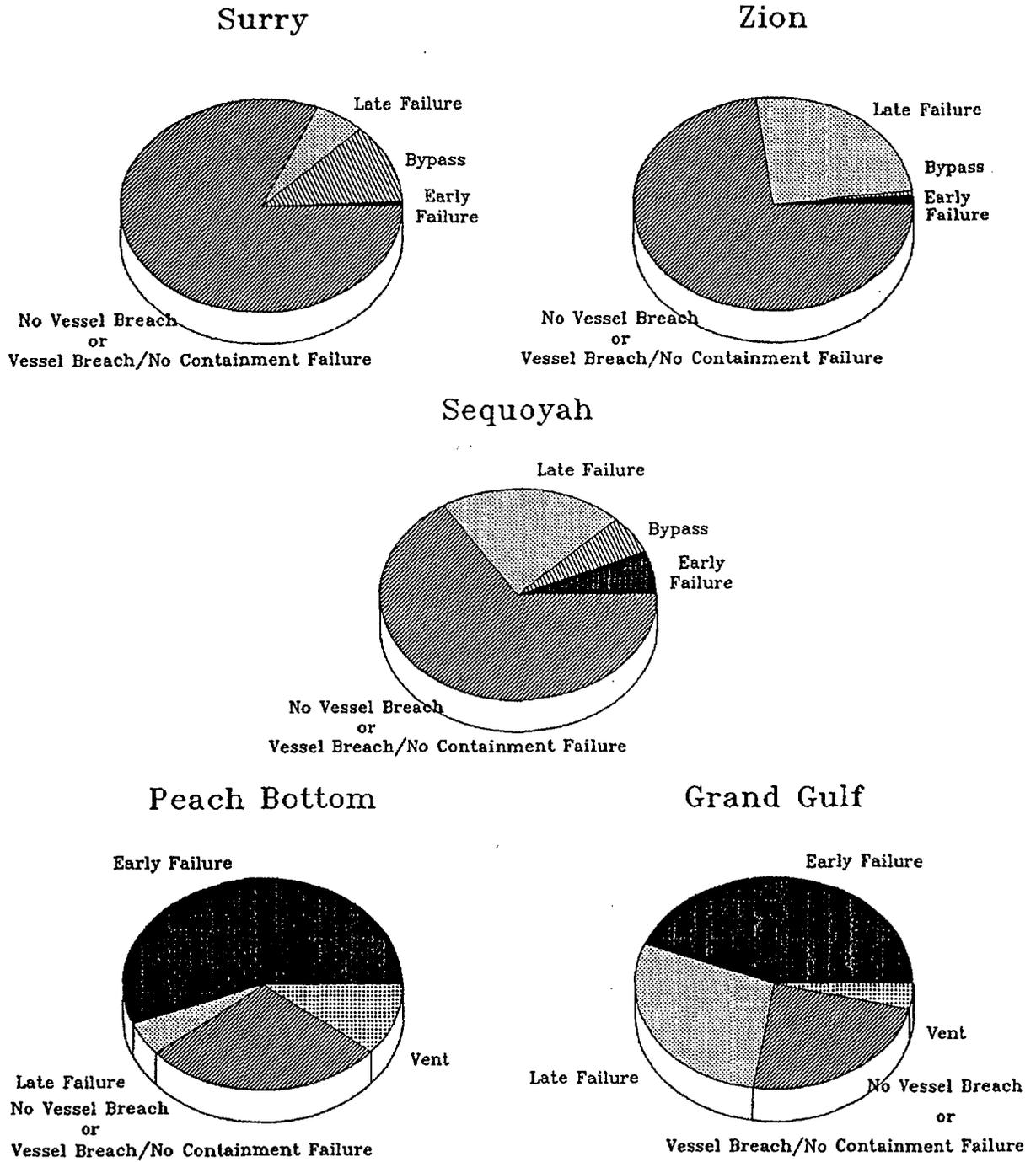
Figure 9.4 Relative probability of containment failure modes (internal events).
