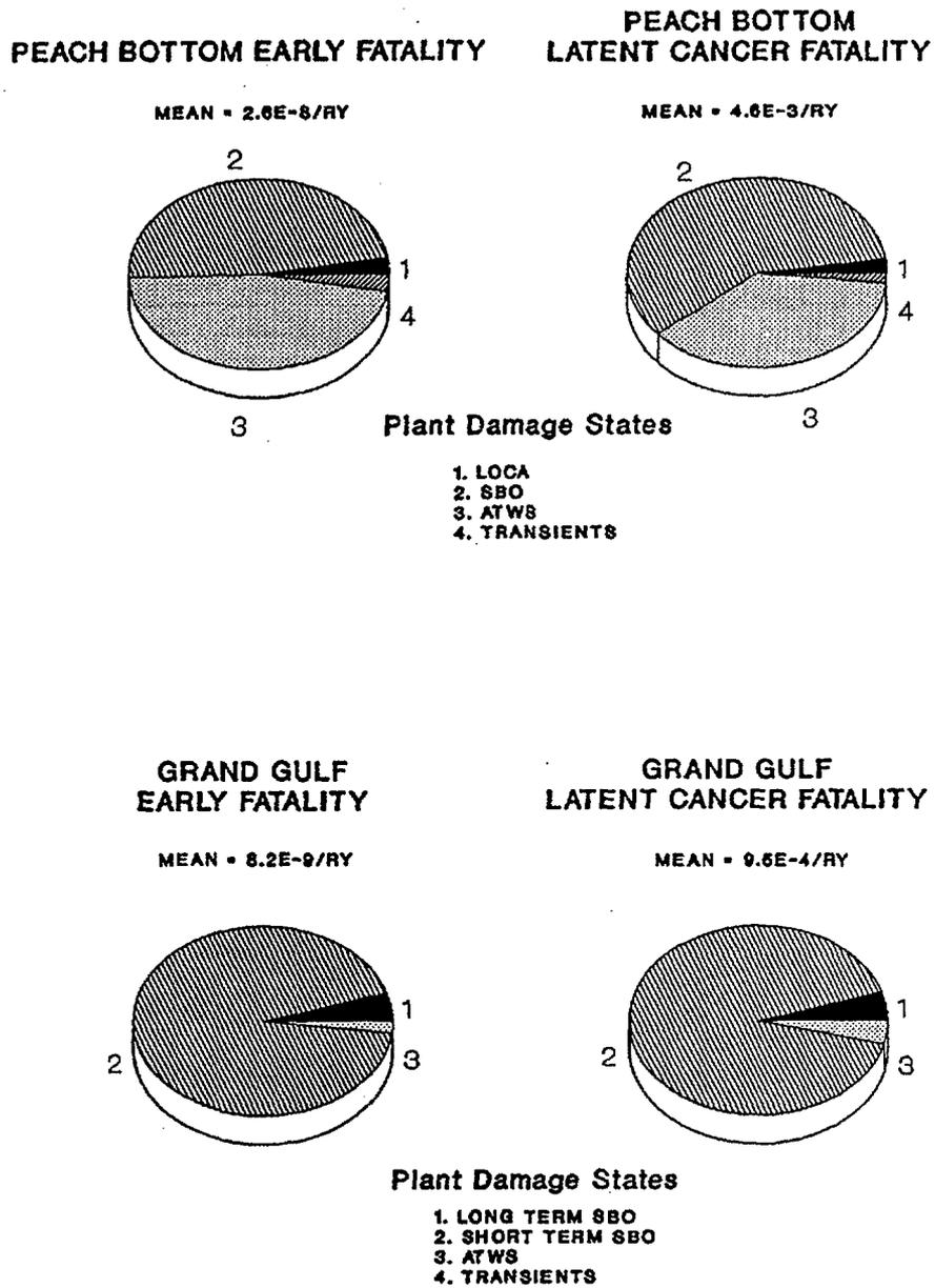
Figure 12.7 Contributions of plant damage states to mean early and latent cancer fatality risks for Peach Bottom and Grand Gulf (internal events).
