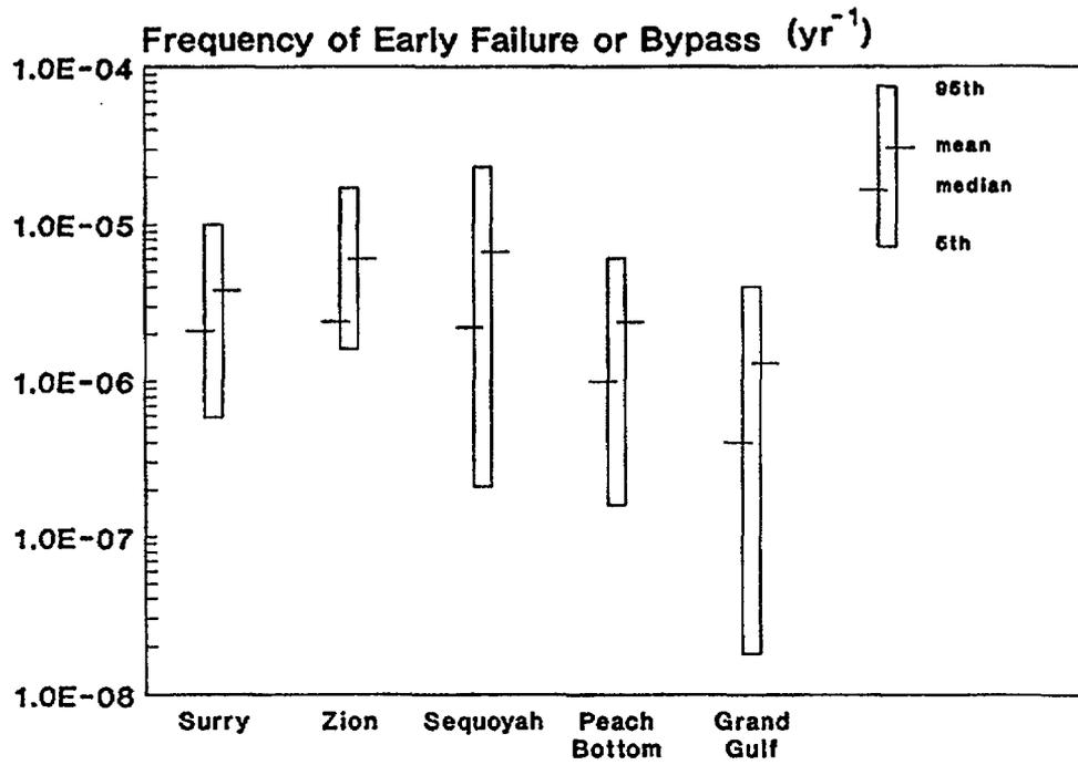
Figure 9.3 Frequency of early containment failure or bypass (all plants).
