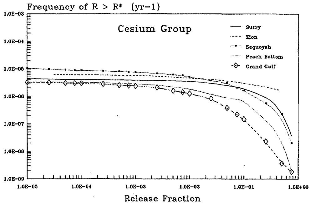
Figure 10.1 Frequency of release for key radionuclide groups.
