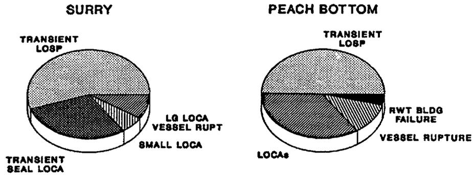
Figure 8.9 Principal contributors to seismic core damage frequencies.
