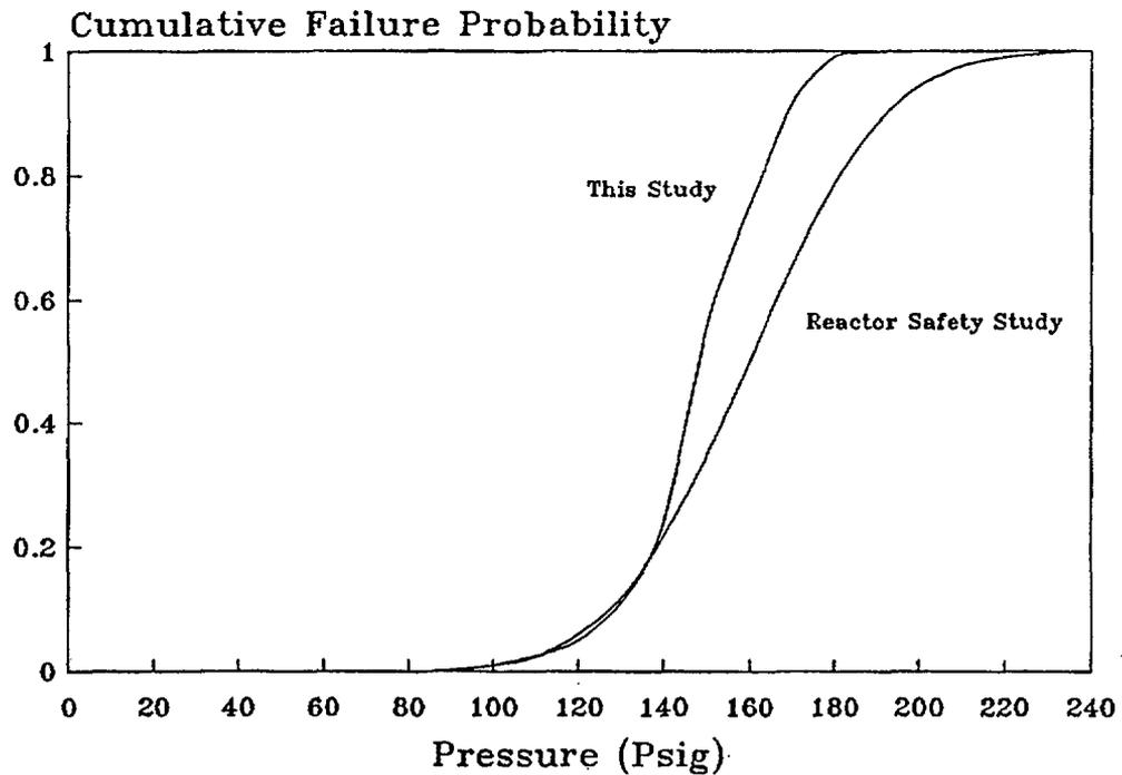
Figure 9.7 Comparison of containment failure pressure with Reactor Safety Study (Peach Bottom).
