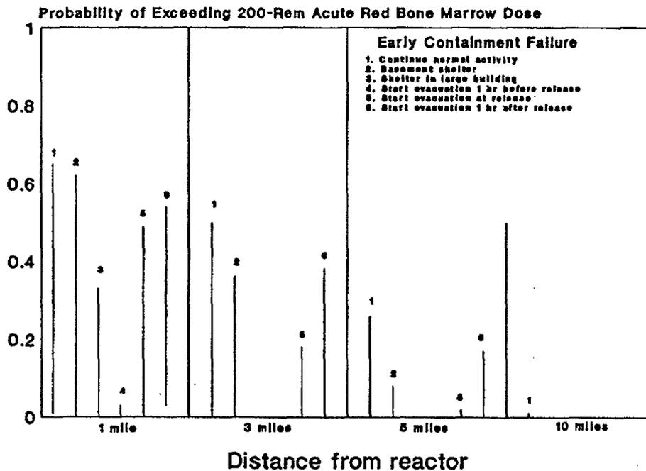
Figure 13.5 Relative effectiveness of emergency response actions assuming early containment failure with high and low source terms.
