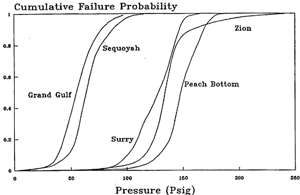
Figure 9.9 Cumulative containment failure probability distribution for static pressurization (all plants).
