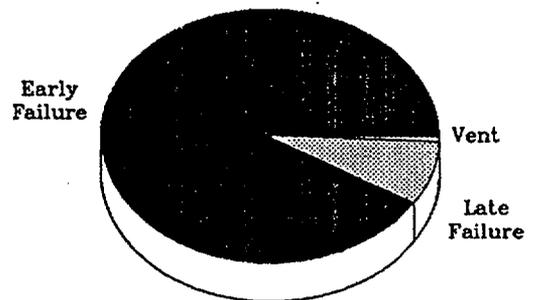
Figure 9.5 Relative probability of containment failure modes (internal and external events, Surry and Peach Bottom).
