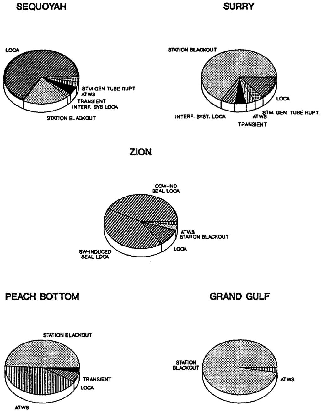
Figure 8.4 Principal contributors to internal core damage frequencies.
