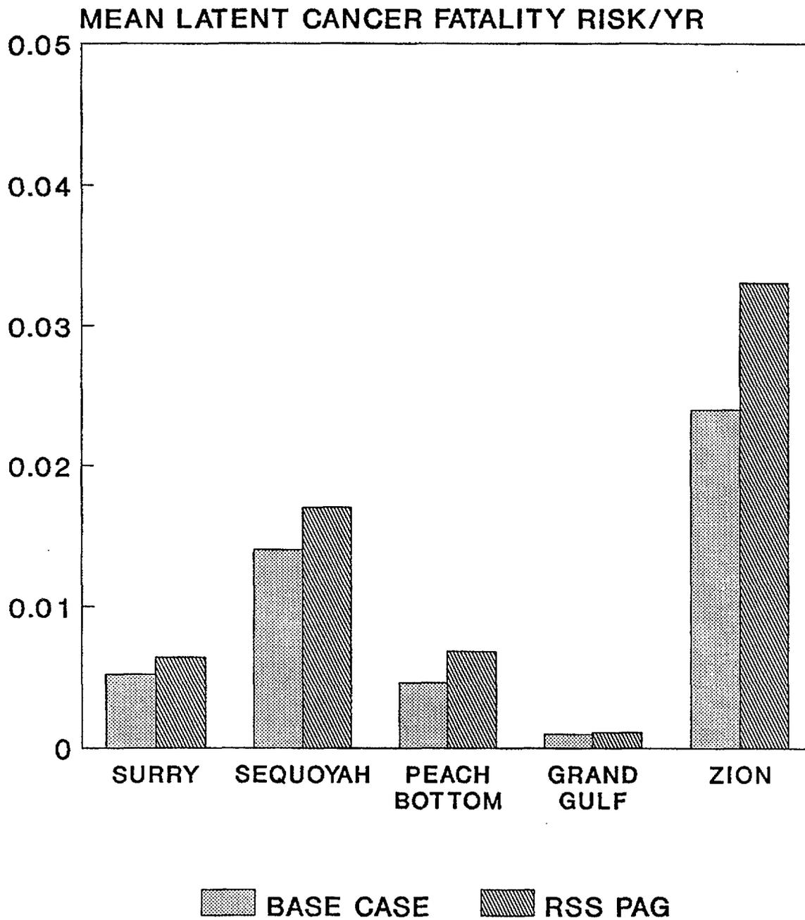
Figure 12.12 Effects of protective action assumptions on mean latent cancer fatality risks at all plants (internal events).
