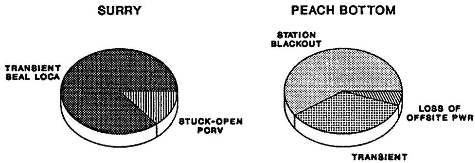
Figure 8.10 Principal contributors to fire core damage frequencies.
