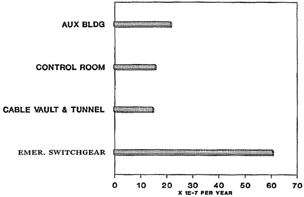
Figure 8.11 Surry mean fire core damage frequency by fire area.
