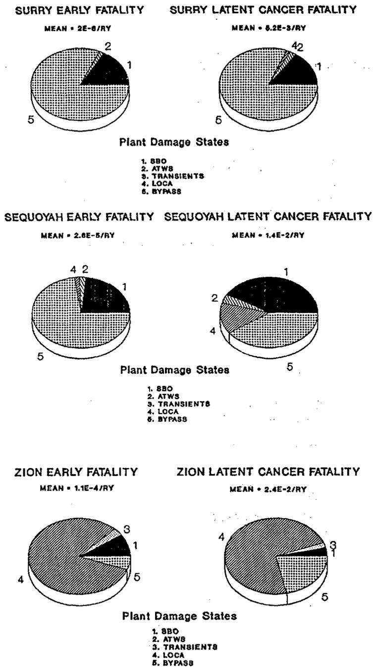
Figure 12.6 Contributions of plant damage states to mean early and latent cancer fatality risks for Surry, Sequoyah, and Zion (internal events).
