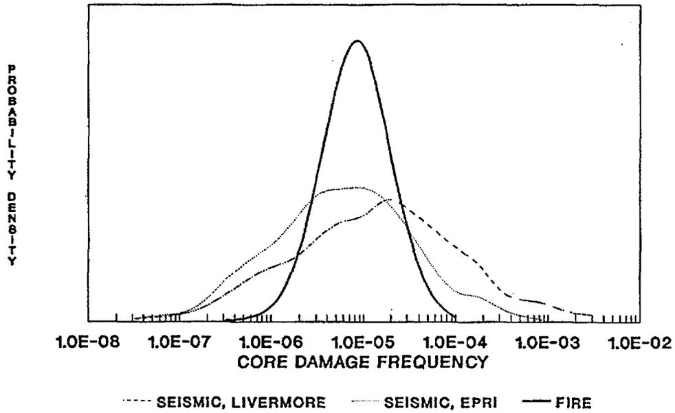
Figure 8.5 Surry external-event core damage frequency distributions.
