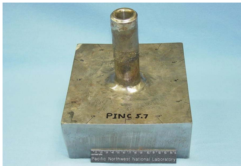
Figure 2.17 PINC 5.7 from PNNL – WNP-1 BMI Nozzle Penetration 1
