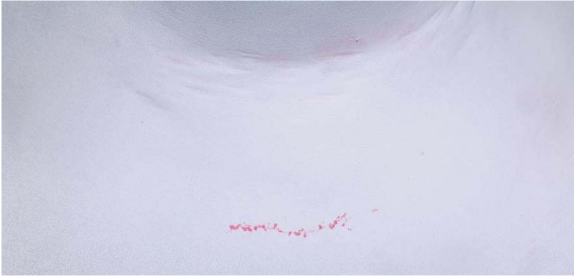
Figure 2.58 Example of Laboratory-Induced SCC in BMI Test Block (parallel to the weld)
