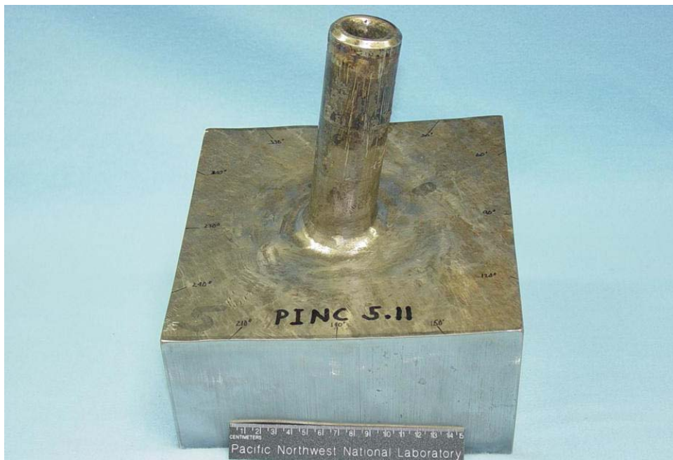
Figure 2.21 PINC 5.11 from PNNL – WNP-1 BMI Nozzle Penetration 5
