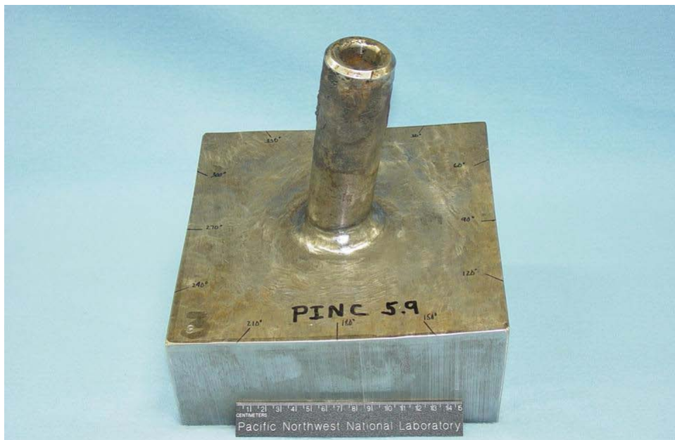
Figure 2.19 PINC 5.9 from PNNL – WNP-1 BMI Nozzle Penetration 3
