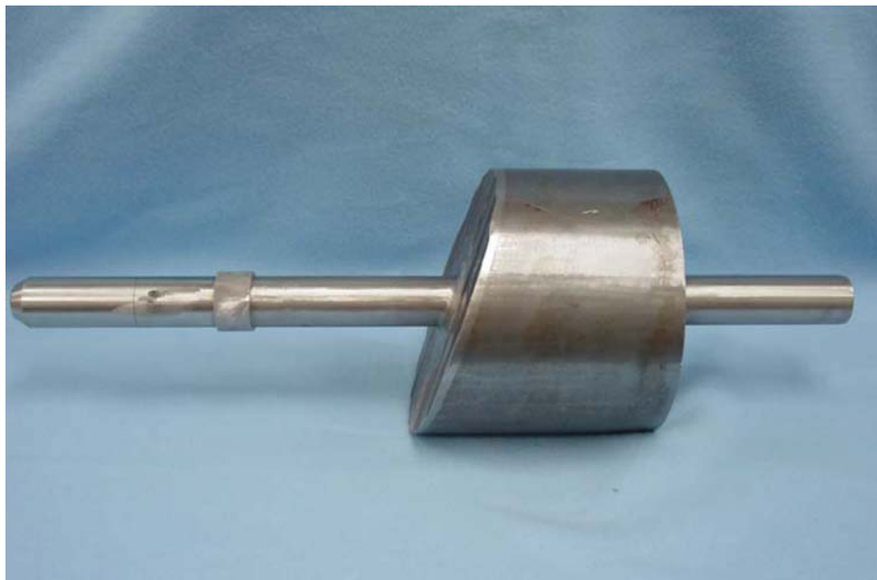
Figure 2.27 PINC 5.1 from KINS – BMI Nozzle Test Block
