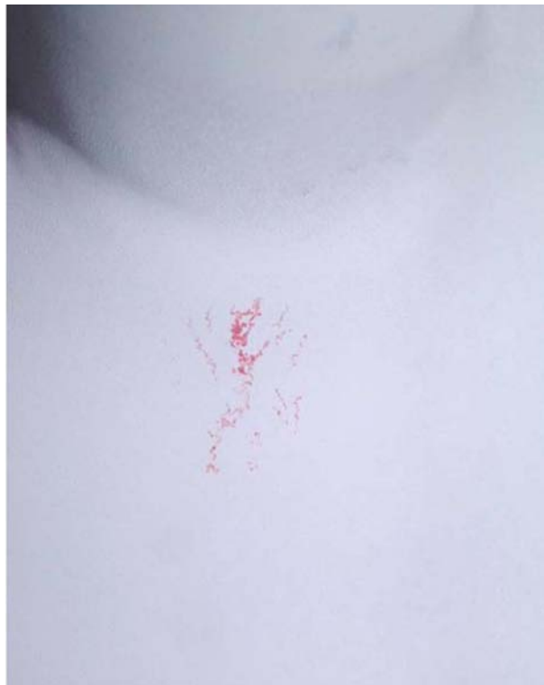
Figure 2.59 Example of Laboratory-Induced SCC in BMI Test Block (perpendicular to the weld)
