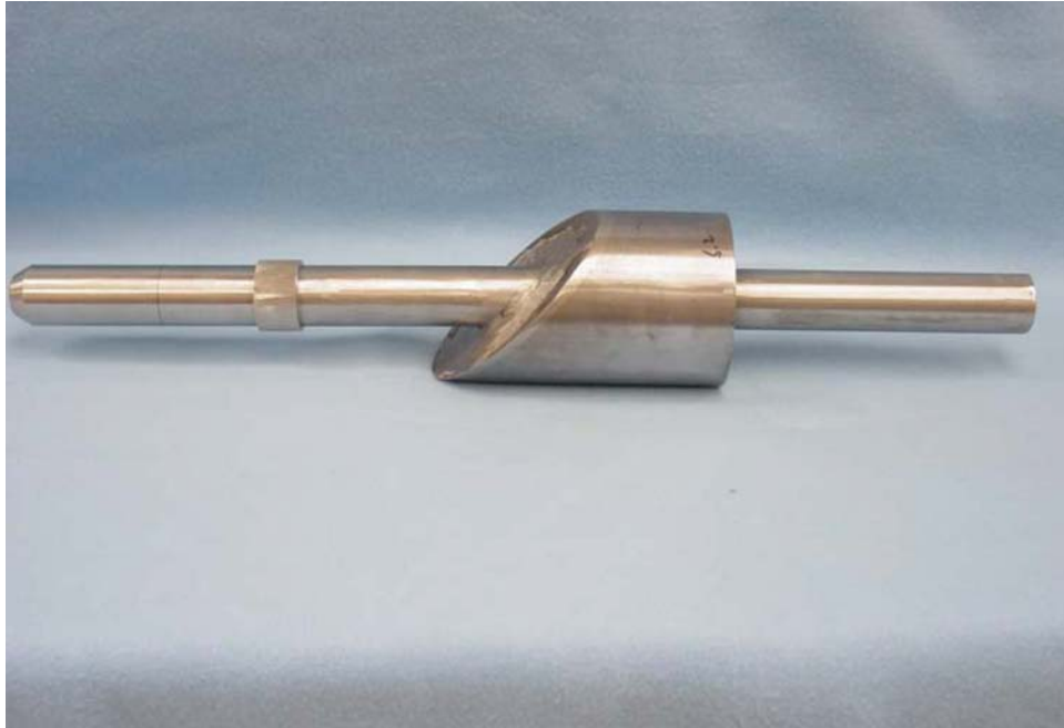
Figure 2.28 PINC 5.2 from KINS – BMI Nozzle Test Block
