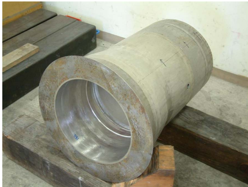
Figure 2.7 PINC Block 2.9 from Swedish Qualification Center (SQC)
