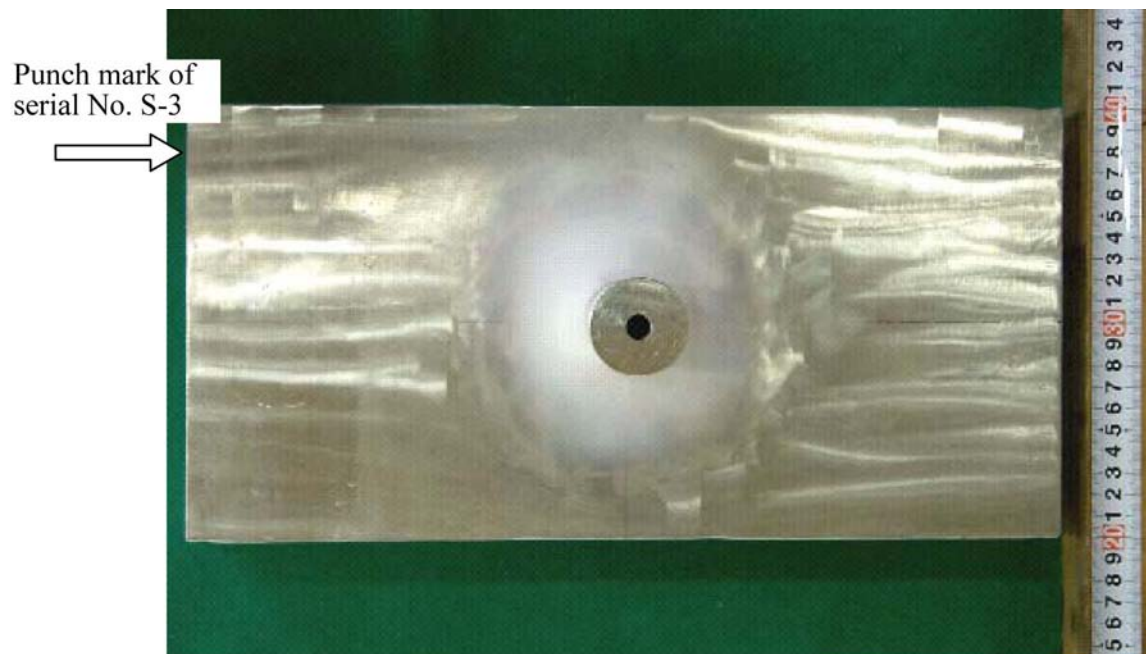
Figure 2.25 PINC 5.15 from JNES – BMI Nozzle Test Block No. 3
