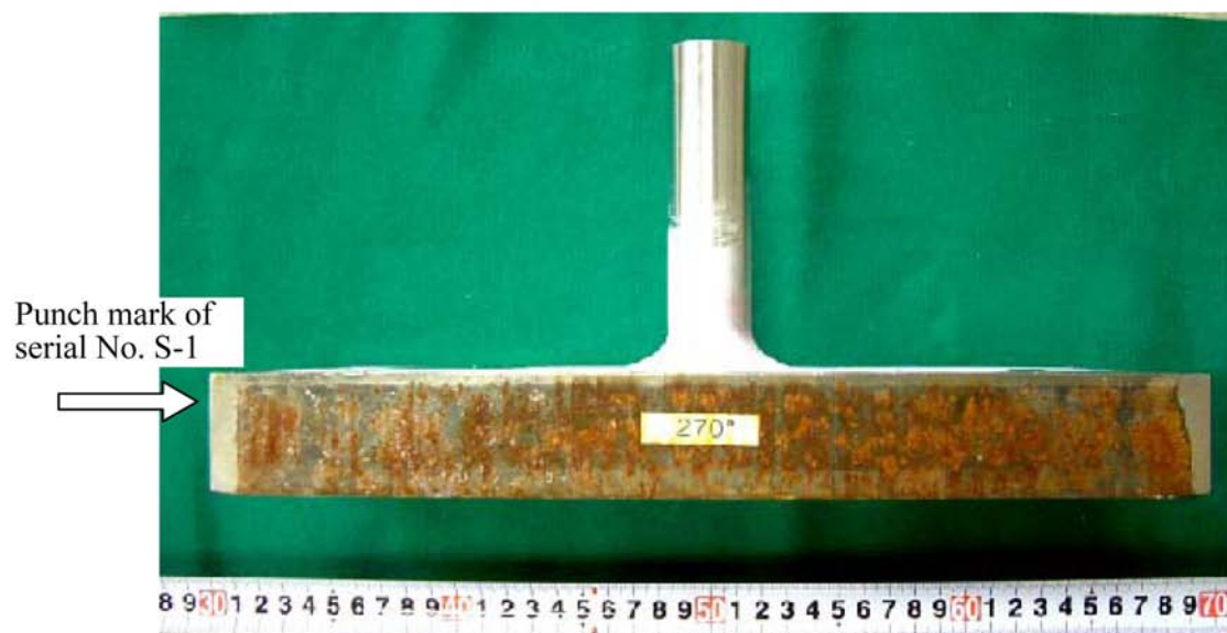
Figure 2.23 PINC 5.13 from JNES – BMI Nozzle Test Block No. 1
