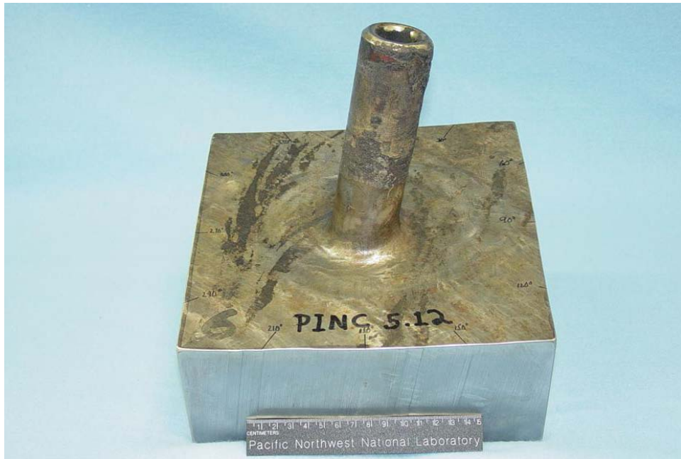
Figure 2.22 PINC 5.12 from PNNL – WNP-1 BMI Nozzle Penetration 6
