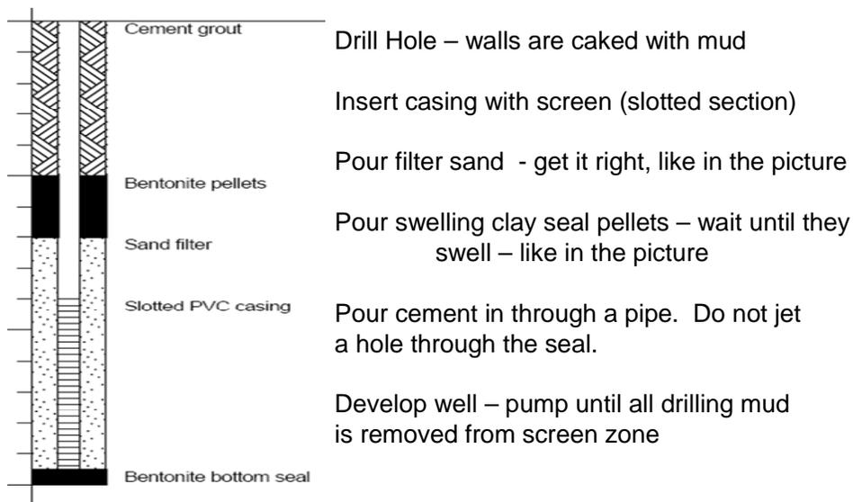
**Figure 8-20. Schematic of monitoring well with steps in installation.**
