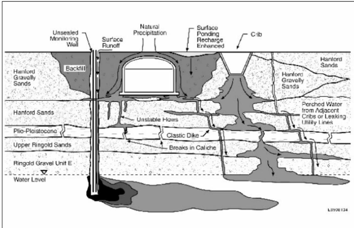
**Figure 7-9. Conceptual model of fluid flow beneath single shell tanks at Hanford Site showing fingering, funnel flow, and flow associated with clastic dikes or poorly sealed borehole annular space (Faybishenko, 2000)**
