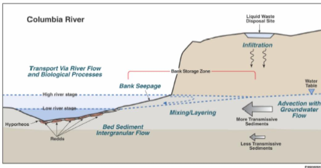
**Figure 7-16. Hydrogeologic conceptual model of contaminant movement below the Hanford 300 Area (DOE, 2002)**
