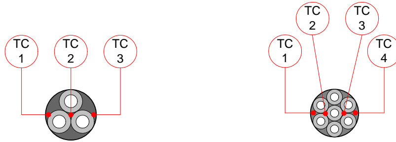
Figure 7: Example thermocouple arrangements for cross sectional temperature mapping of 3- and 7-conductor cables.
