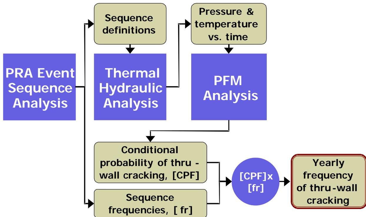
Figure 1. Integrated technical analyses comprising the PTS re-analysis project.
