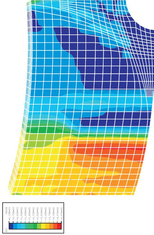
Figure 7-24. Concrete Hoop Strain Contours, Posttest Analysis Case C
