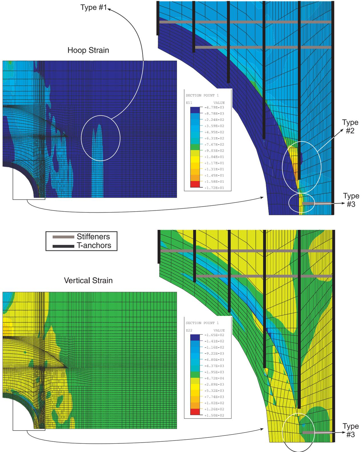
Figure 7-3. Liner Contour Strain Plots at P = 3.2 Pd for E/H from Pretest Analysis [1]
