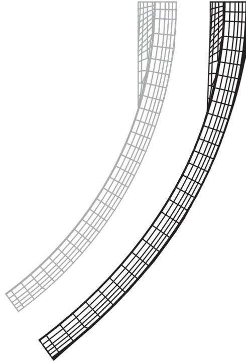
Figure 7-9. Deformed Shape of E/H Mode, Case A (Magnification Factor = 10)
