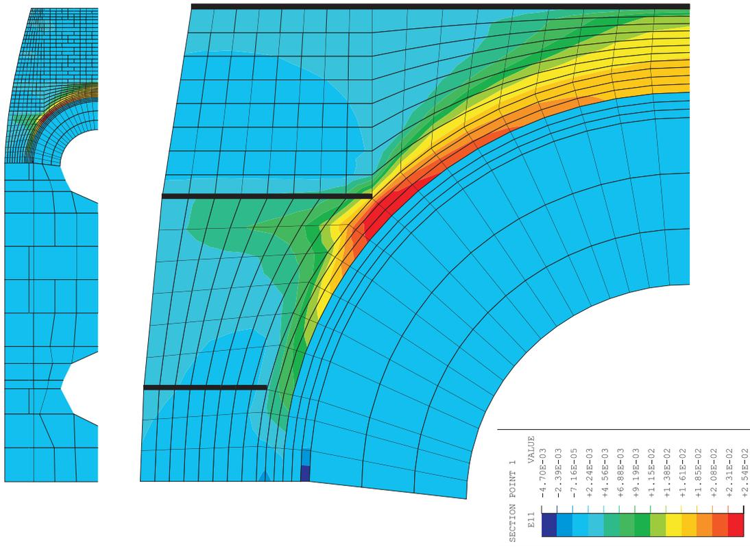
Figure 7-43. Hoop (Left) and Meridional (Right) Strains for Posttest M/S Analysis at P = 3.3 Pd
