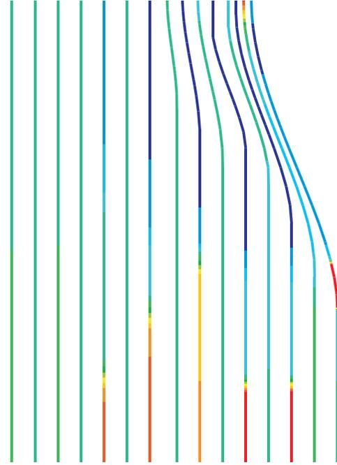
Figure 7-12. Hoop Tendon Stresses and Strains, Posttest Analysis Case A, at 3.5 Pd and 3.6 Pd (Stresses in psi; multiply by 0.00690 for MPa)
