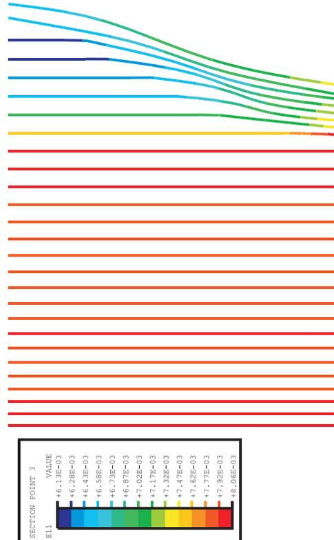
Figure 7-13. Vertical Tendon Stresses and Strains, Posttest Analysis Case A, at Prestress and 3.6 Pd (Stresses in psi; Multiply by 0.00690 for MPa)
