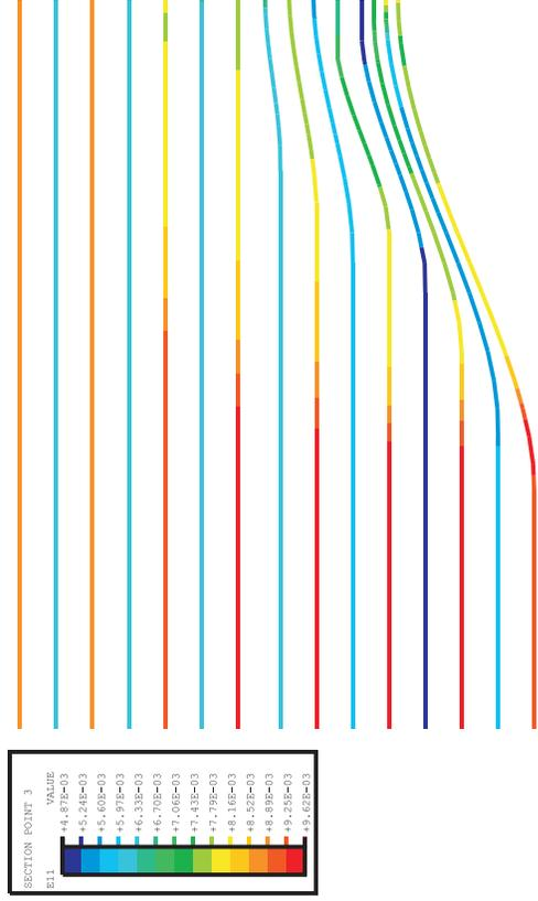
Figure 7-25. Hoop Tendon Stresses and Strains, Posttest Analysis Case C, at Prestress and 3.0 Pd (Stresses in psi; Multiply by 0.00690 for MPa)
