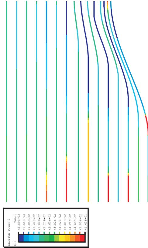
Figure 7-26. Hoop Tendon Stresses and Strains, Posttest Analysis Case C, at 3.5 Pd and 3.6 Pd (Stresses in psi; Multiply by 0.00690 for MPa)
