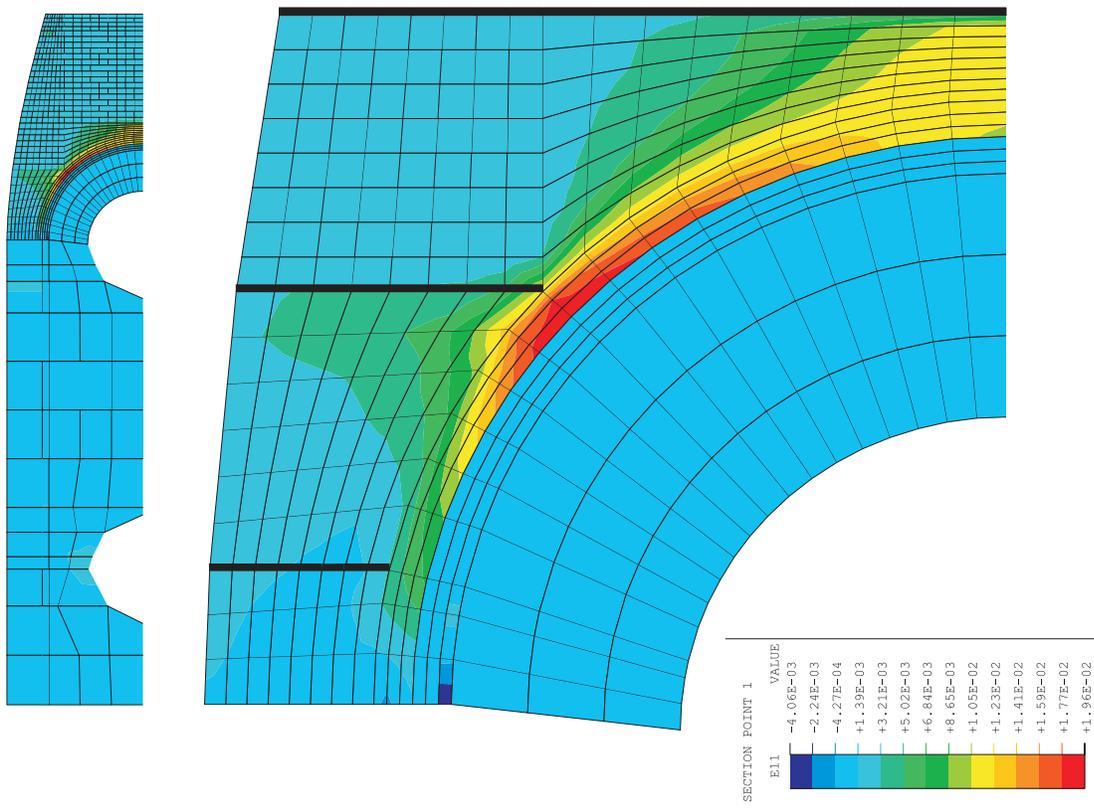
Figure 7-42. Hoop (Left) and Meridional (Right) Strains for Posttest M/S Analysis at P = 3.0 Pd
