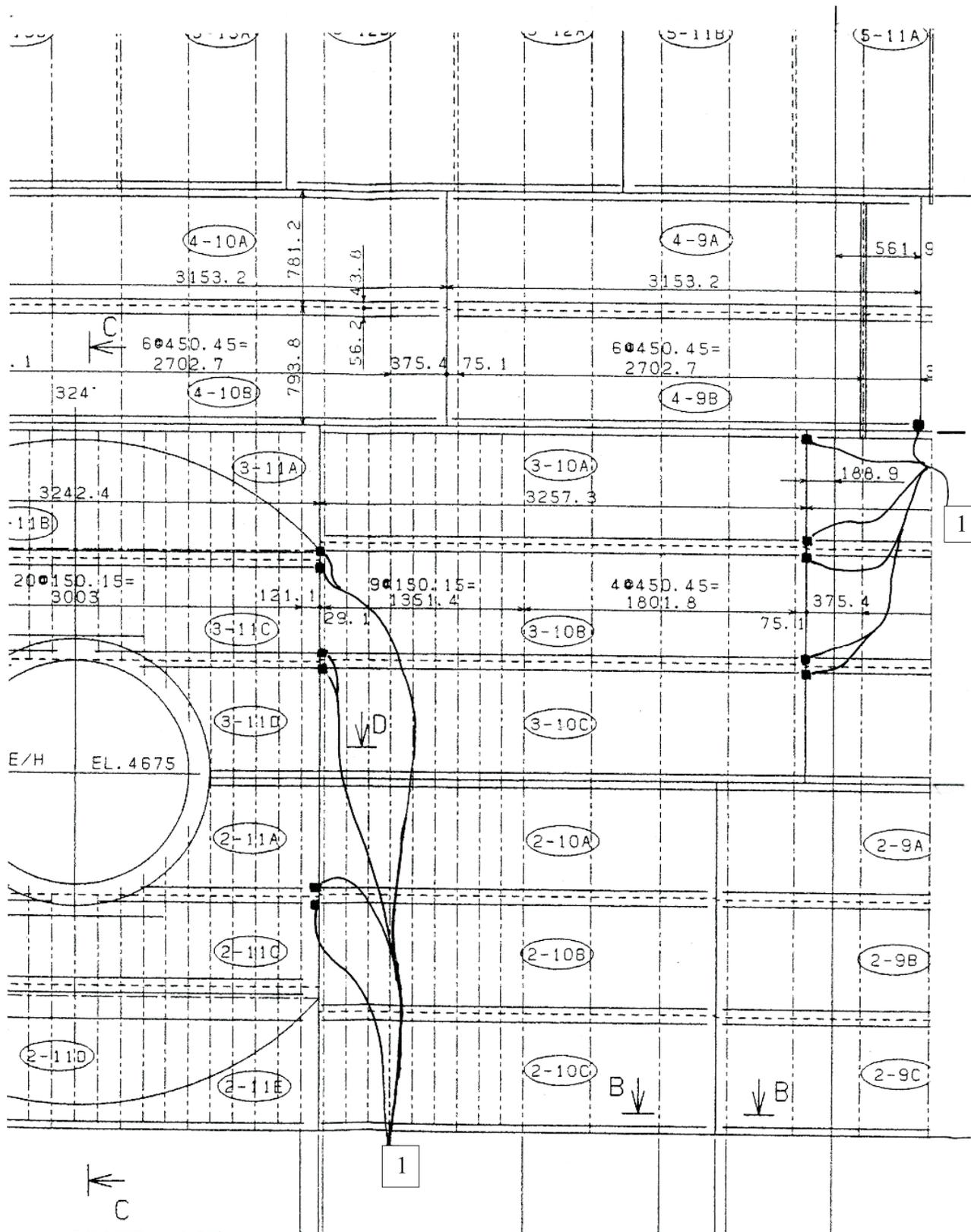
Figure 7-30. Strain Concentration Type 1 Near 270 Degrees Buttress and Near E/H
