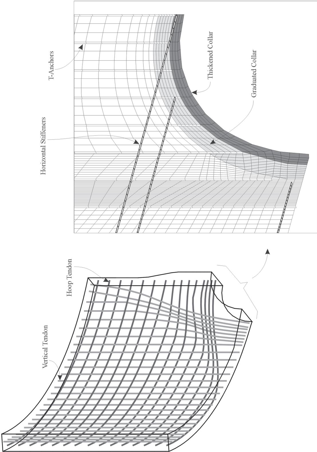
Figure 7-8. E/H Finite Element Model Including Tendons, Liner, Anchors, and Stiffeners
