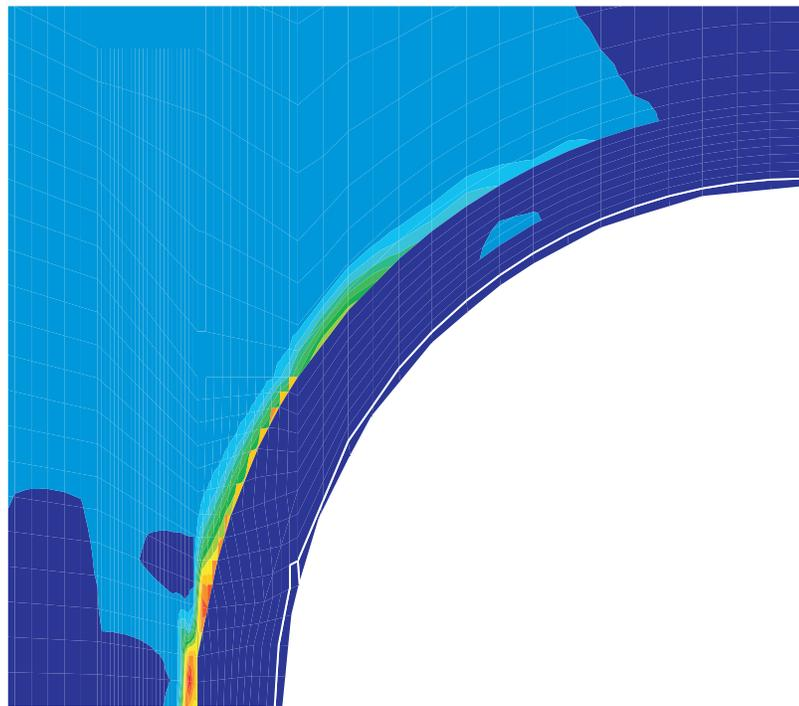
Figure 7-28. Liner Hoop Strains, Posttest Analysis Case C, at 3.2 Pd
