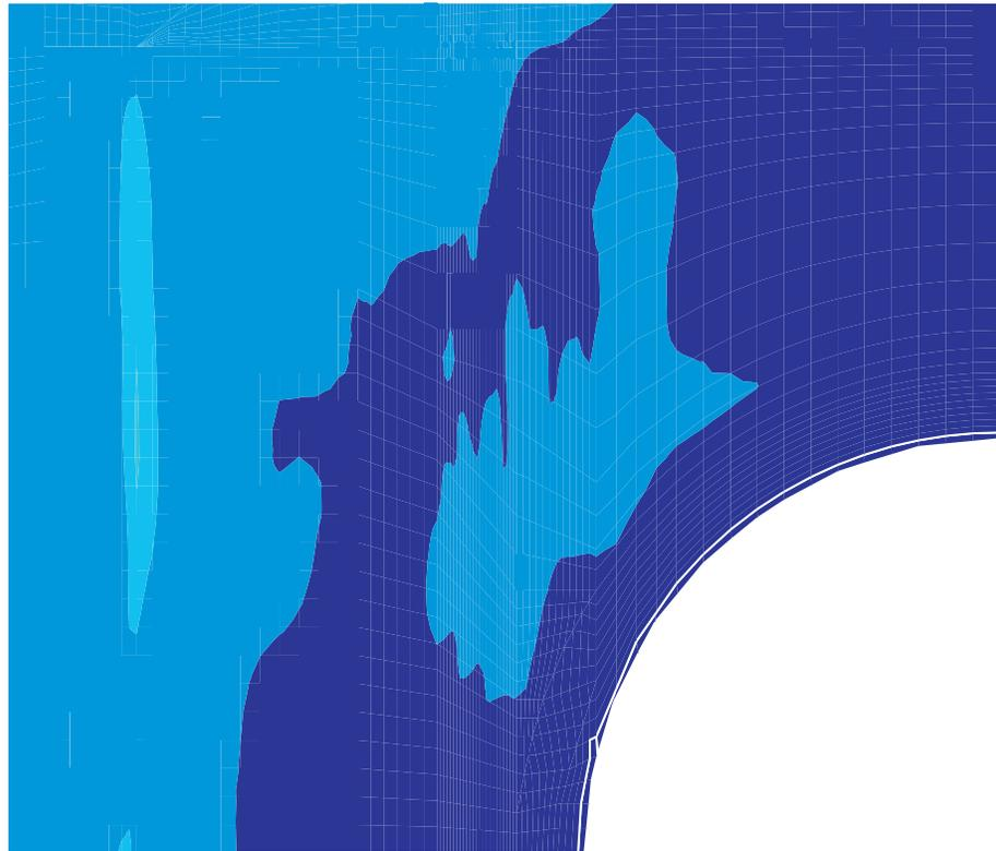
Figure 7-38. Liner Hoop Strains, Posttest Analysis Case E, at 3.2 Pd
