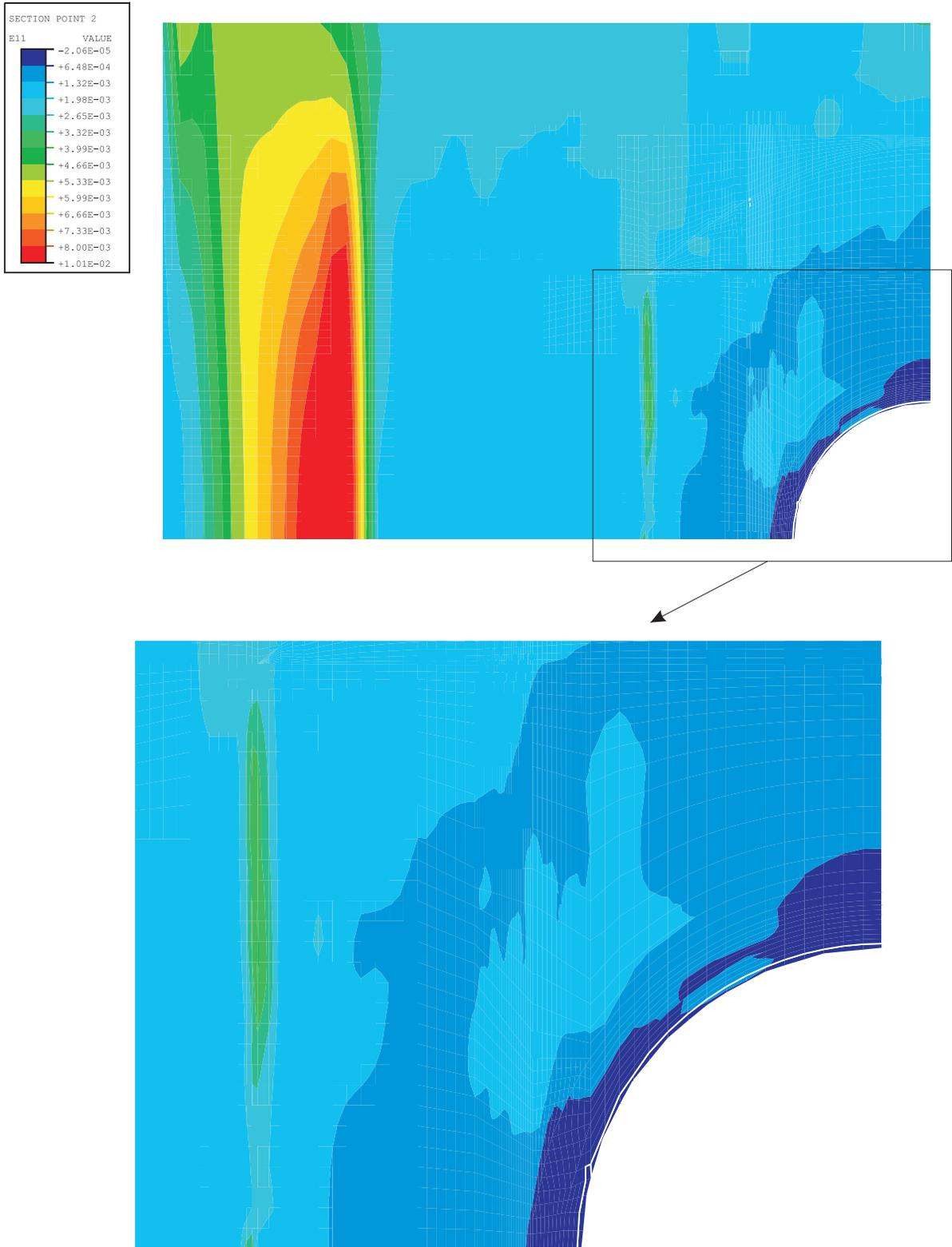
Figure 7-37. Liner Hoop Strains, Posttest Analysis Case E, at 3.0 Pd
