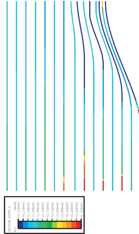
Figure 7-19. Hoop Tendon Stresses and Strains, Posttest Analysis Case B, at 3.5 Pd and 3.6 Pd (Stresses in psi; Multiply by 0.00690 for MPa)
