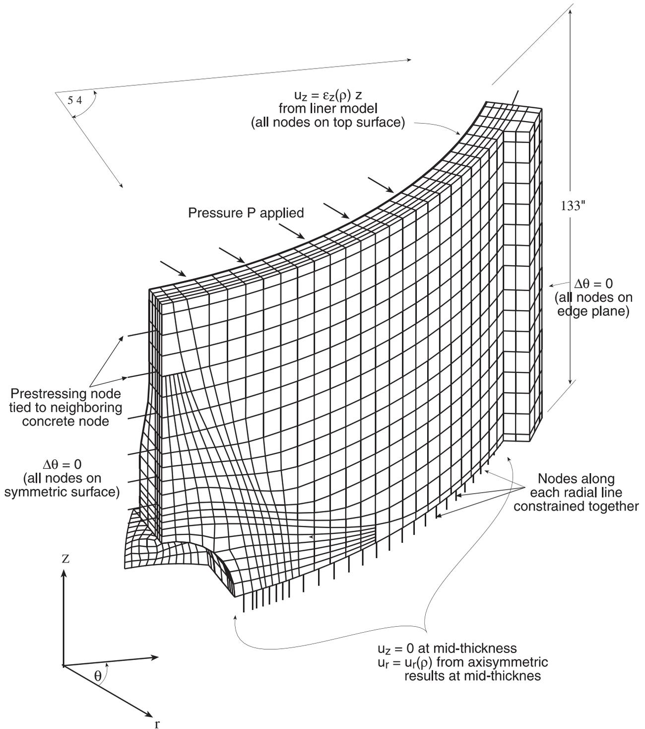
Figure 7-1. Boundary Conditions and Geometry for 3D E/H Model Used in Pretest Analysis [1]
