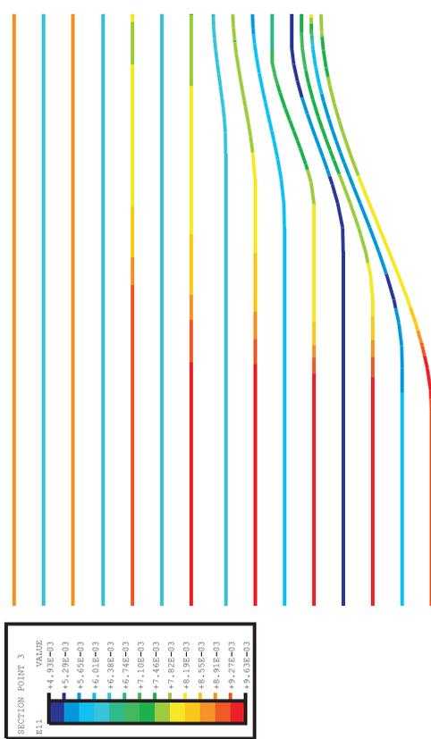
Figure 7-18. Hoop Tendon Stresses and Strains, Posttest Analysis Case B, at Prestress and 3.0 Pd (Stresses in psi; Multiply by 0.00690 for MPa)
