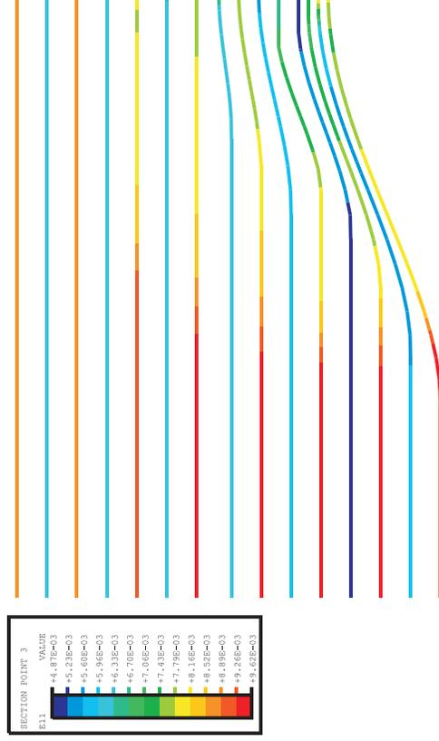
Figure 7-11. Hoop Tendon Stresses and Strains, Posttest Analysis Case A, at Prestress and at 3.0 Pd (Stresses in psi; multiply by 0.00690 for MPa)
