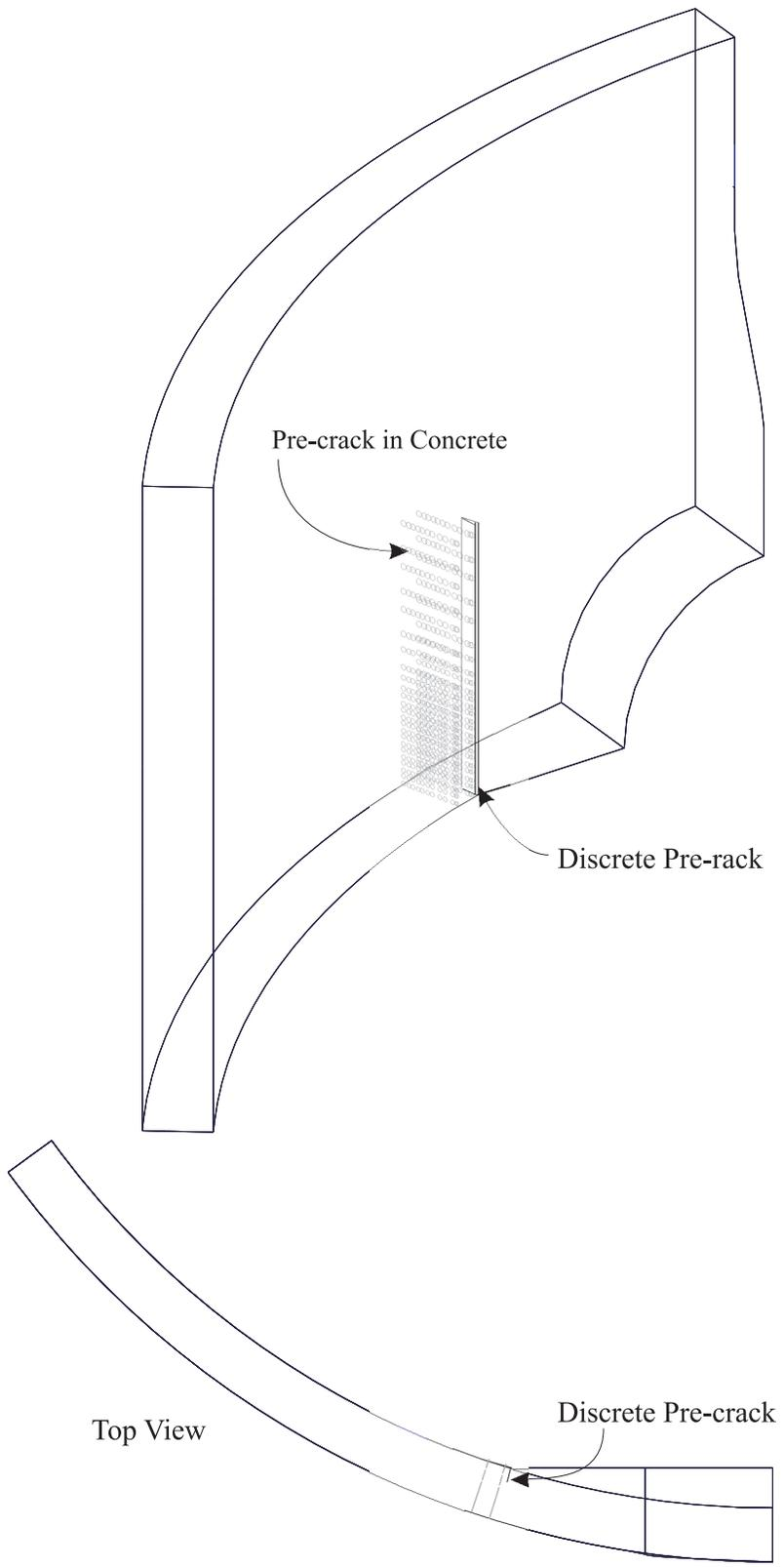
Figure 7-35. Illustration of Case E, Discrete Pre-Crack
