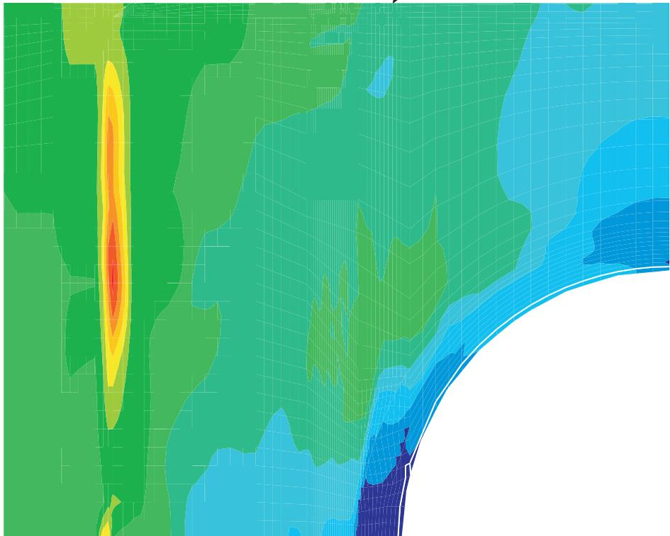
Figure 7-36. Liner Hoop Strains, Posttest Analysis Case E, at 2.8 Pd
