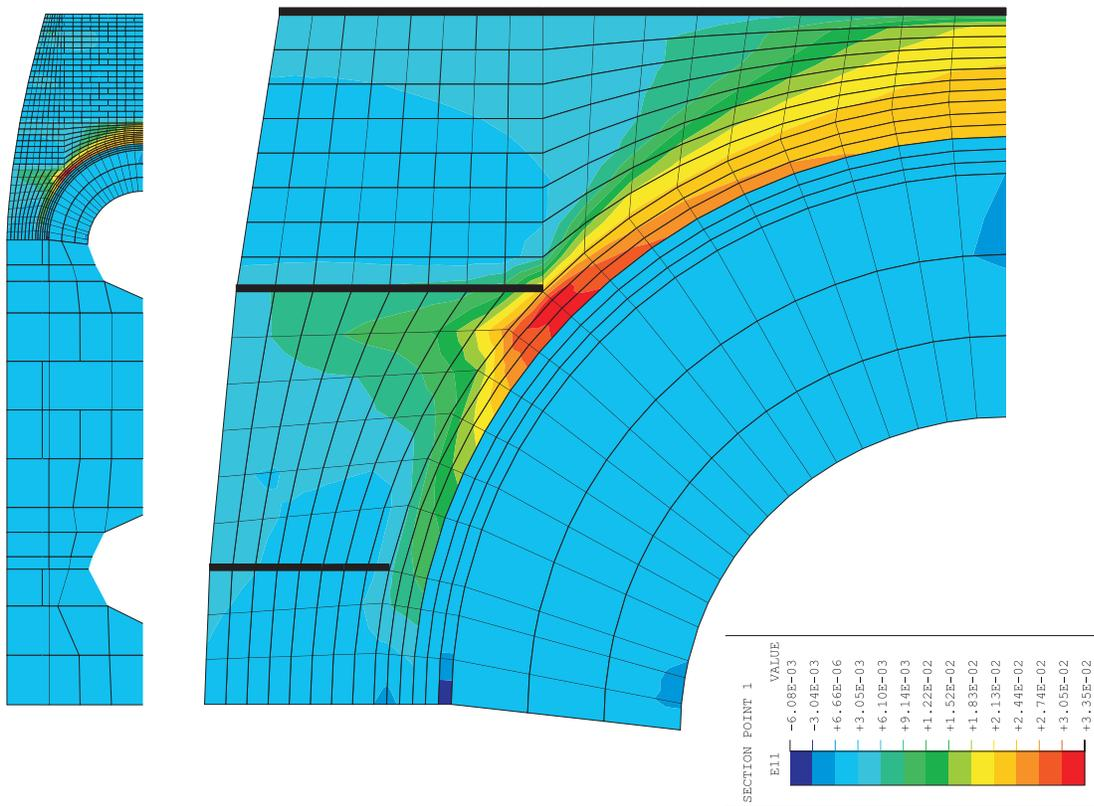
Figure 7-44. Hoop (Left) and Meridional (Right) Strains for Posttest M/S Analysis at P = 3.5 Pd
