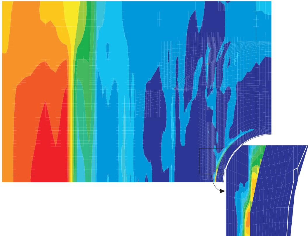
Figure 7-29. Liner Hoop Strains, Posttest Analysis Case C, at 3.5 Pd and 3.6 Pd
