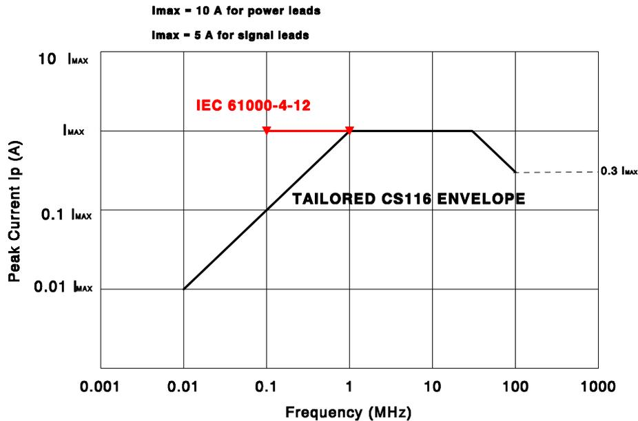
**Fig. 6.14. Damped sinusoid conducted susceptibility operating envelopes.**
