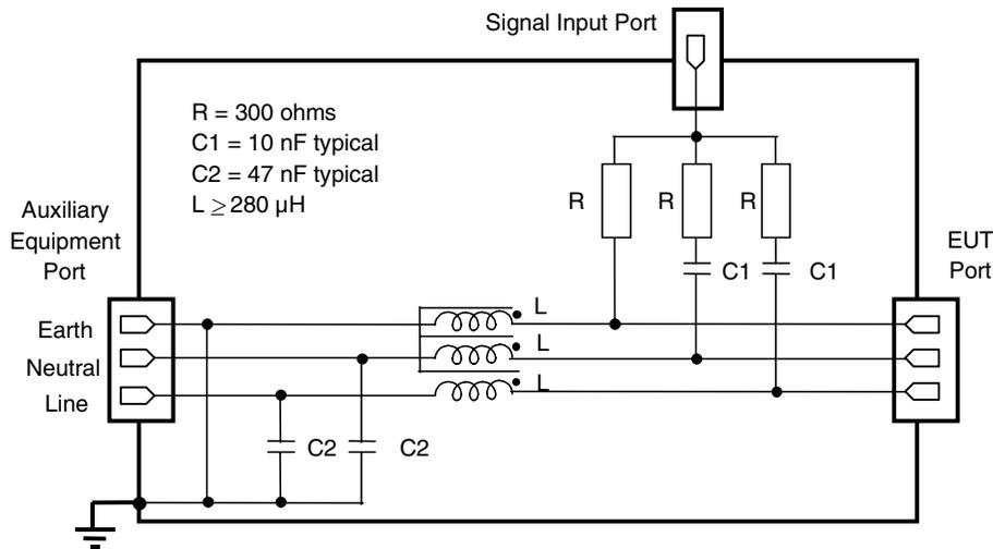
**Fig. 6.4. IEC 61000-4-6 coupling and decoupling network.**
