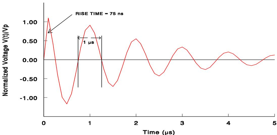
Fig. 6.13. Waveform of the damped oscillatory wave.
