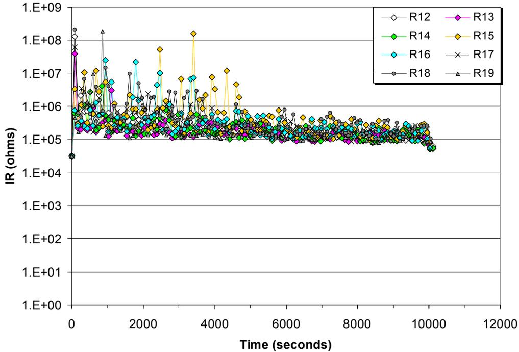
Figure 5-53. Representative conductor-to-conductor IRs obtained during Test 14.
