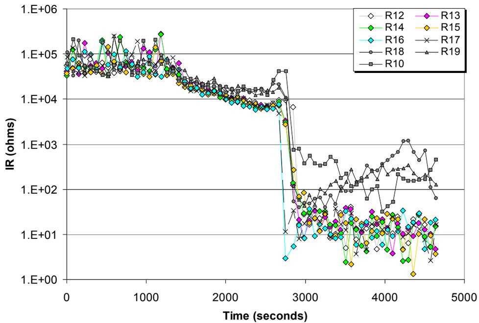
Figure 5-10. Representative conductor-to-conductor IRs obtained during Test 3.
