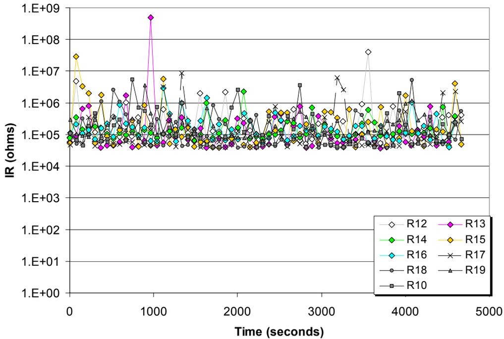
Figure 5-18. Representative conductor-to-conductor IRs obtained during Test 5.
