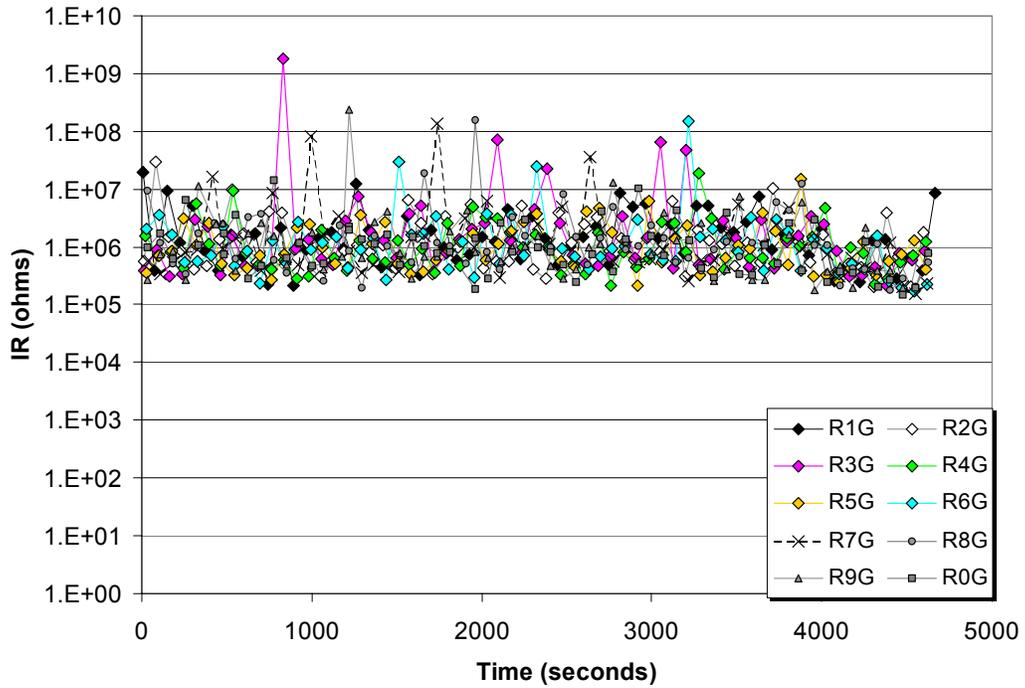
Figure 5-19. Conductor-to-ground IRs obtained during Test 5.
