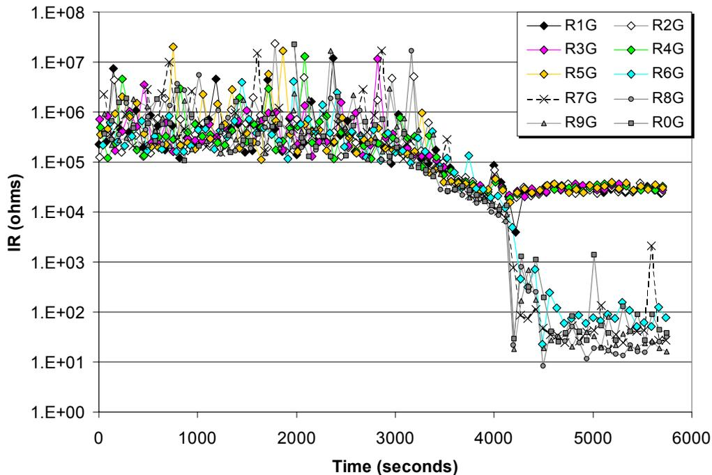
**Figure 5-33. Conductor-to-ground IRs obtained during Test 8.**
