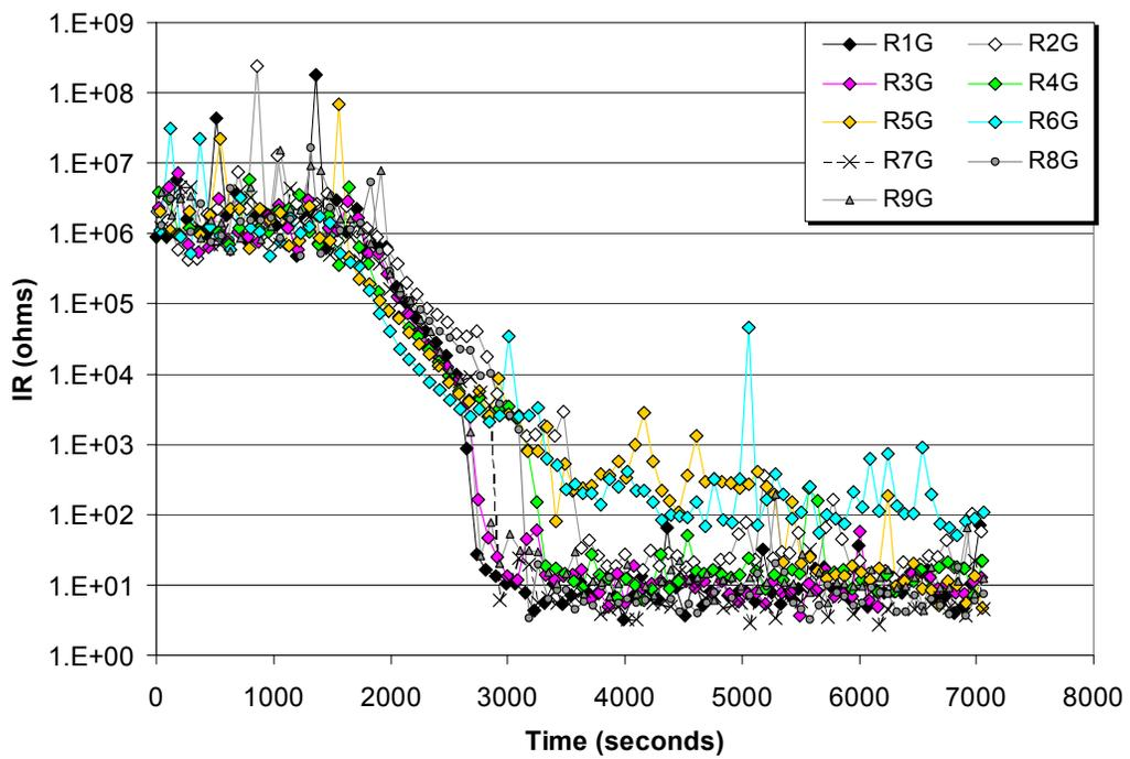
Figure 5-66. Conductor-to-ground IRs obtained during Test 18.
