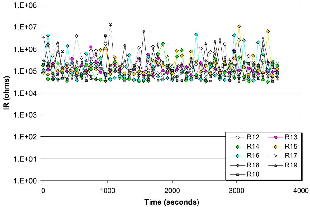
Figure 5-6. Representative conductor-to-conductor IRs obtained during Test 2.
