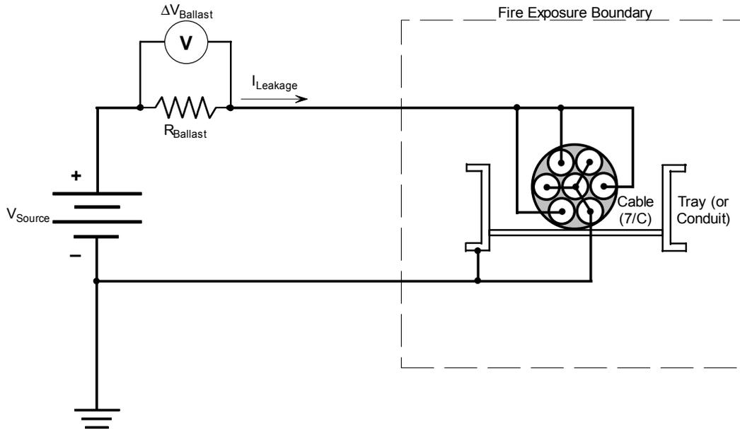
**Figure 2-3.** A single voltage source system applied to a multiconductor cable without a switching system. Note that the individual conductors are ganged into two groups, one energized and the second grounded. IR is determined for the energized conductors only, and then only as a group.
