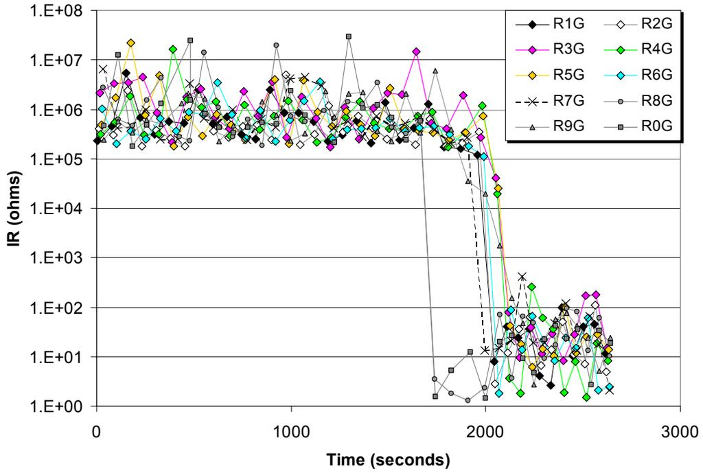
Figure 5-23. Conductor-to-ground IRs obtained during Test 6.
