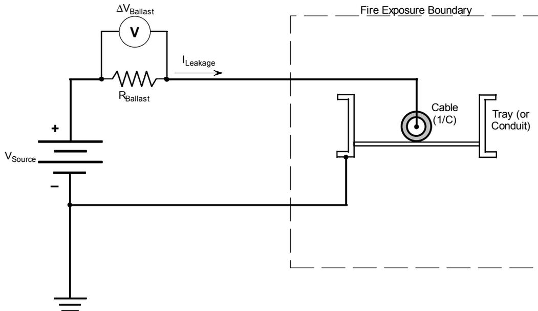
**Figure 2-1.** A simple cable functionality monitoring circuit using a single voltage potential applied to a single conductor cable. The circuit is capable of estimating the cable IR based on the measured voltage drop across the ballast resistor.
