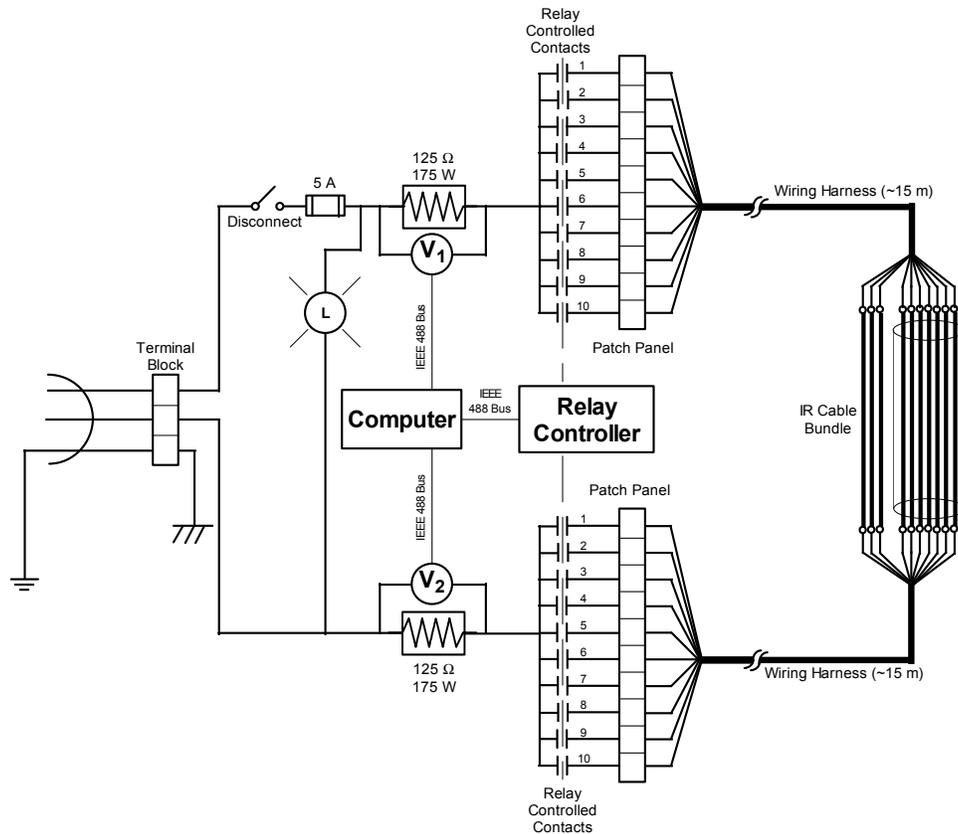
Figure 3-7. Schematic diagram of the IR measurement system.
