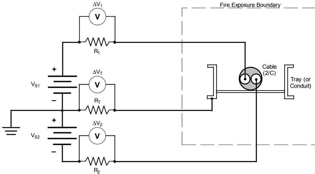
**Figure 2-4.** An example of a cable monitoring circuit using two energizing voltage potentials. Note the isolation of the raceway from ground by a ballast resistor and monitoring of the leakage current to ground.
