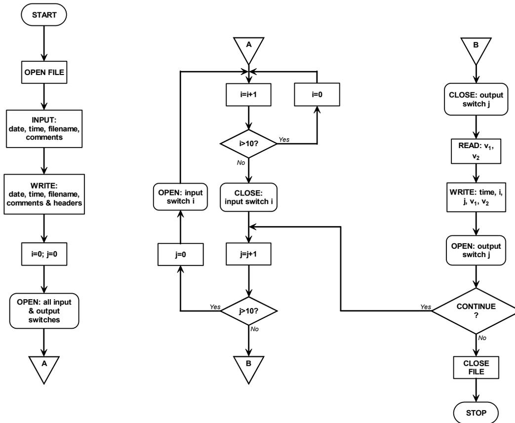
Figure 3-12. IR measurement system control program flow chart.
