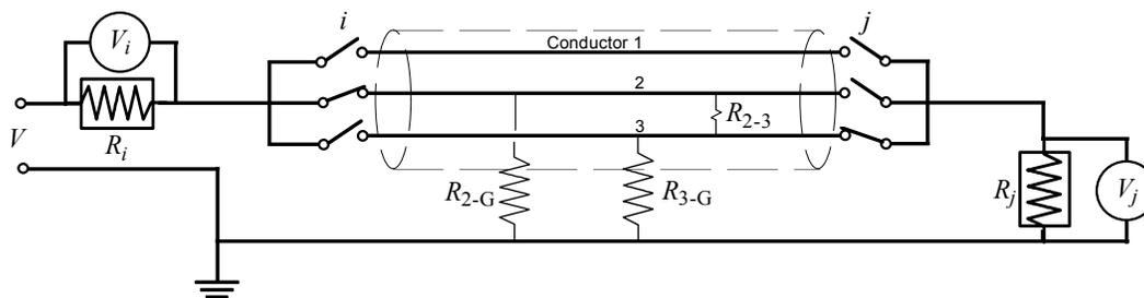
Figure 3-4. IR measuring circuit with ground paths.
