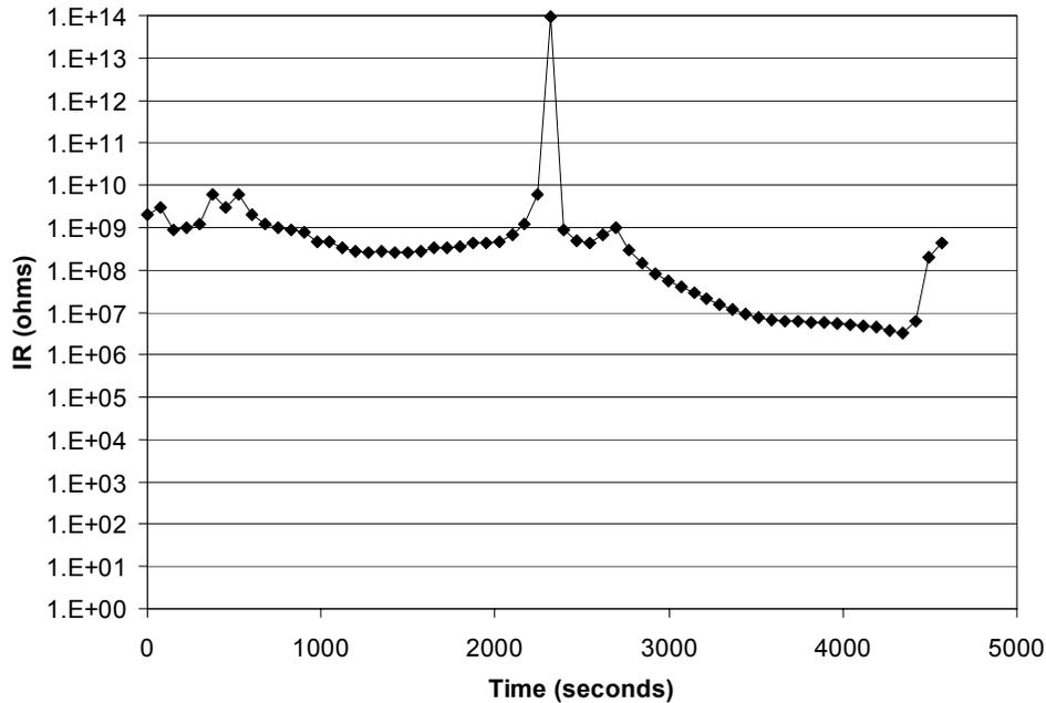
Figure 5-43. IR between Conductor 1 and 2 obtained during Test 11.
