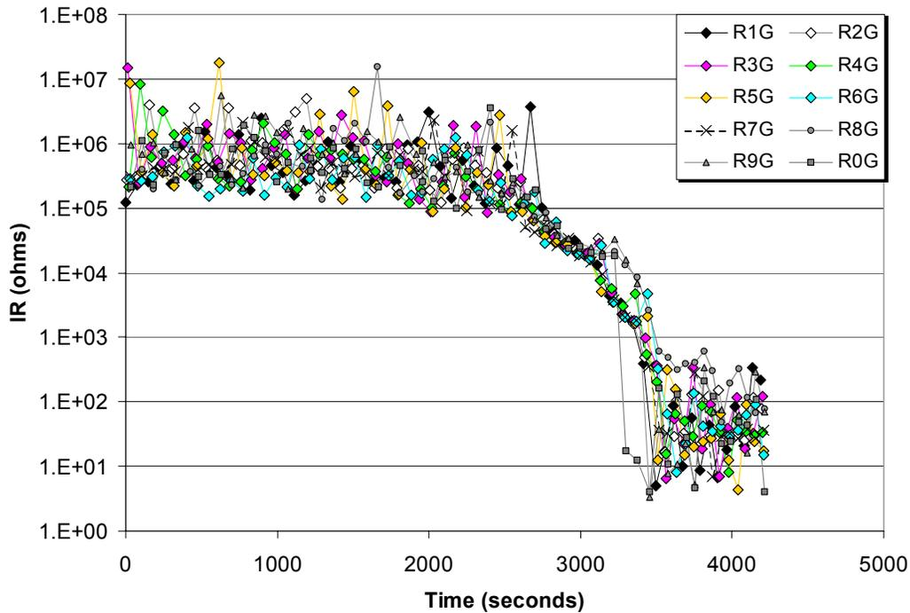
Figure 5-27. Conductor-to-ground IRs obtained during Test 7.
