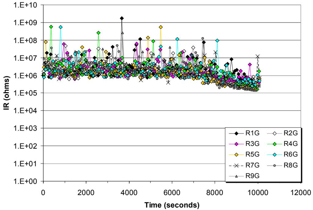
Figure 5-54. Conductor-to-ground IRs obtained during Test 14.
