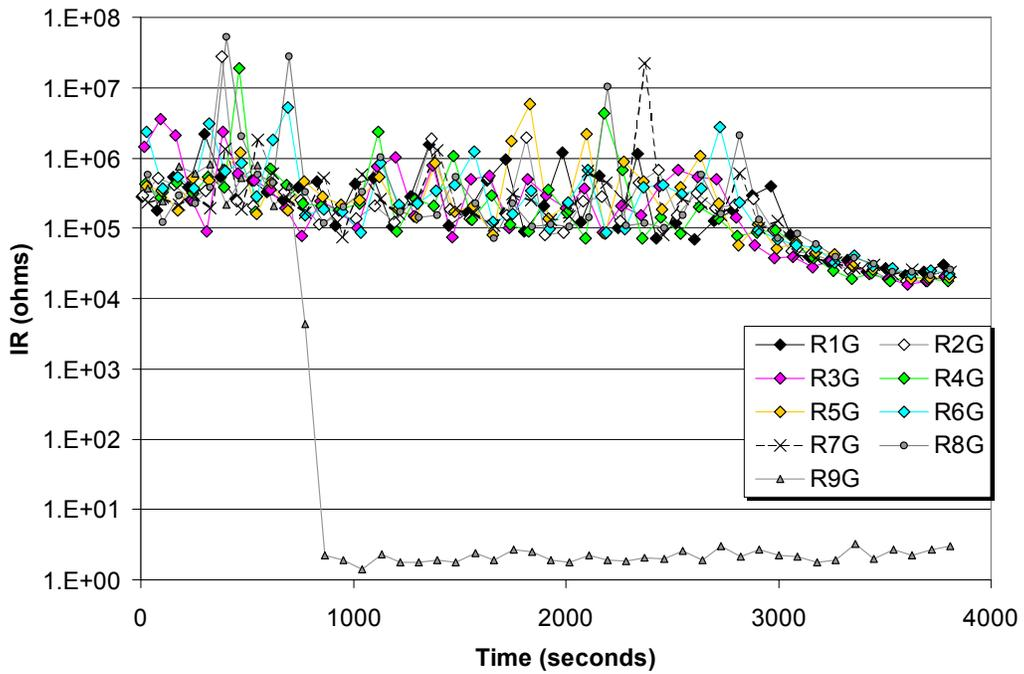
Figure 5-3. Conductor-to-ground IRs obtained during Test 1.
