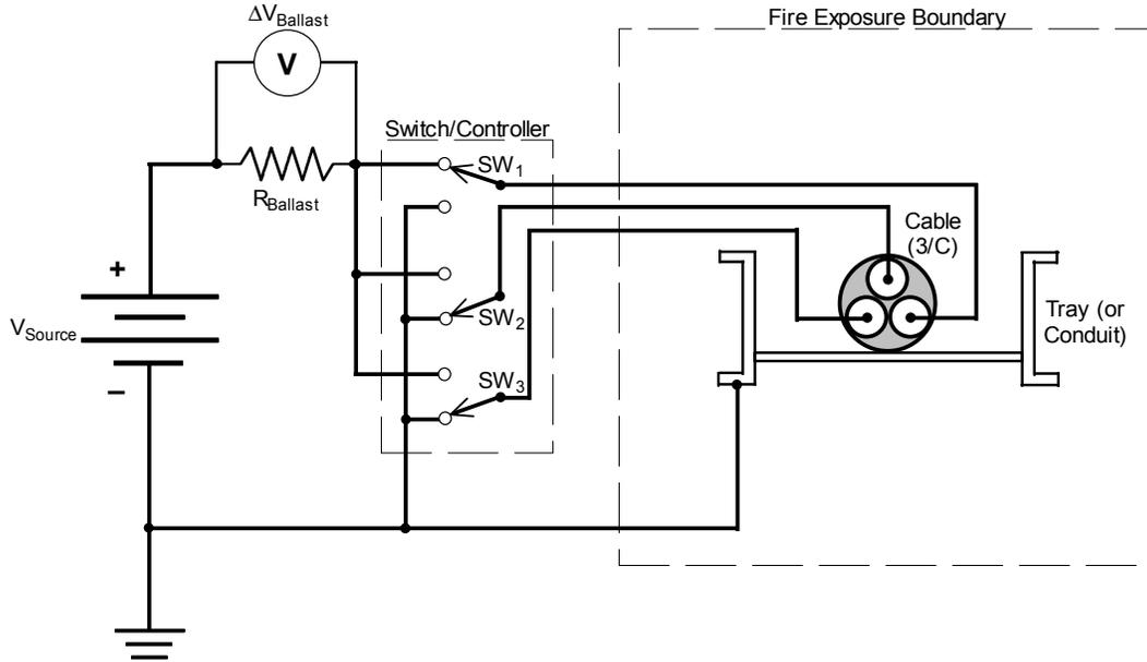
**Figure 2-2.** Electrical schematic of a single voltage potential monitoring system applied to a multiconductor cable. Note the switching controller is designed to select one conductor at a time to be energized while all others are grounded. A full measurement cycle sequentially energizes each conductor and measures leakage current. This approach can theoretically handle any number of individual conductors.
