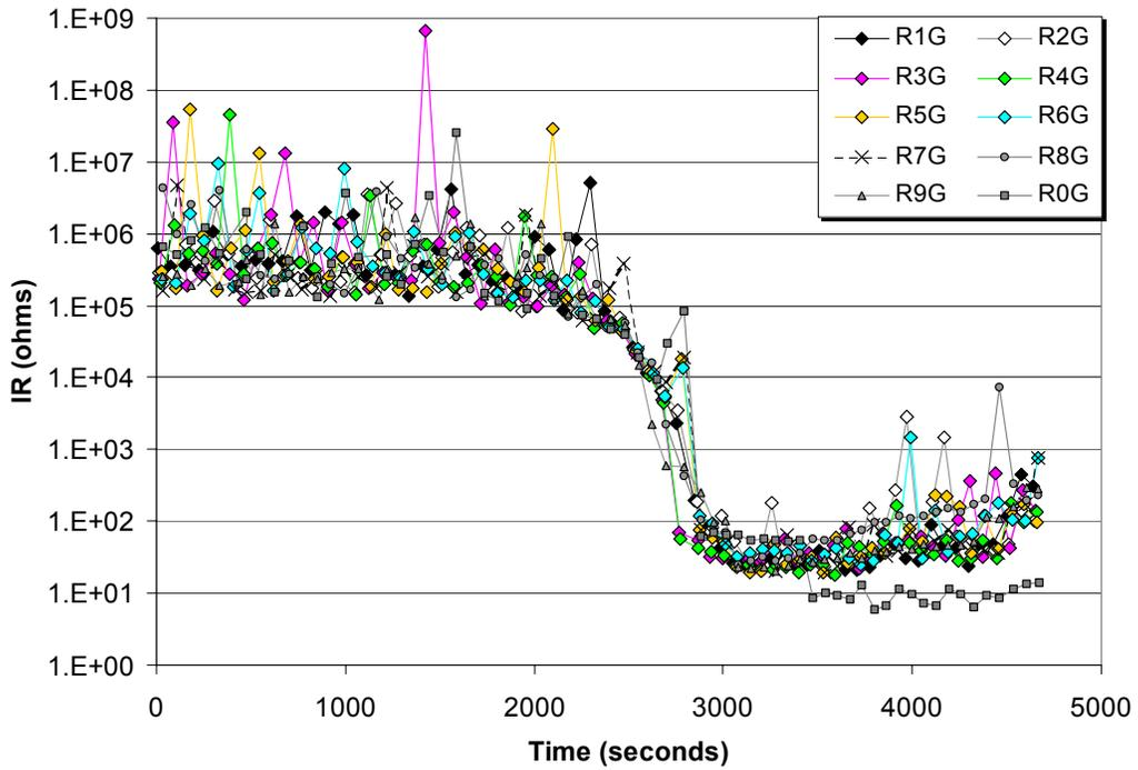
Figure 5-11. Conductor-to-ground IRs obtained during Test 3.
