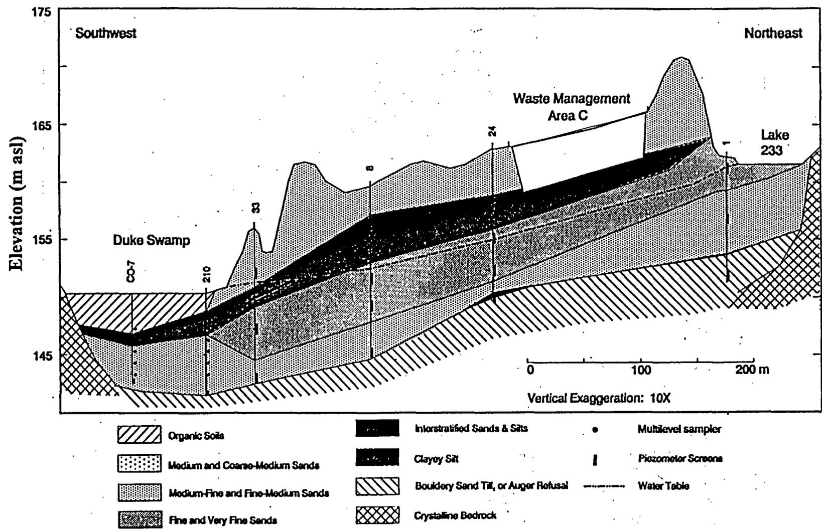
**Figure 1.10** Surface hydrology, water table contours, and areal extent of groundwater contamination by  $^3\text{H}$  (bifurcating, medium-gray pattern) in the vicinity of Area C. Dots indicate piezometer nest locations (refer to Figure 1.8 for nest identifiers).
