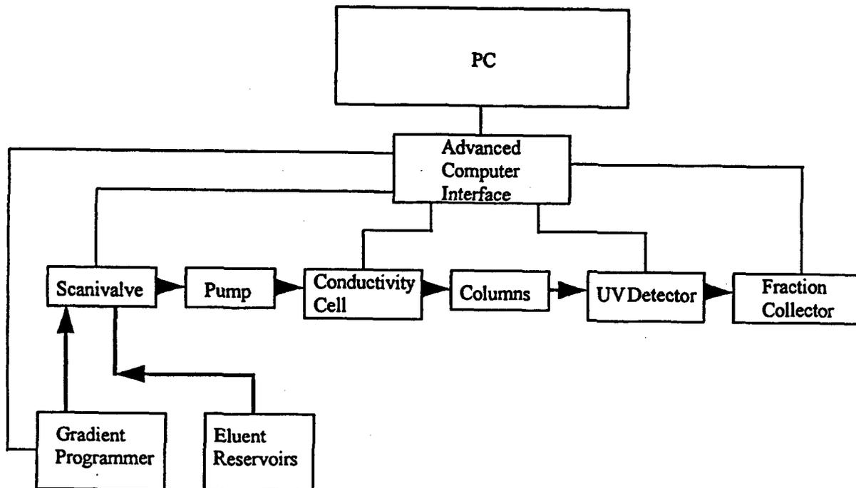
The Advanced Computer Interface was connected to a PC and controlled with Dionex software (AI-450). Fractions of effluent (6 mL) were collected with an LKB model 2070 ULTRORAC II programmable fraction collector, which was programmed to collect fractions for 2 minutes.
