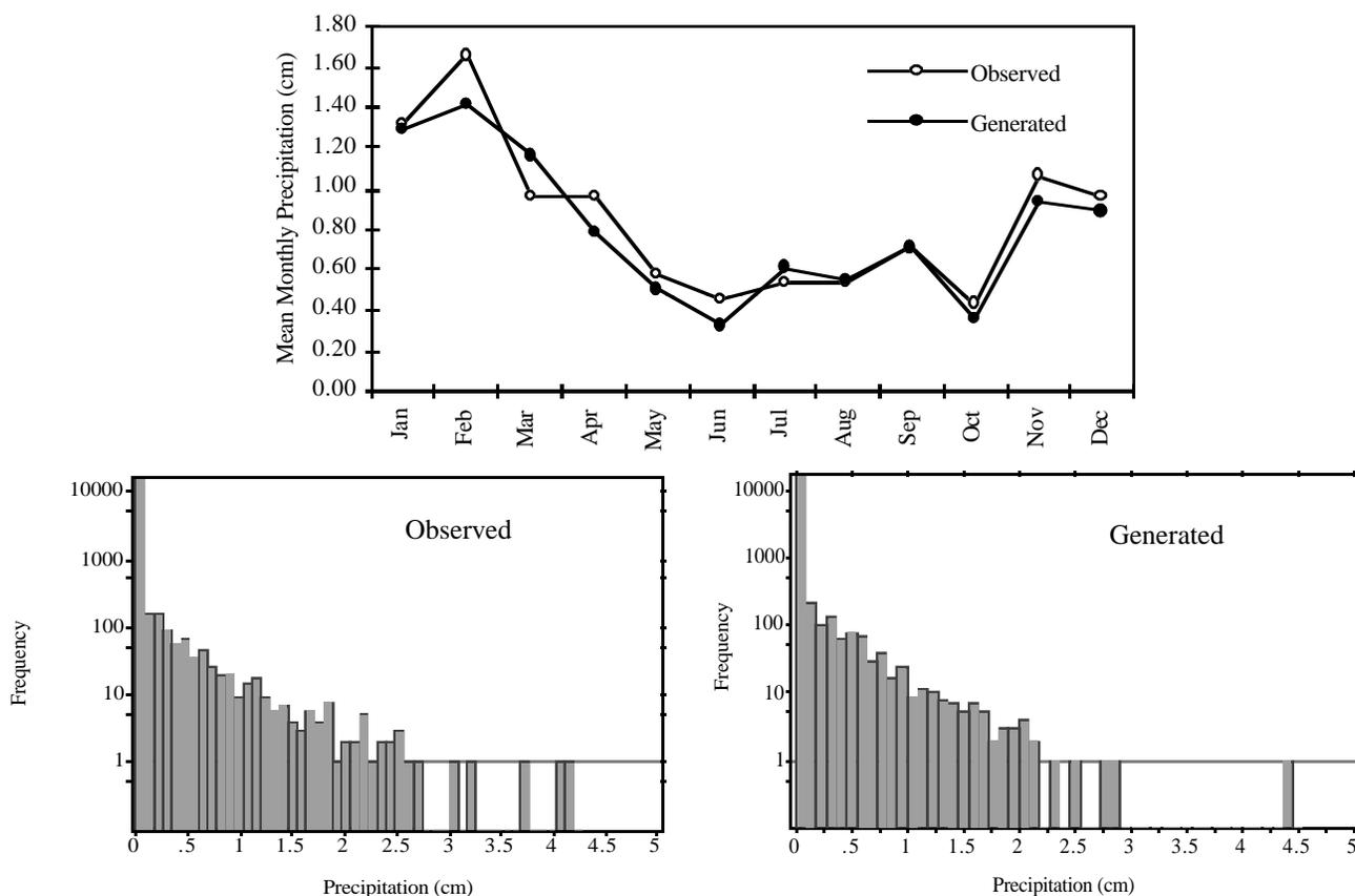
**Figure 6.12 Monthly average precipitation (top) and histograms of daily precipitation for the arid site example (Observed: 45-year adjusted record; Generated: the first 45 years of WGEN simulated precipitation)**
