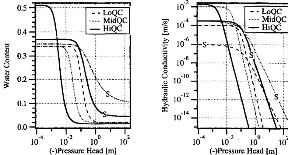
**Figure 6.8** Water retention and hydraulic conductivity curves for Hi-, Mid-, and LoQC sand and gravel materials. Curves labeled with an “S” are sand, and the others are gravel (MidQC and LoQC water retention curves for sand coincide).
