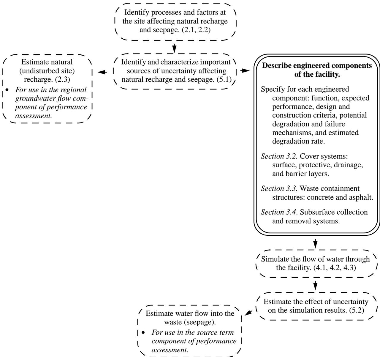
**Figure 3.1** Flowchart for the Hydrologic Evaluation Methodology. Chapter 3 discusses the engineered components of the facility. Numbers indicate sections in this document in which the items are discussed.
