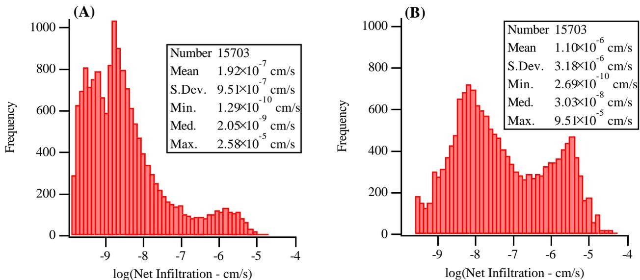
**Figure 5.4 Histograms of simulated daily net infiltration for a 43 year period based on (A) hourly averaged precipitation and (B) daily averaged precipitation**
