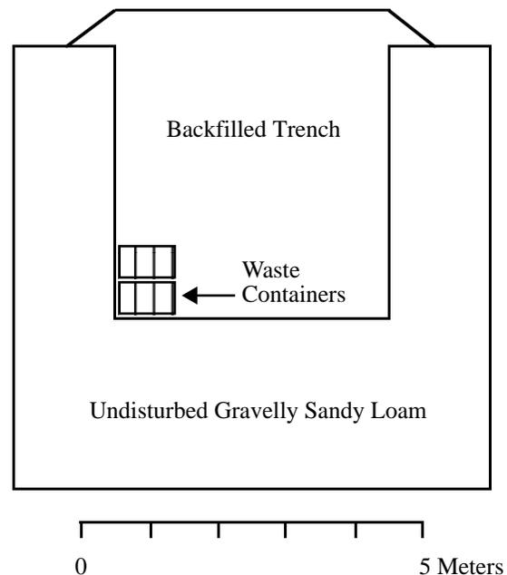
**Figure 6.10** Cross-section of hypothetical arid-site LLW disposal facility
