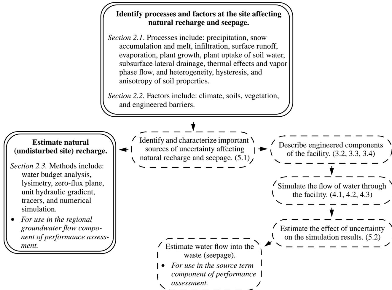
**Figure 2.1** Flowchart for the Hydrologic Evaluation Methodology. Chapter 2 discusses the processes and factors affecting recharge and seepage as well as methods for estimating recharge. Numbers indicate sections in this document in which the items are discussed.
