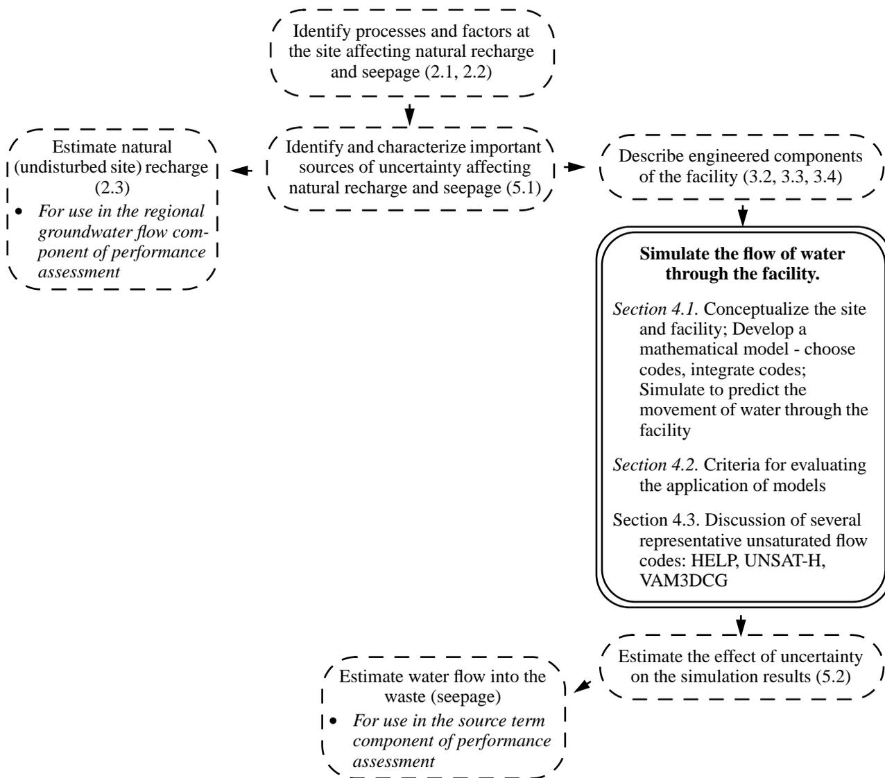
**Figure 4.1** Flowchart for the Hydrologic Evaluation Methodology. Chapter 4 discusses the simulation of water flow through the facility and the evaluation of model application. Numbers indicate sections in this document in which the items are discussed.
