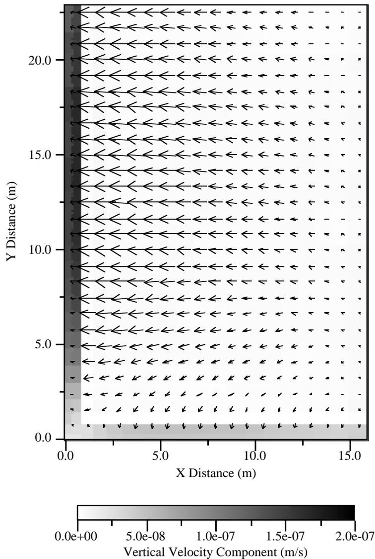
**Figure 6.9** Velocity vector plot for three-dimensional model, 1:5 slope, HiQC materials in XY plane 15 (the plane immediately above the capillary barrier). The vectors depict the velocity components in the X and Y directions (parallel to the capillary barrier), while the grayscale raster image depicts the magnitude of the element vertical (Z-direction) velocity components.
