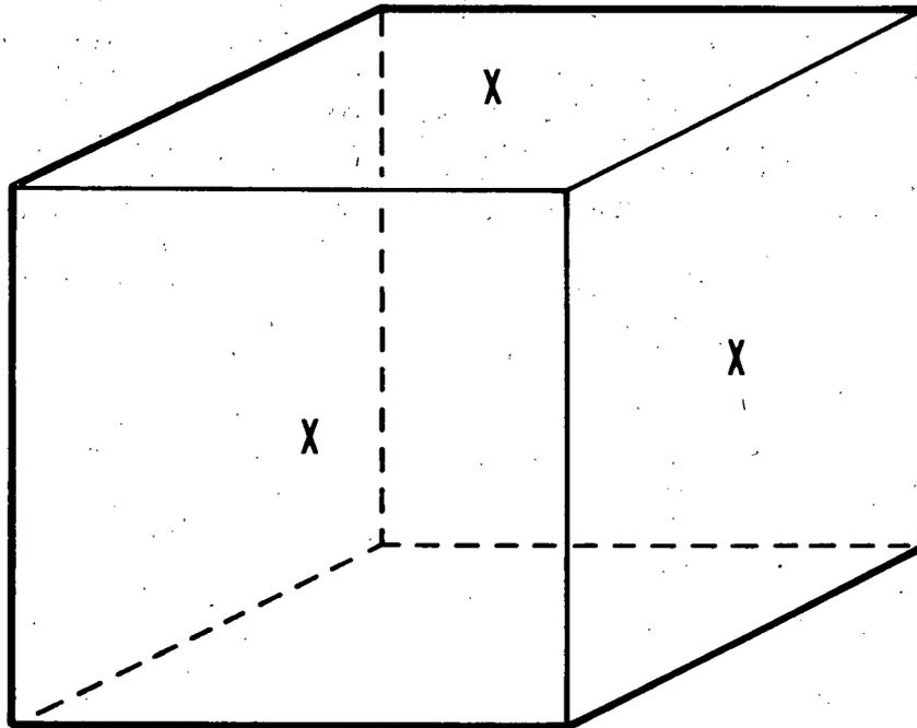
Figure 7. Location of Thermocouples on Solid and Hollow Cube Calorimeters
