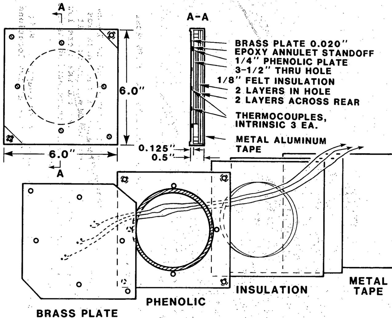
Figure 5. Assembly Drawing of Flat-Plate Calorimeter
