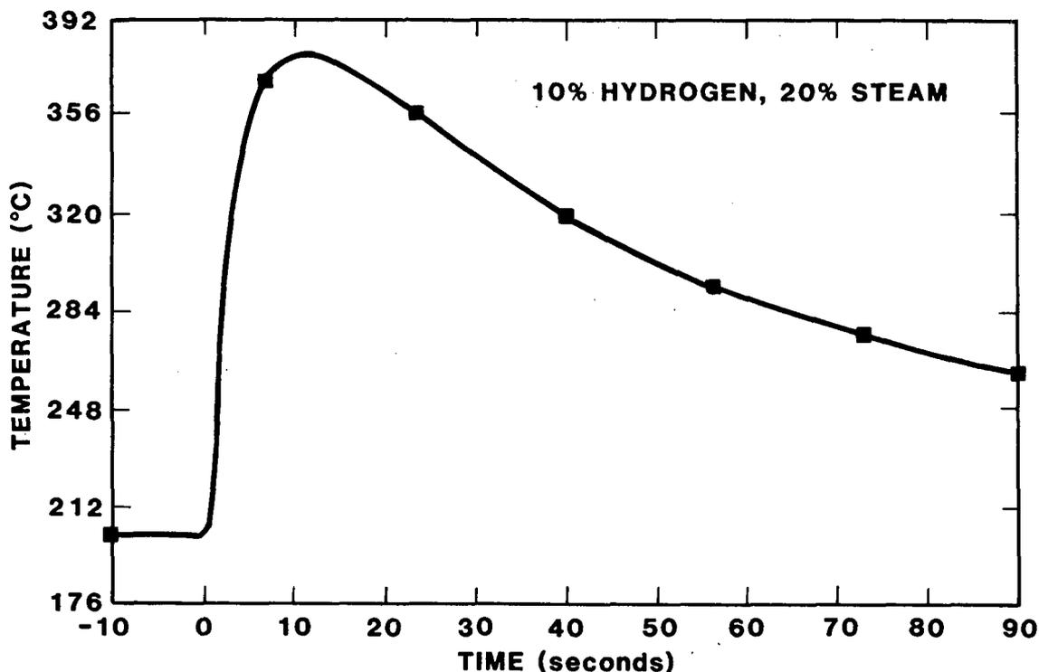
Figure 15. Typical Temperature Response for Flat-Plate Calorimeter
