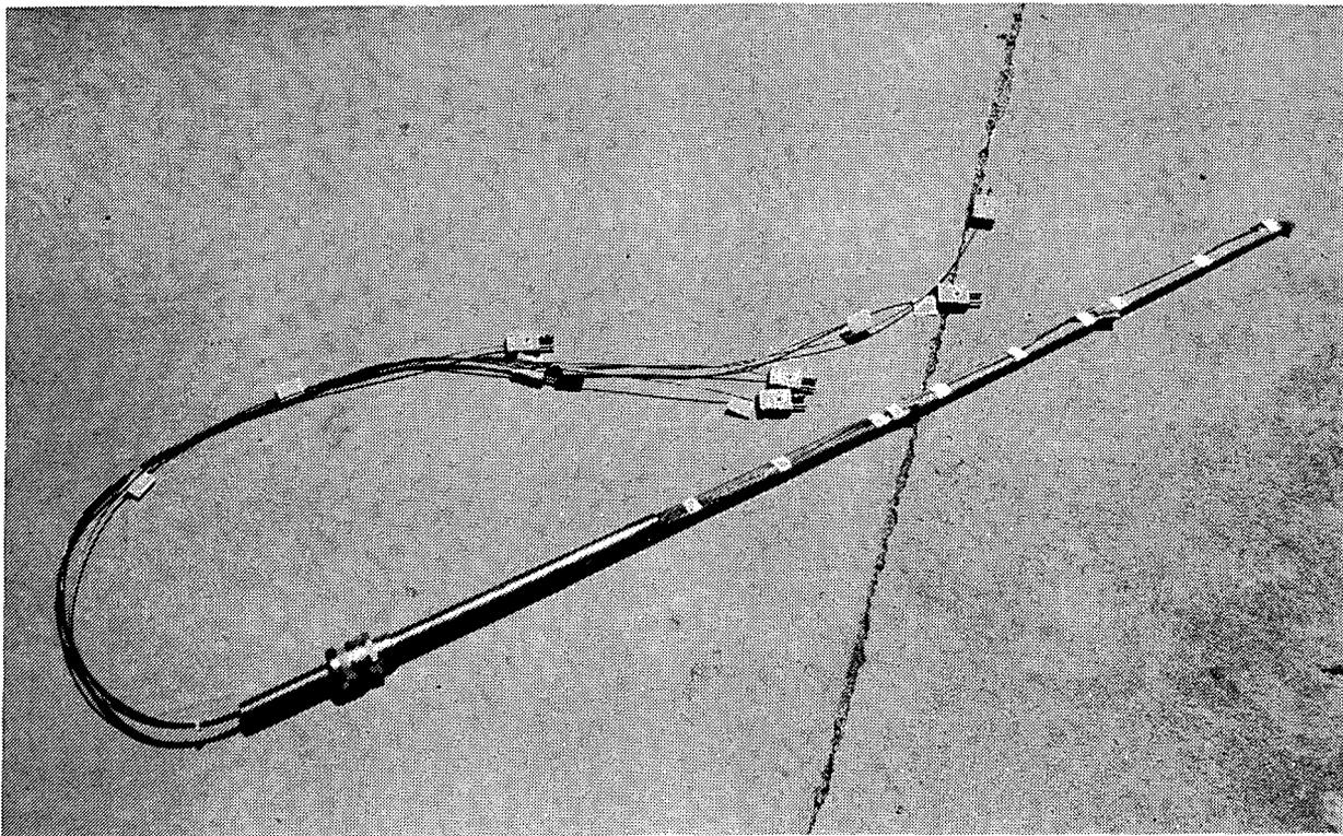
Figure 4. Photograph of Thermocouple Probe
