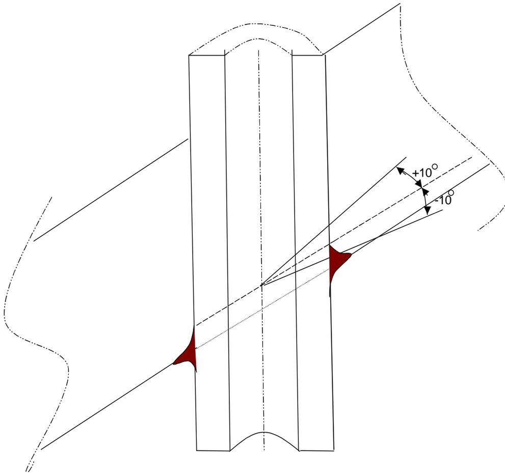
**Fig. 1 Definition of Circumferential Orientation for Flaw Characterization**
