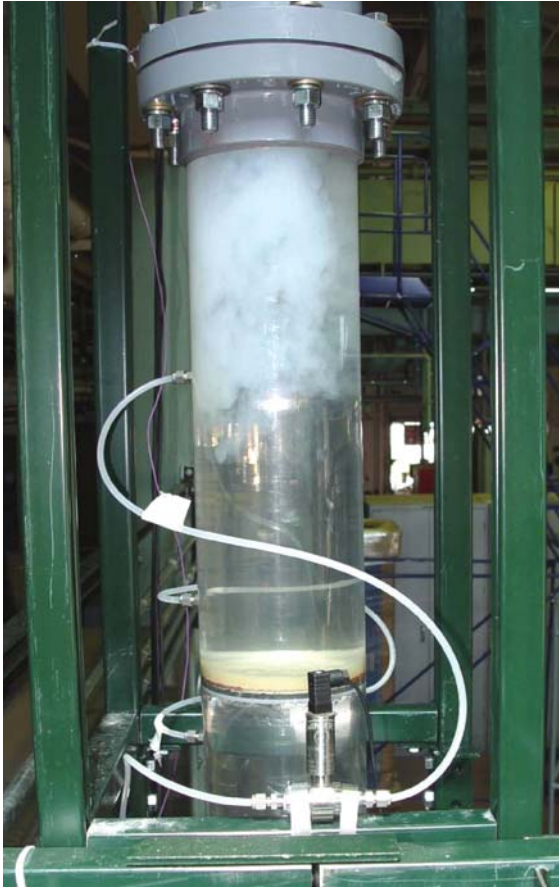
Figure 6. \text{Ca}_3(\text{PO}_4)_2 forming after addition of \text{CaCl}_2 and approaching the debris bed.
