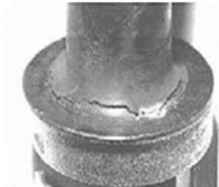
Vessel Internals – Baffle Bolt
