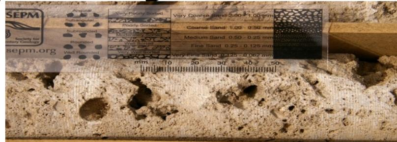
**Small disconnected dissolution voids.**
