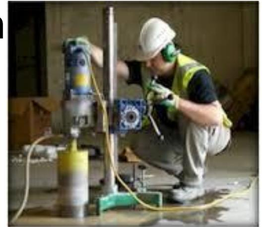
*Concrete coring to obtain samples for evaluating effects of aging and environmental stressors.*
