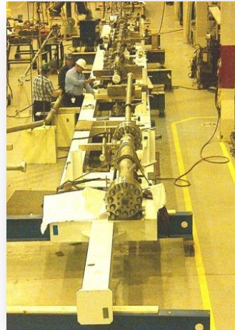
Component prototype testing on reactor coolant pumps and control drive mechanisms
