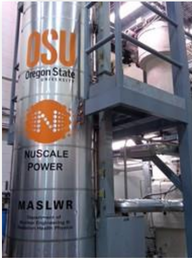
MASLWR integral test facility continues to support NuScale design development and validation.
