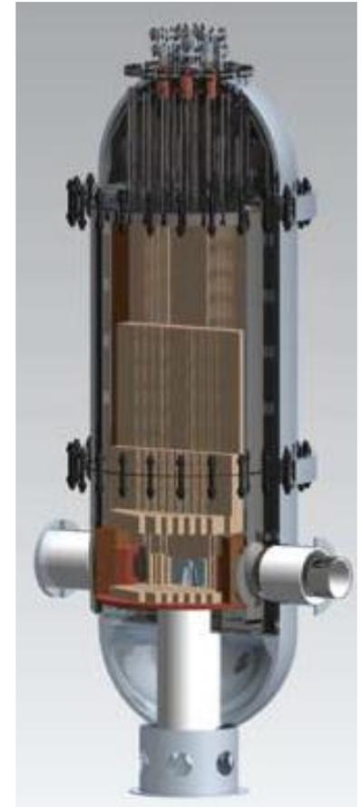
HTGR Reactor Vessel Concept
