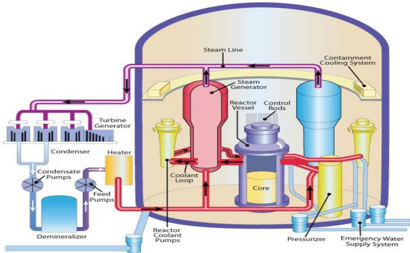
Figure 1 San Onofre Replacement Steam Generator Schematic
