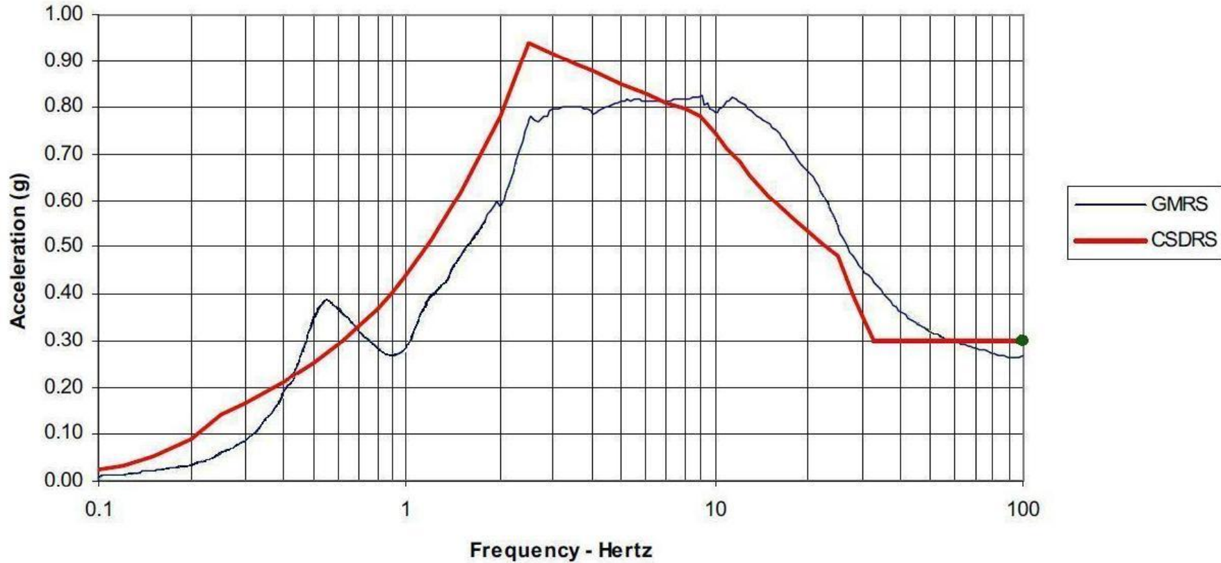
Comparisons of VEGP Horizontal Seismic Response Spectra to AP1000 CSDRS 5% Damping
