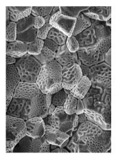
UO<sub>2</sub> fuel pellets consist of crystalline grains with porosity
