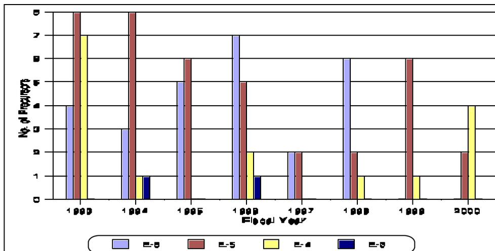
**Figure 2.** Conditional core damage probability results from ASP Program (1993-2000) for each of the CCDP bins ( $E$ -3:  $\geq 1 \times 10^{-3}$ ;  $E$ -4:  $9.9 \times 10^{-4}$  to  $1.0 \times 10^{-4}$ ;  $E$ -5:  $9.9 \times 10^{-5}$  to  $1.0 \times 10^{-5}$ ;  $E$ -6:  $9.9 \times 10^{-6}$  to  $1.0 \times 10^{-6}$ ). Results for FYs 1999 and 2000 are preliminary.
