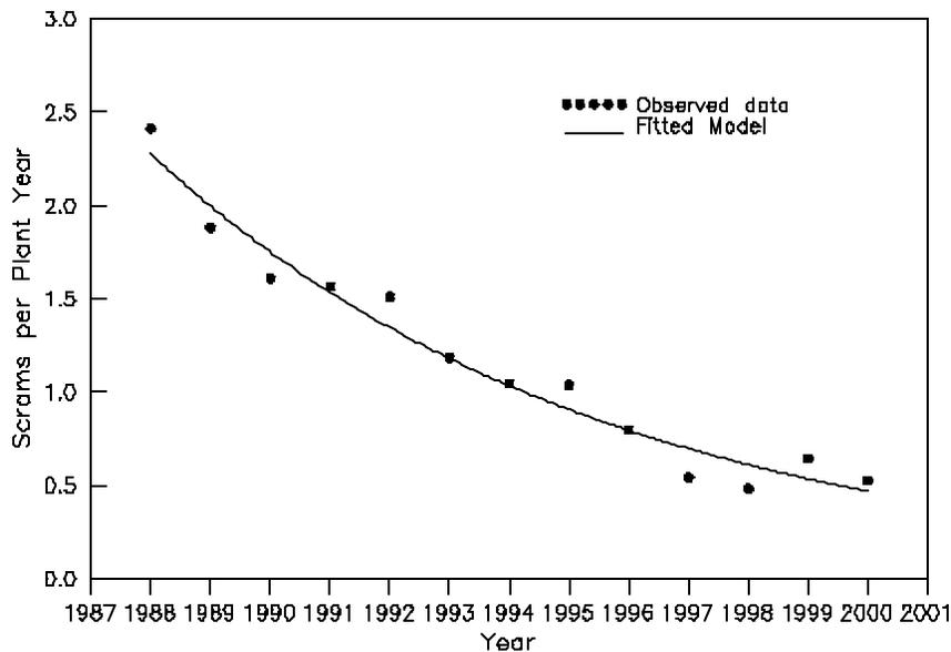
Figure 1: Exponential model fitted to scram data
