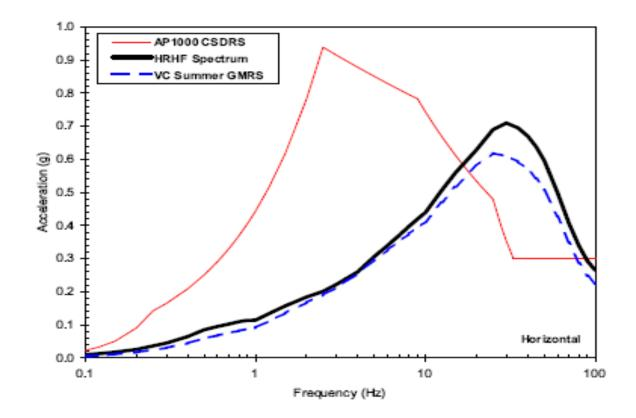
Figure 2.0-201. Comparison Plot of V. C. Summer GMRS and HRHF Spectra for the Horizontal Component of Motion
