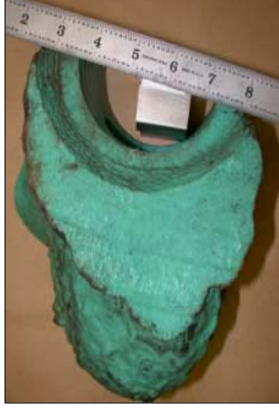
Rubberized Impression of Cavity
