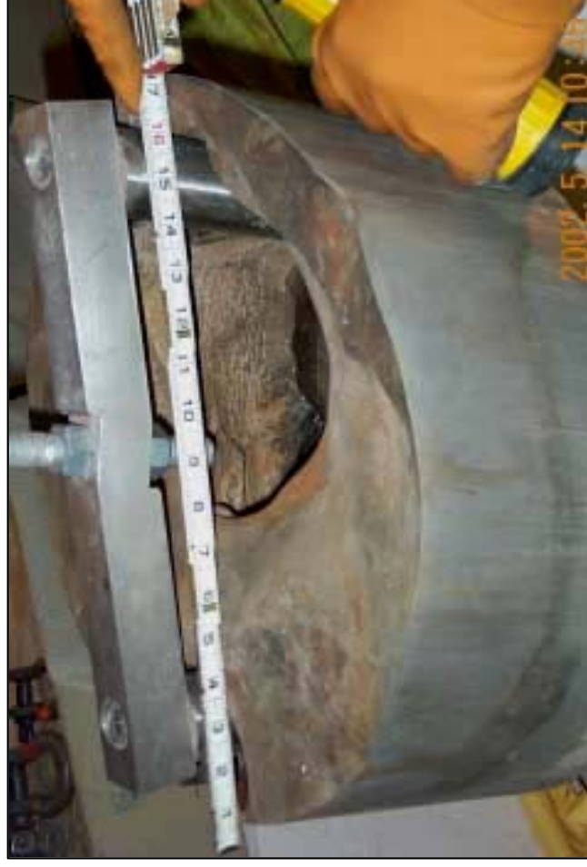
Figure 2-4 DBNPS VHP NOZZLE NO.3 DEGRADATION CAVITY
