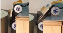
Magnetic wheel robot adheres to magnetic surfaces
