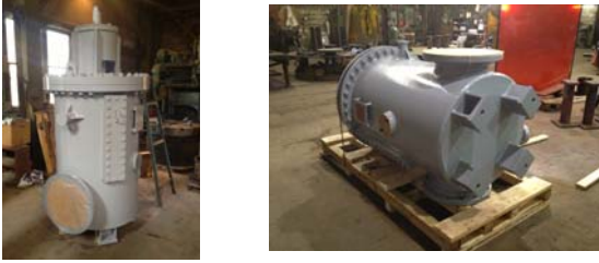
Service Water Strainer
