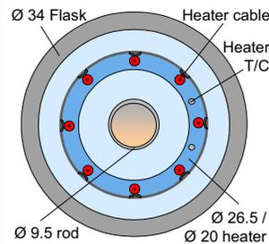
*Cross section of fuel pin, flow separator and pressure tube used in HRP LOCA studies*
