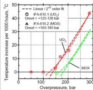
Typical temperature response to overpressure (system pres. 155bar). None of the tests (6) has shown a temperature increase with less than 100bar overpressure.
