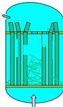
Collapse of fuel with severely oxidized (embrittled) cladding in low-flow incident in cleaning tank at Paks-2 plant in Hungary
