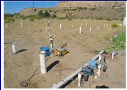
Photo of wells and sampling apparatus including flow cell for measurement of pH, Eh, DO, T, and conductivity during slow purge sampling. Foreground shows injection manifold and stainless steel injection lines to injection wells. [ From Long, Yabusaki et al. 2008 (PNNL-17295) ]
