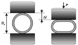
☞ *10CFR50-46*: Cladding oxidation (ECR: 17%) and temperature (PCT: 2200° F) limits derived from Hobson's ring compression tests on oxidized and quenched samples of un-irradiated Zr cladding.
