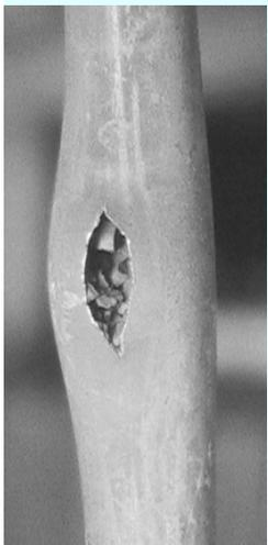
☞ *Do not take into account experimental evidence of relocation of fuel in the ballooned cladding => Recognized to day as non conservative.*
