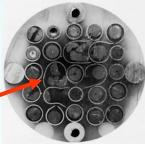
**2. Brittle mode :** Loss of cladding integrity upon quench and post-quench loads
