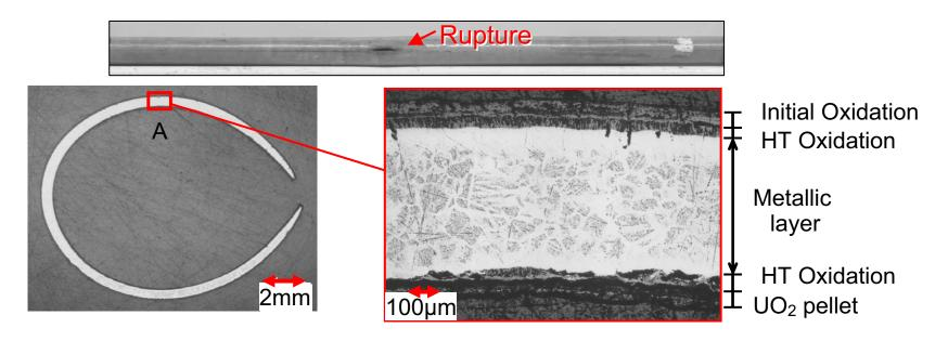
✓ Oxide layers formed during the high temperature period. The oxide layer is not uniform inside the cladding, probably due to thin UO₂ layer.
