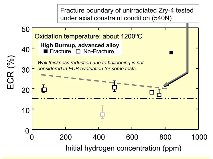
✓ Tests up to ~75 GWd/t ZIRLO, MDA and M5 cladding indicate that the current ECR limit has appreciable safety margin at high burnup.
