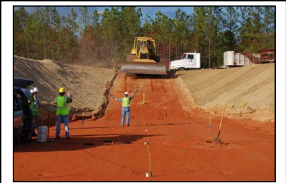
SASW Using Bulldozer as the Source
