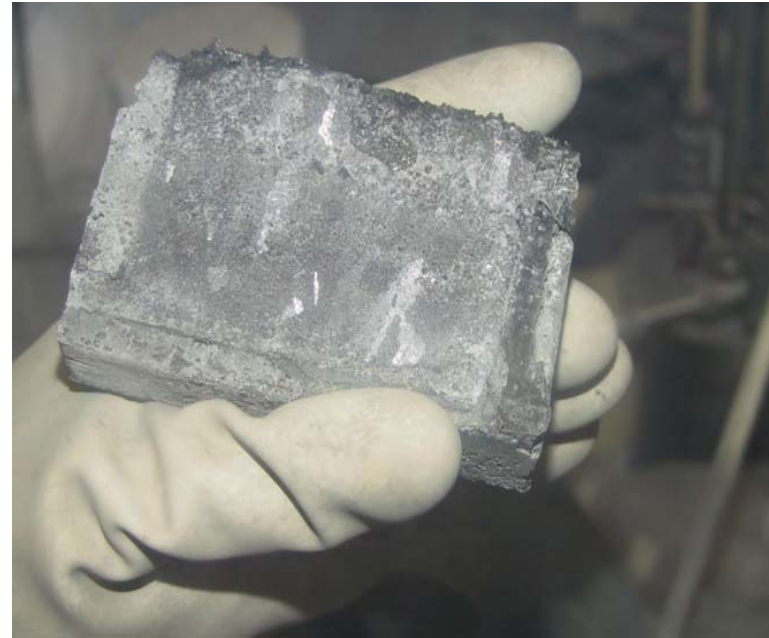
Metallic uranium product from high-capacity reduction cell test
