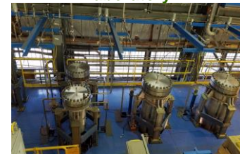
Na-CO 2 Interaction Loop at Argonne National Laboratory
