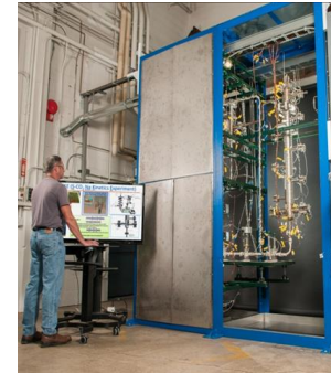
Na-CO 2 Interaction Loop at Argonne National Laboratory
