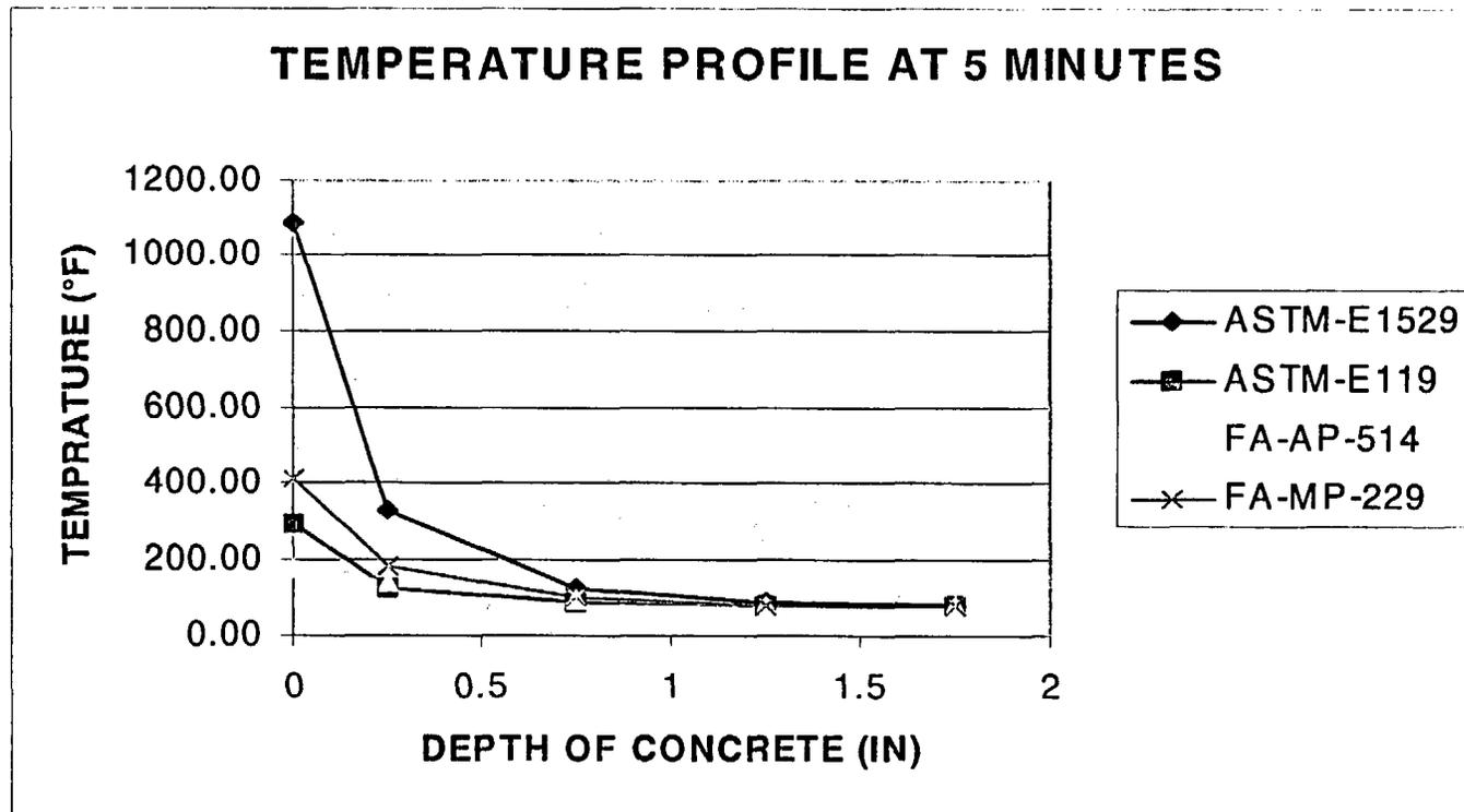
Since two fire areas, even for a short duration, fall outside the E119 curve, a one-dimensional implicit finite difference analysis was performed to determine the temperature effects within the concrete.
