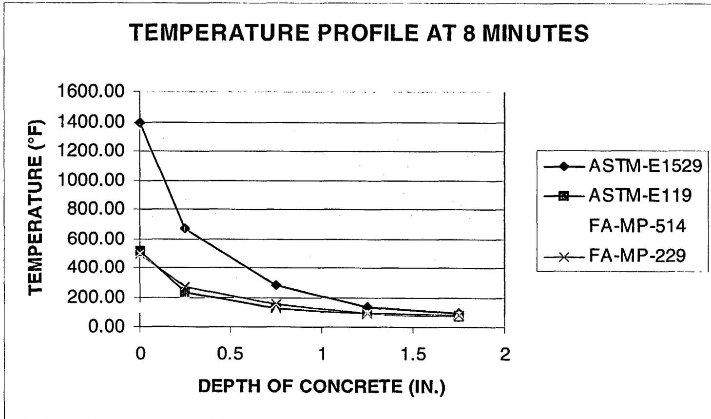
It can be seen from this graph that within 8 minutes, the concrete is within the E119 curve and the concrete temperatures are below 200 °F at 1 inch into the concrete.
