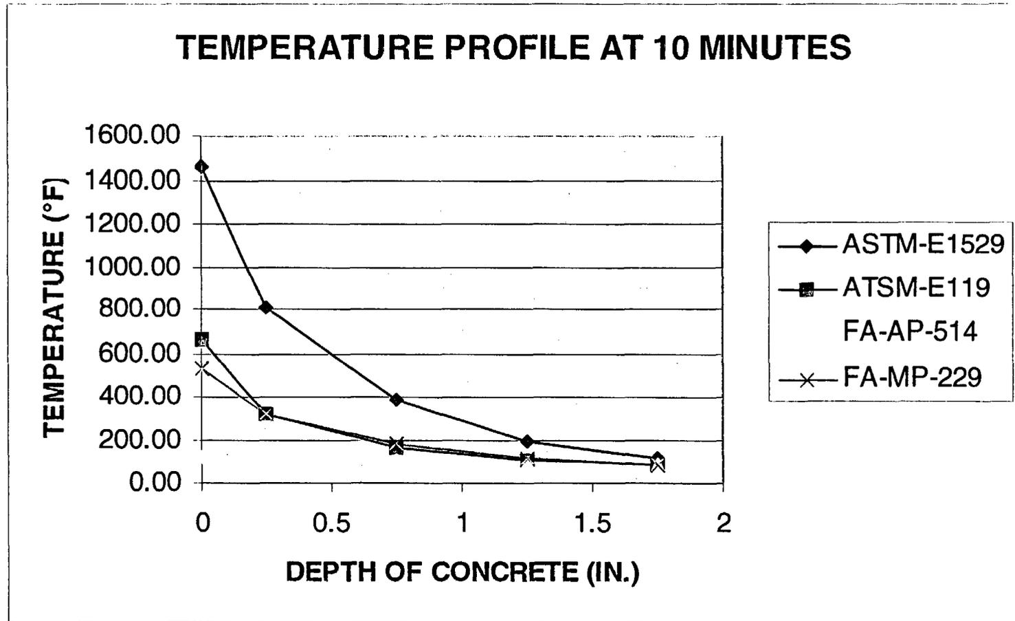
The concrete temperatures at 1 inch are still less than 200°F for the fire areas and E119 curve.
