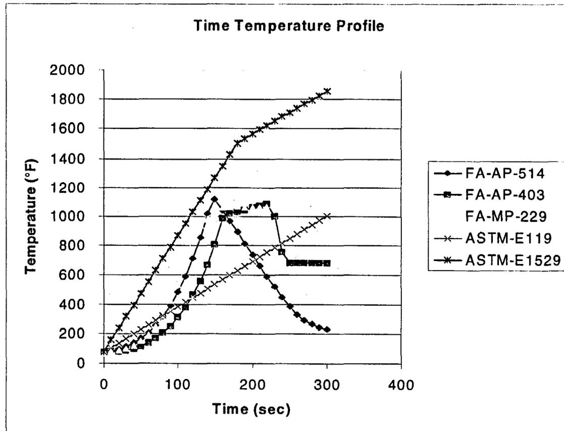
The fire curves during the first 5 minutes with the ASTM-E1529 curve for a comparison.
