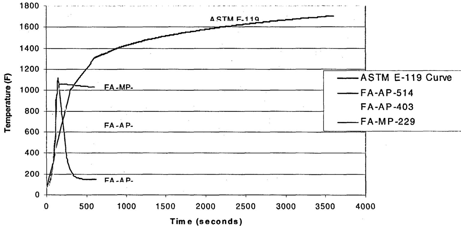
All fire areas have temperatures under the E119 curve within 5 minutes and level off at this point.
