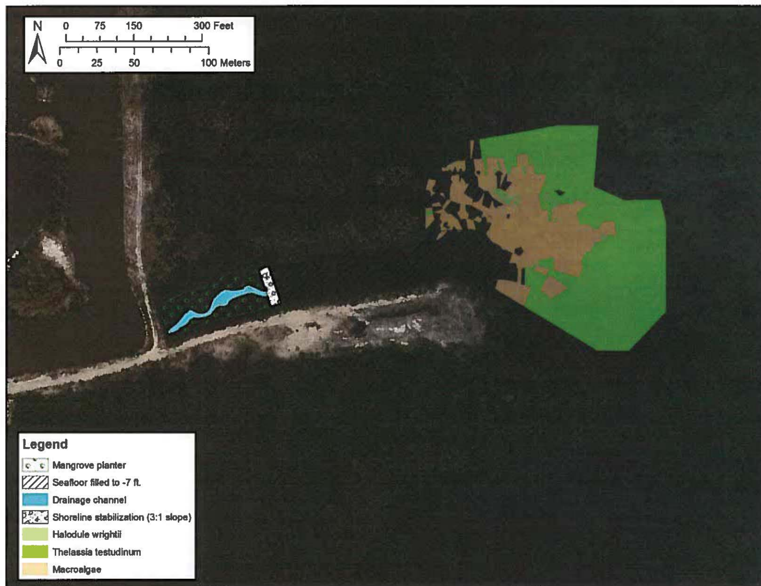
Figure 3-1. Proposed restoration conceptual plan for filling one third of the TPC
