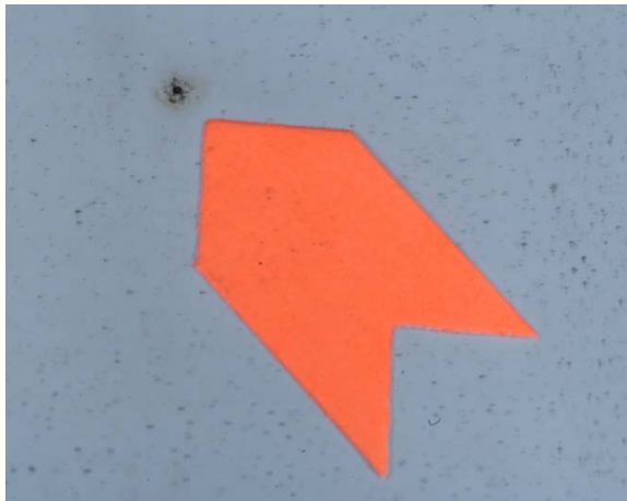
Figure 13. An example of a micro-shorting location on a separator, at the point of shorting, the separator locally melted and shutdown. The micro-short is approximately 1 mm in diameter.
