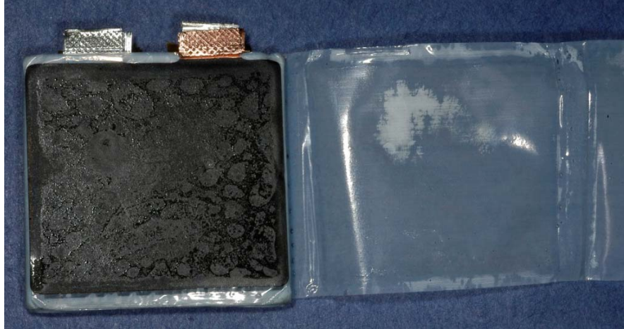
Figure 4. Example of a stacked prismatic cell design.
