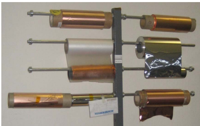
Figure 16. Current collector foils prior to coating with active material.
