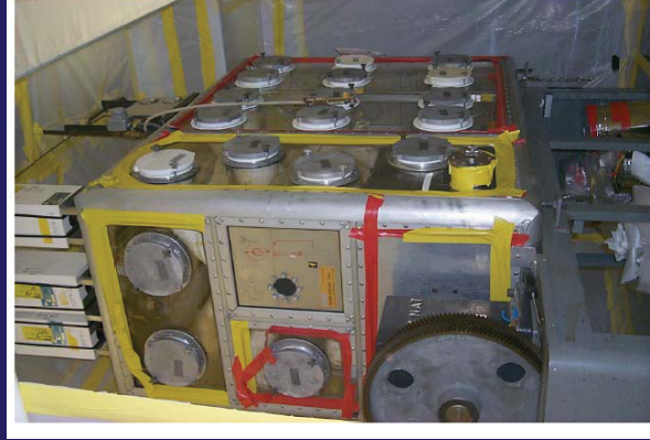
Figure 1. Exterior and interior of glovebox. Note rolling mill inside glovebox was removed prior to decontamination and the floor of the glovebox was swept.
