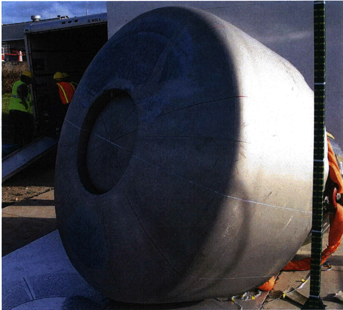
Figure 2-38. Impact Limiter after Head-On Drop – AOS-165A Prototype
