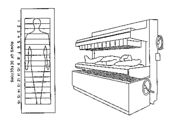
Fig. 2b. A drawing of the upgraded Brookhaven whole-body counter. (Figure provided by Kenneth J. Ellis, Brookhaven National Laboratory)
