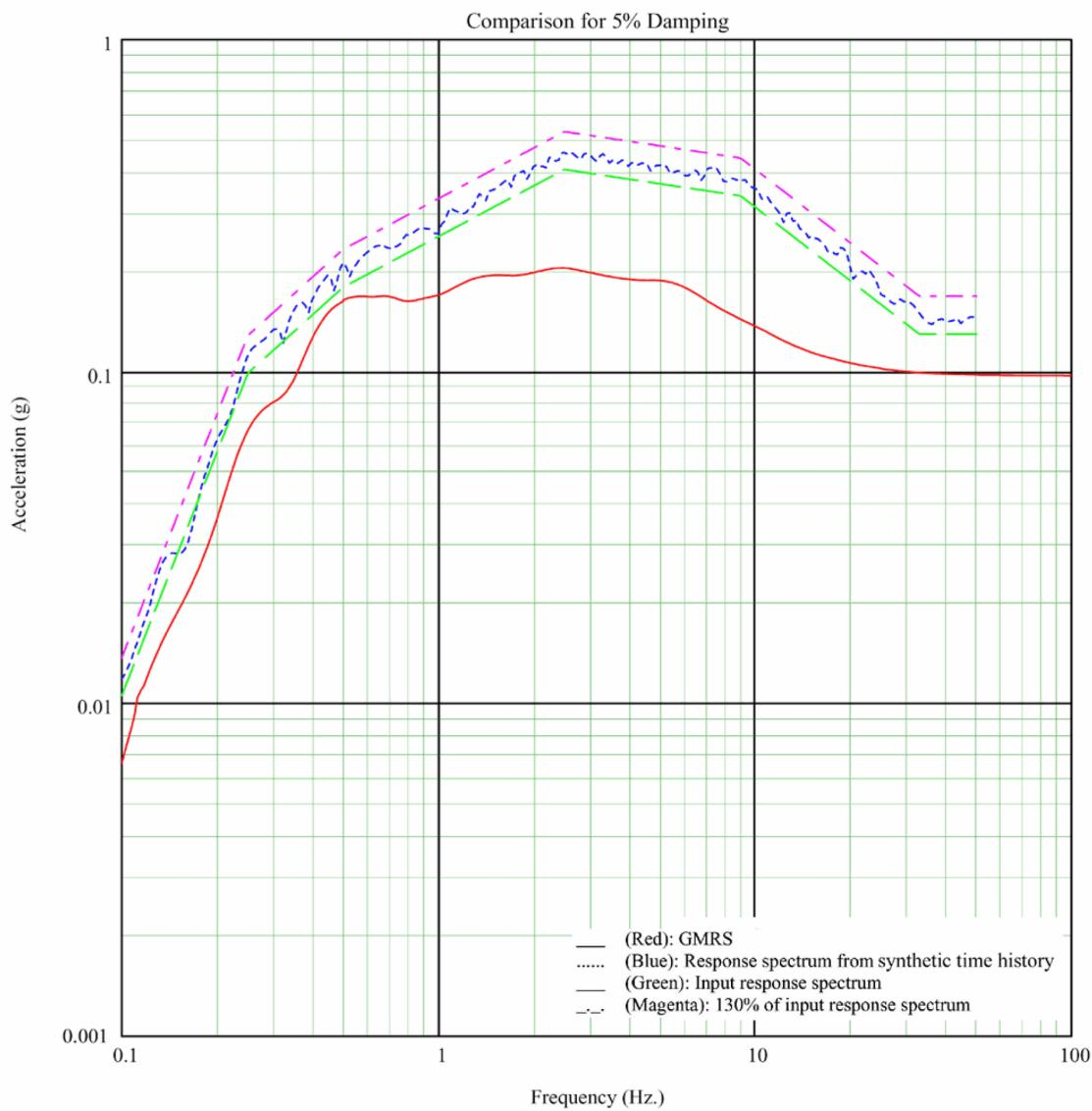
**Figure 3H.6-12 Comparison of Spectrum from Synthetic Time History, Input Spectrum, 130% of Input Spectrum, and GMRS (E-W Direction)**
