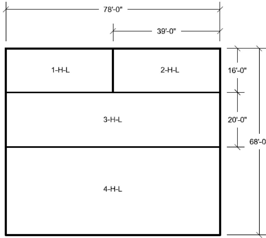
Figure 3H.6-58 Pump House East Wall Looking West Horizontal Reinforcement Zones Far Side Face
