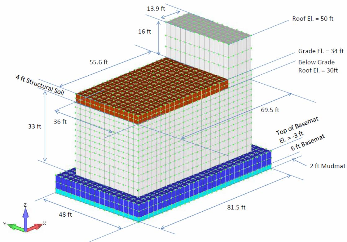
**Figure 3H.6-222 3D Model of DGFOSV for SSI Analysis**
