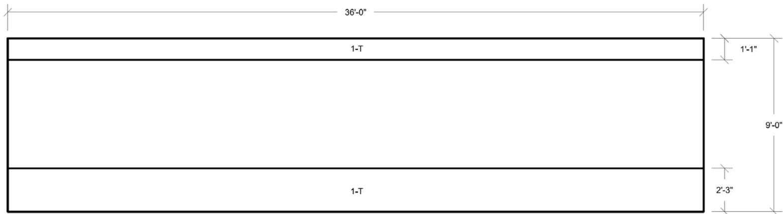
Figure 3H.7-14A Tunnel Walls Looking From Outside Transverse Reinforcement Zones
