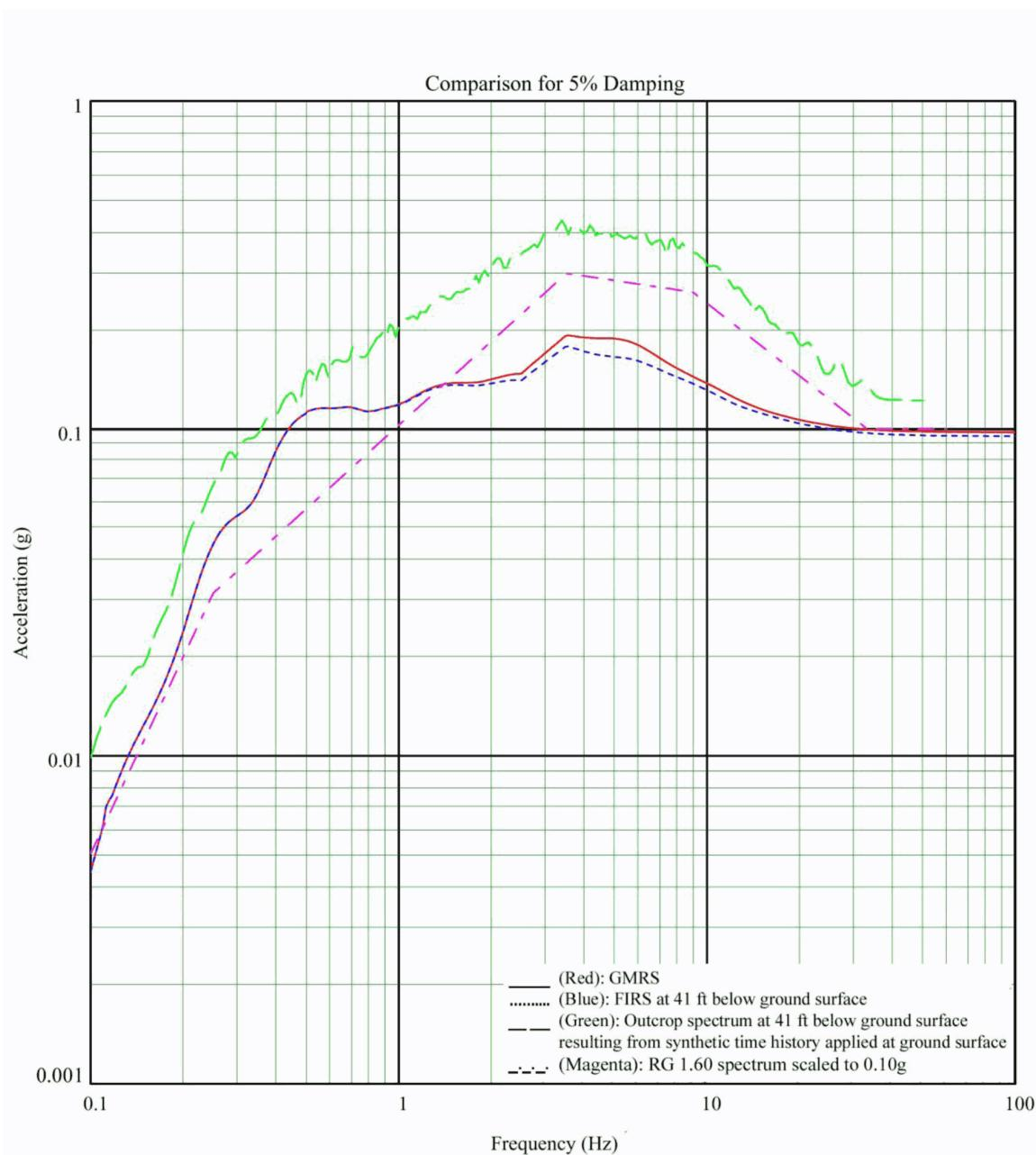
**Figure 3H.6-11k Comparison of Spectra at Foundation of Emergency Diesel Generator Fuel Storage Vault – Upper Bound Soil Properties, Vertical Direction**
