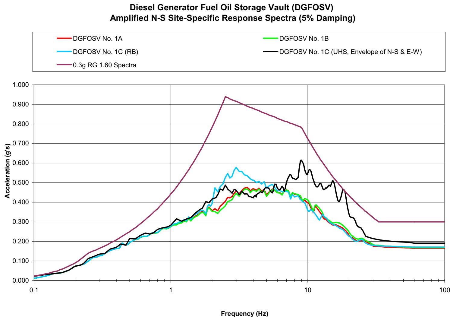
**Figure 3H.6-222a Amplified N-S Site-Specific Response Spectra
