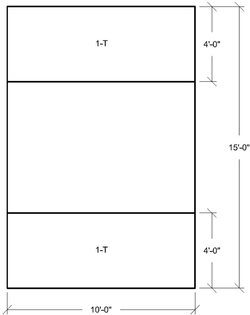
Figure 3H.6-208 Wall 16 Looking From Outside Transverse Reinforcement Zones
