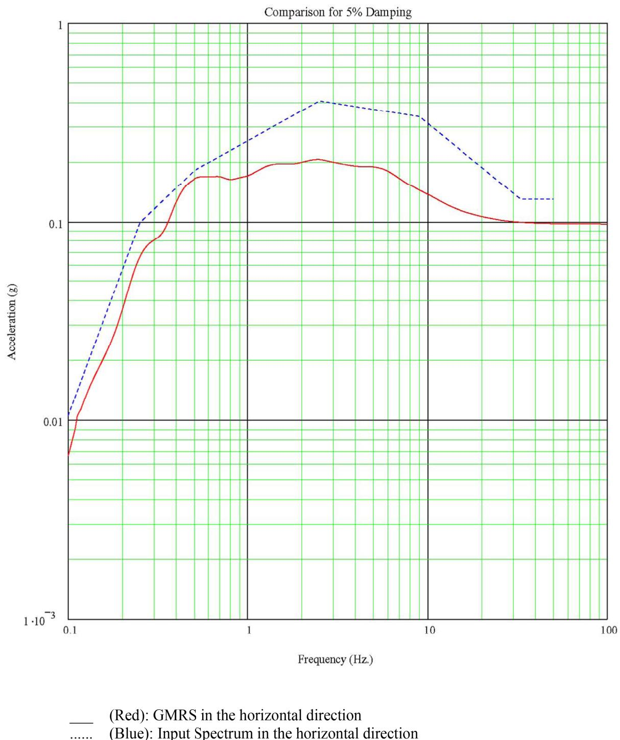
**Figure 3H.6-1 Comparison of GMRS with the Input Spectrum (Horizontal)**
