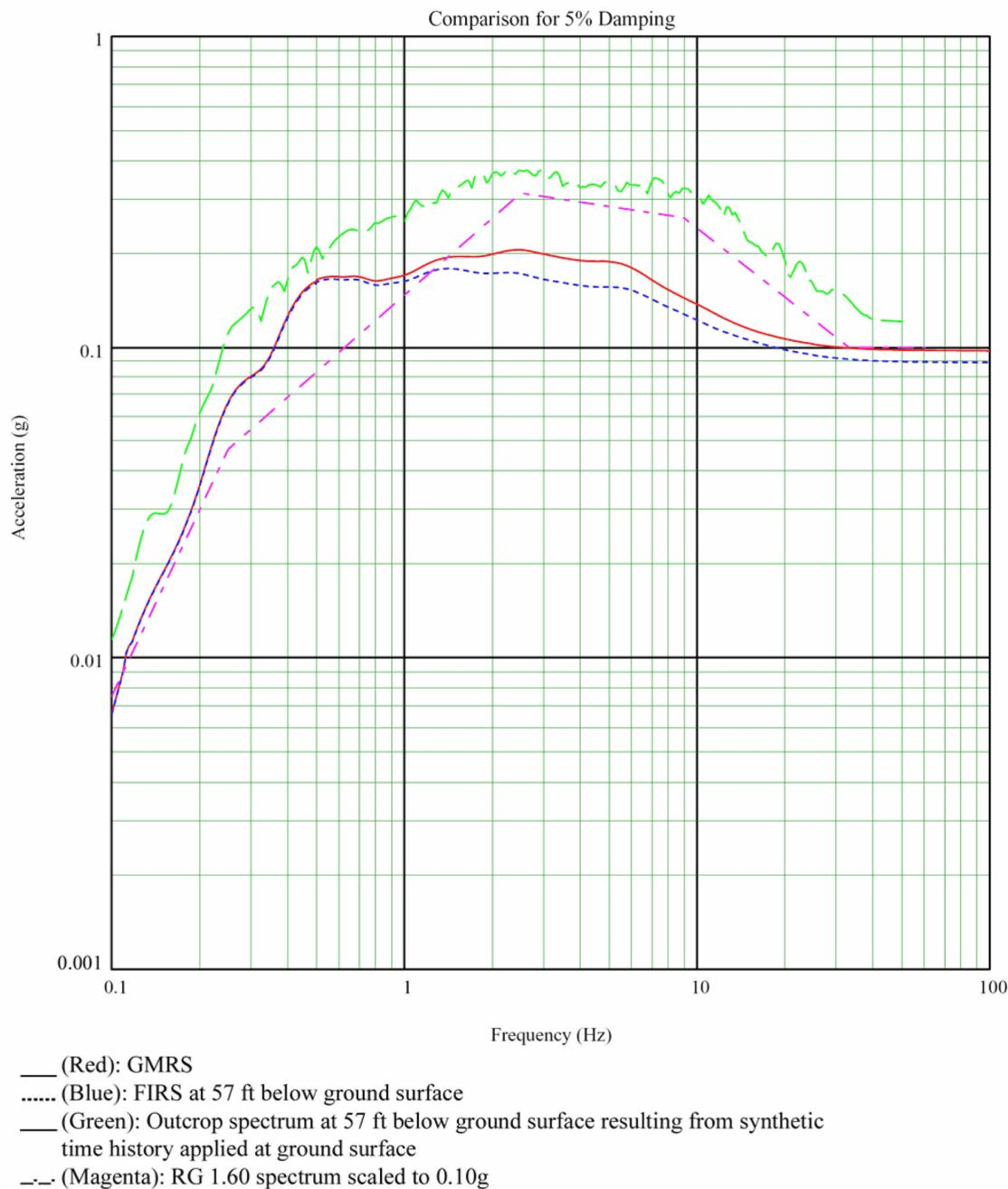
**Figure 3H.6-6a Comparison of Spectra at Foundation of RSW Piping Tunnel (Mean Soil Properties, E-W Direction)**
