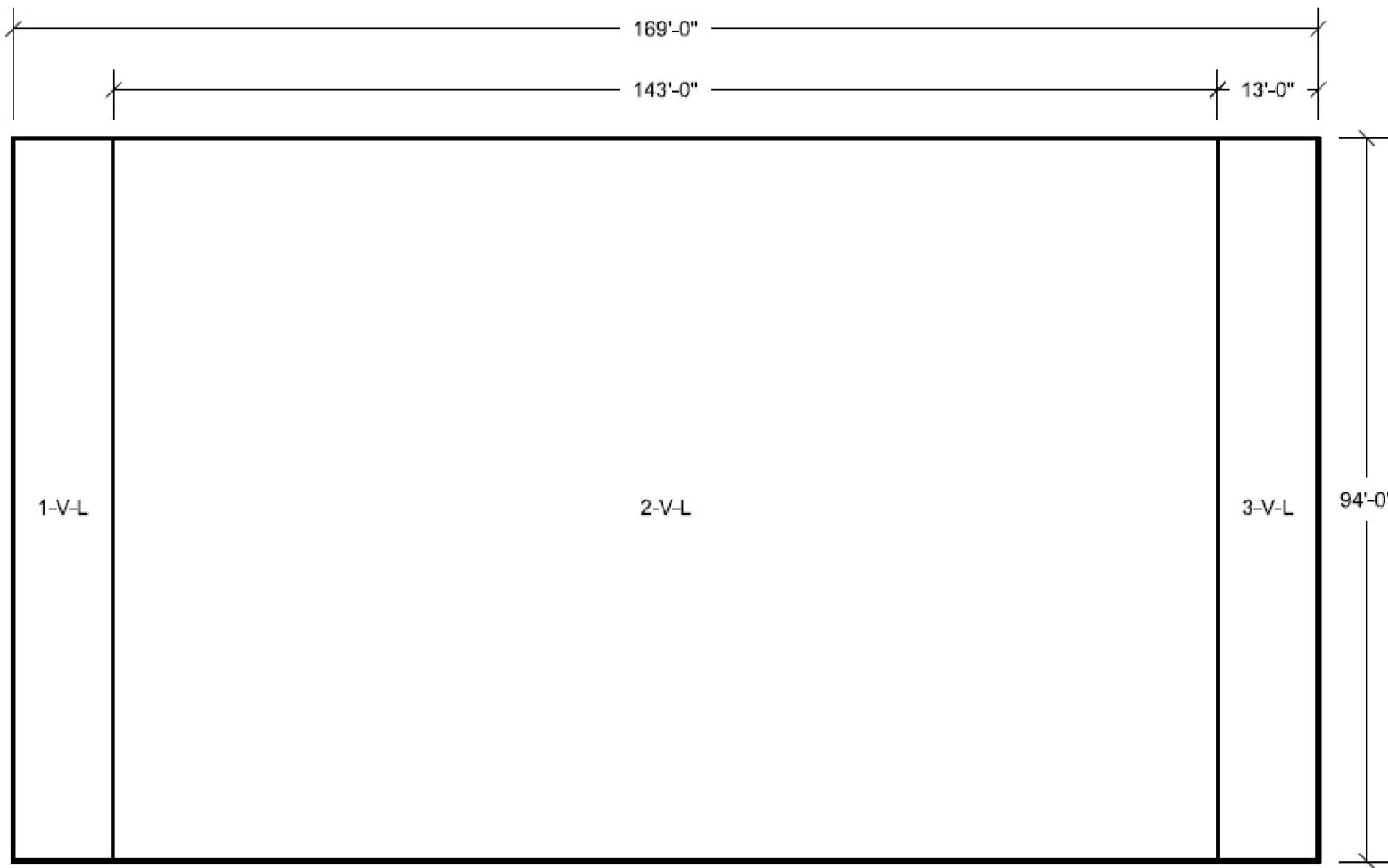
**Figure 3H.6-126 Pump House Foundation Mat North/South Reinforcement Zones Bottom Face**
