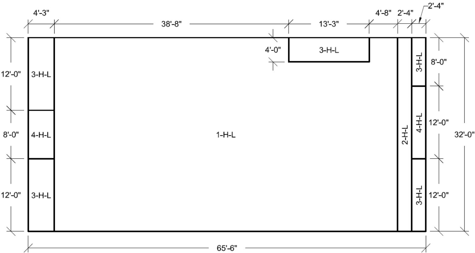
Figure 3H.6-163 Wall 7 Looking From Outside Horizontal Reinforcement Zones Near Side Face
