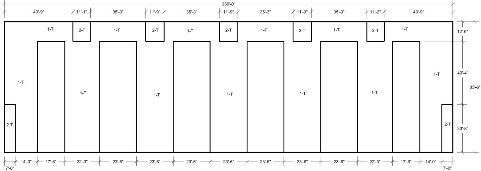
Figure 3H.6-91 UHS Basin South Wall Looking North Transverse **Horizontal Reinforcing** **Reinforcement** Zones
