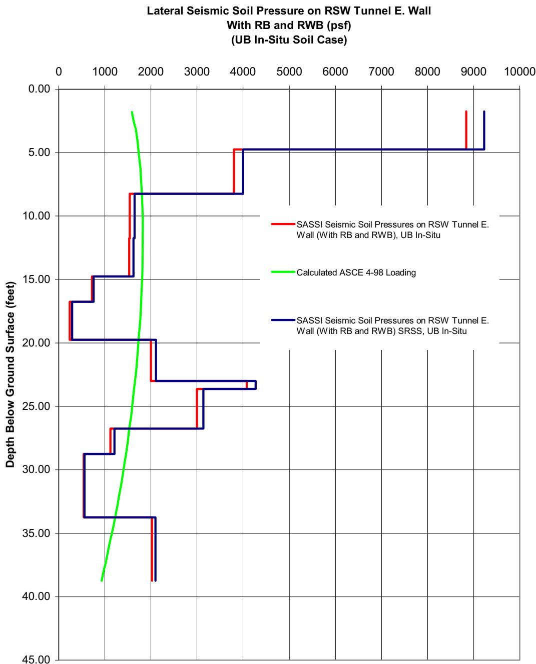
**Figure 3H.6-216 Lateral Seismic Soil Pressures (psf) on RSW Piping Tunnel East Wall For UB In-Situ Soil Case (Main Cross Section of RSW Piping Tunnel, Including Effect of Vertical Excitation)**
