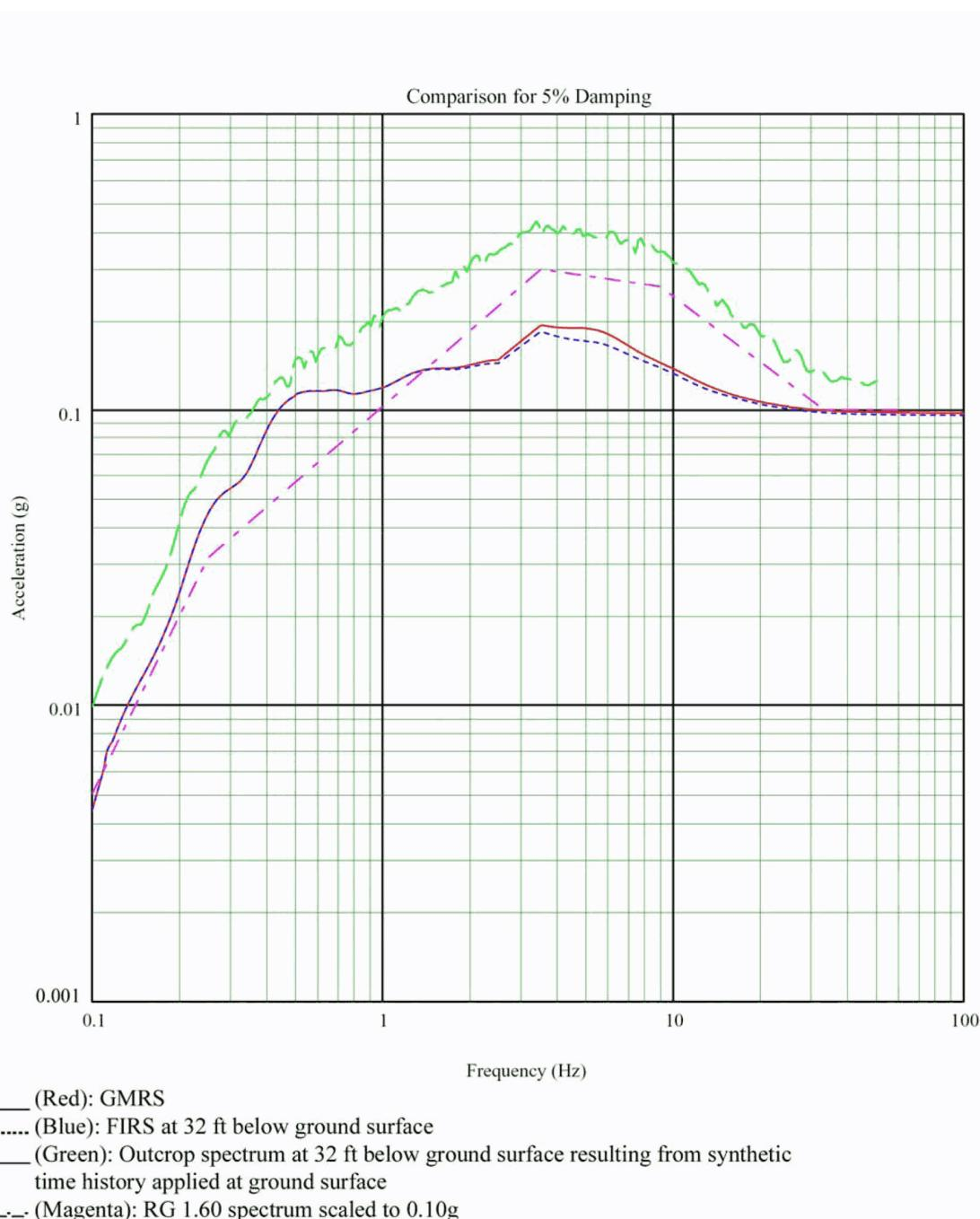
**Figure 3H.6-5a Comparison of Spectra at Foundation of UHS Basin (Mean Soil Properties, Vertical Direction)**
