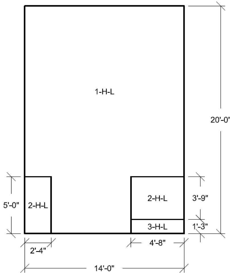
Figure 3H.6-177 Wall 10 Looking From Outside Horizontal Reinforcement Zones Near Side Face
