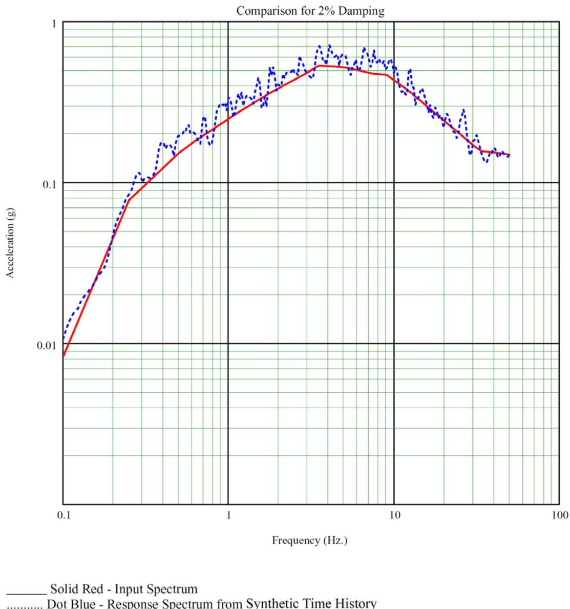
**Figure 3H.6-14a Comparison of Input Spectrum and Spectrum from Synthetic Time History, Vertical – 2% Damping**
