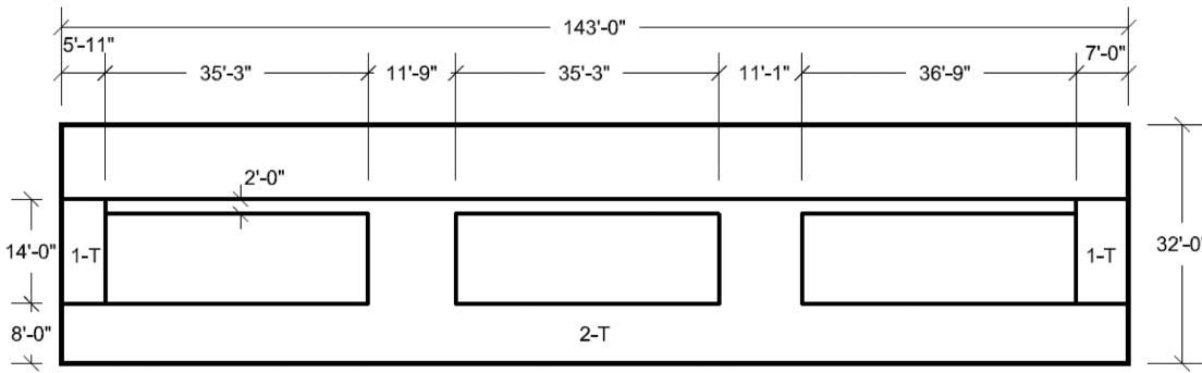
Figure 3H.6-65 Pump House South Wall Looking South Transverse ~~Horizontal~~ Reinforcement Zones
