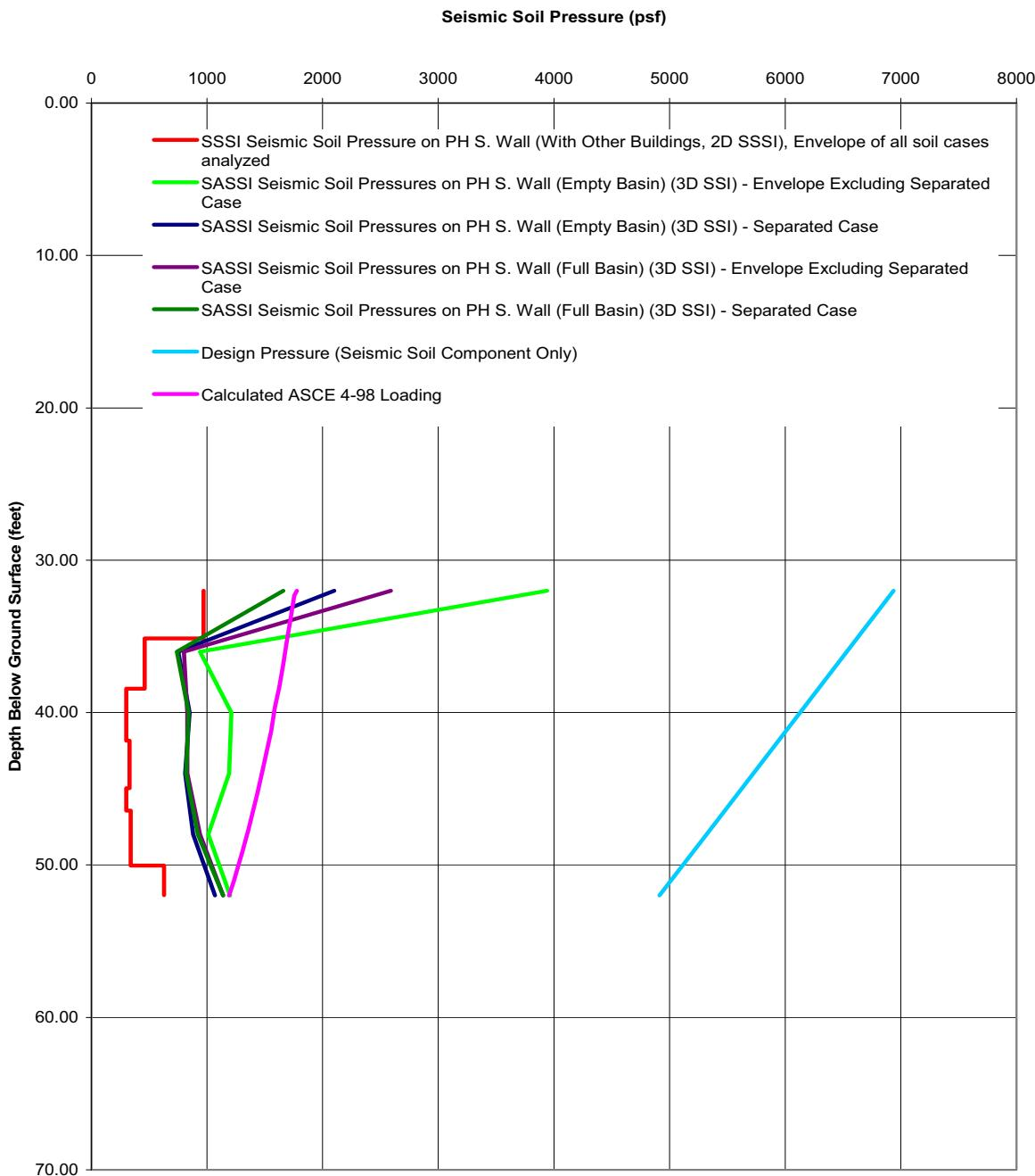
**Figure 3H.6-218 SSI, SSSI, ASCE 4-98 and Design Lateral Seismic Soil Pressures on RSW Pump House South Wall**
