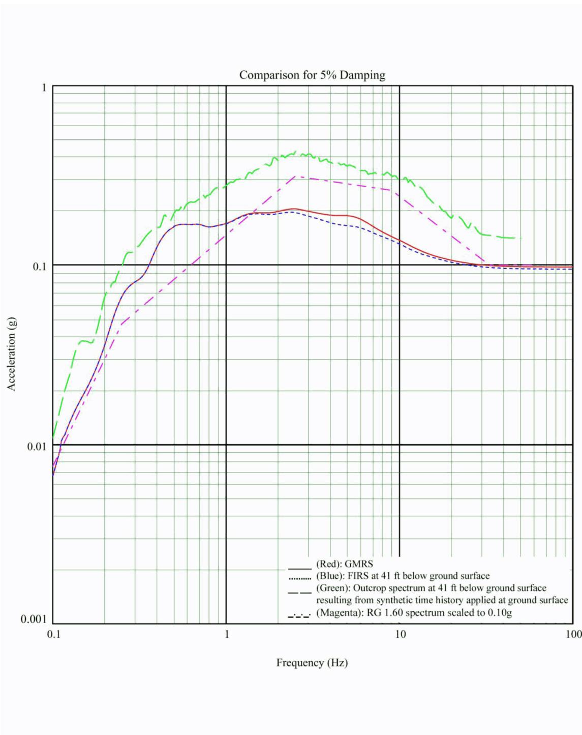
**Figure 3H.6-11h Comparison of Spectra at Foundation of Emergency Diesel Generator Fuel Storage Vault – Upper Bound Soil Properties, N-S Direction**
