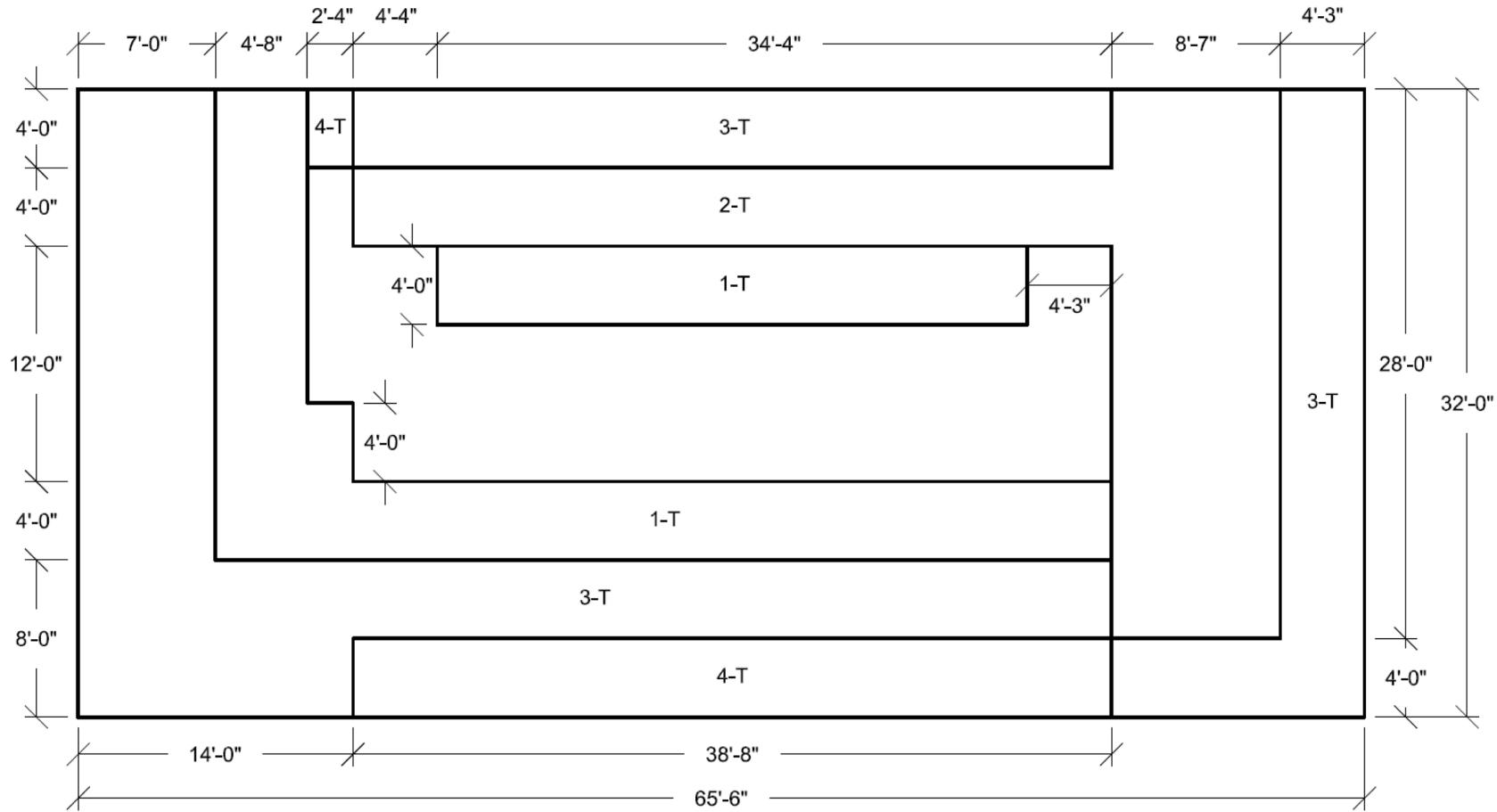
Figure 3H.6-172 Wall 8 Looking From Outside Transverse Reinforcement Zones
