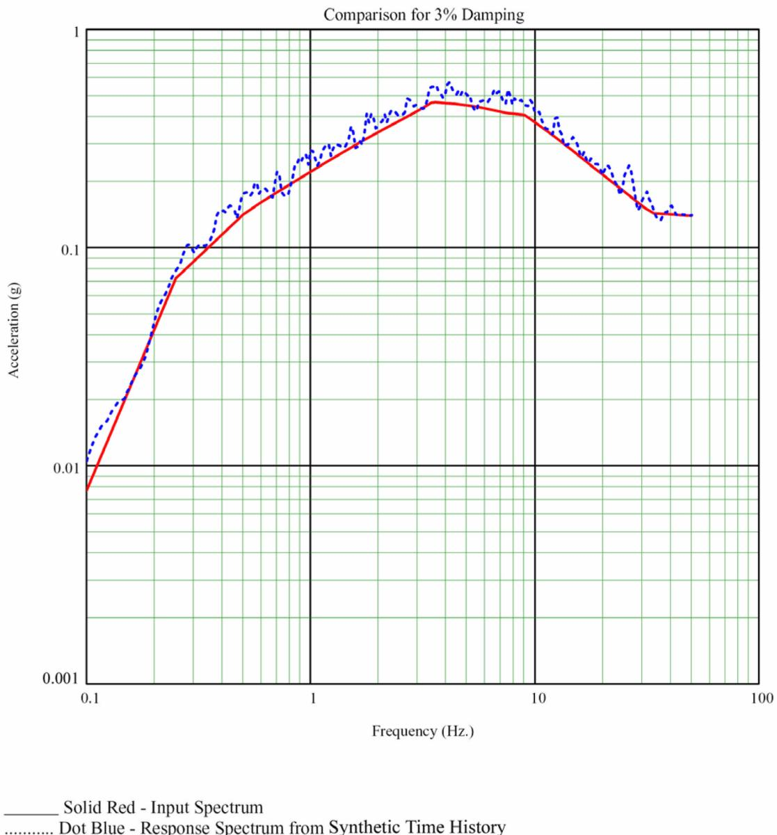
**Figure 3H.6-14b Comparison of Input Spectrum and Spectrum from Synthetic Time History, Vertical – 3% Damping**
