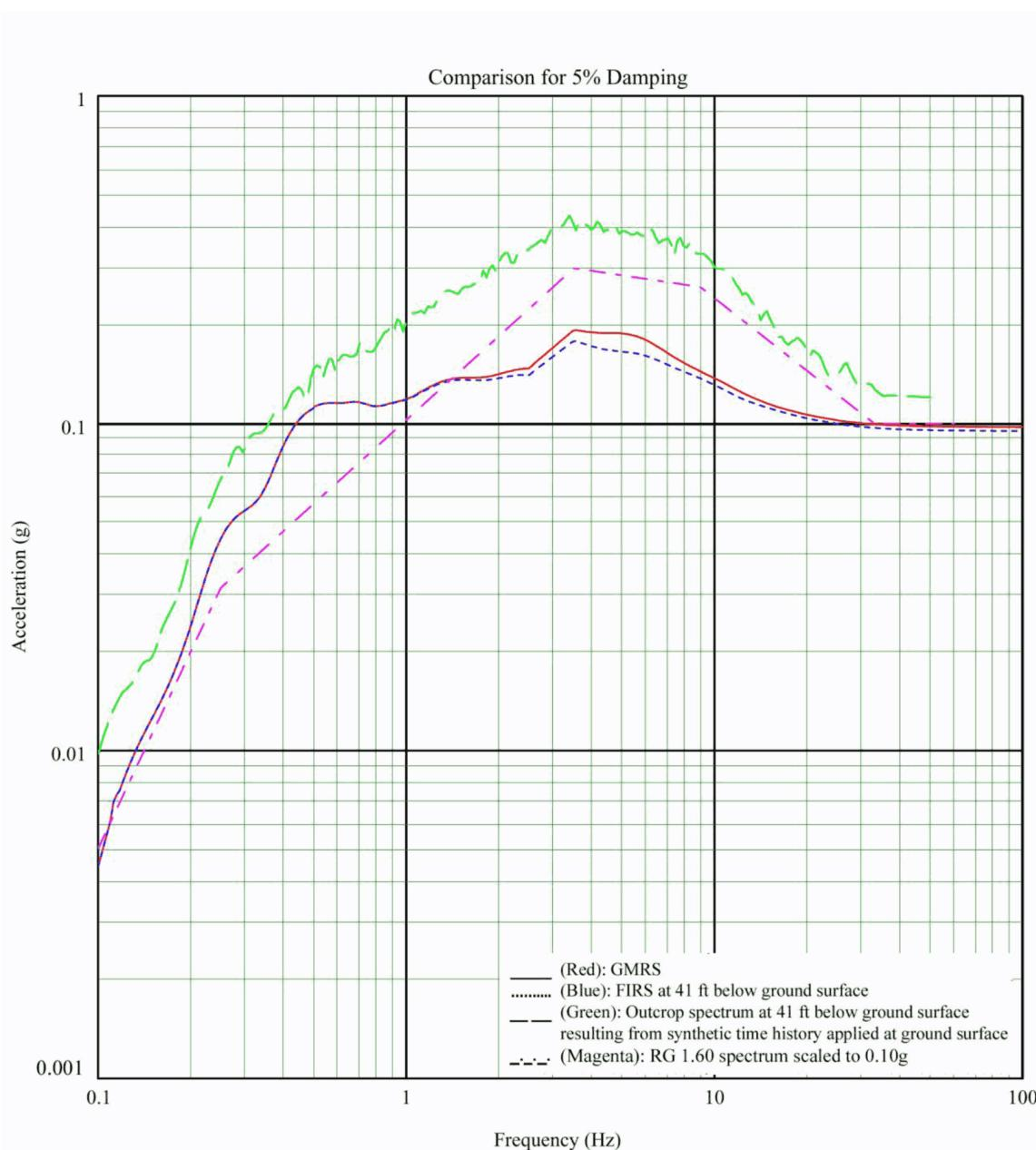
**Figure 3H.6-11L Comparison of Spectra at Foundation of Emergency Diesel Generator Fuel Storage Vault – Lower Bound Soil Properties, Vertical Direction**
