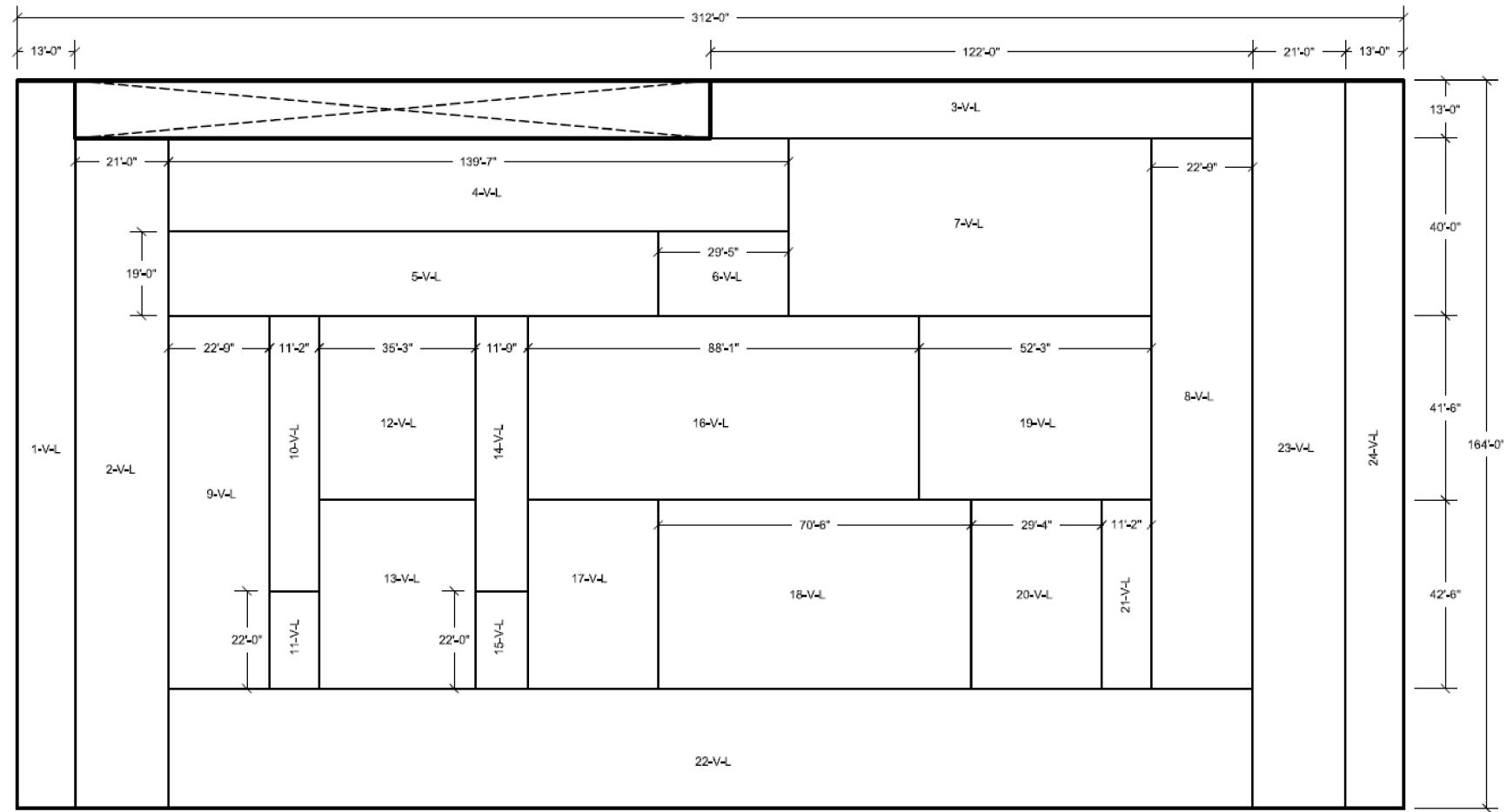
Figure 3H.6-132 UHS Basin Foundation Mat-Plan
