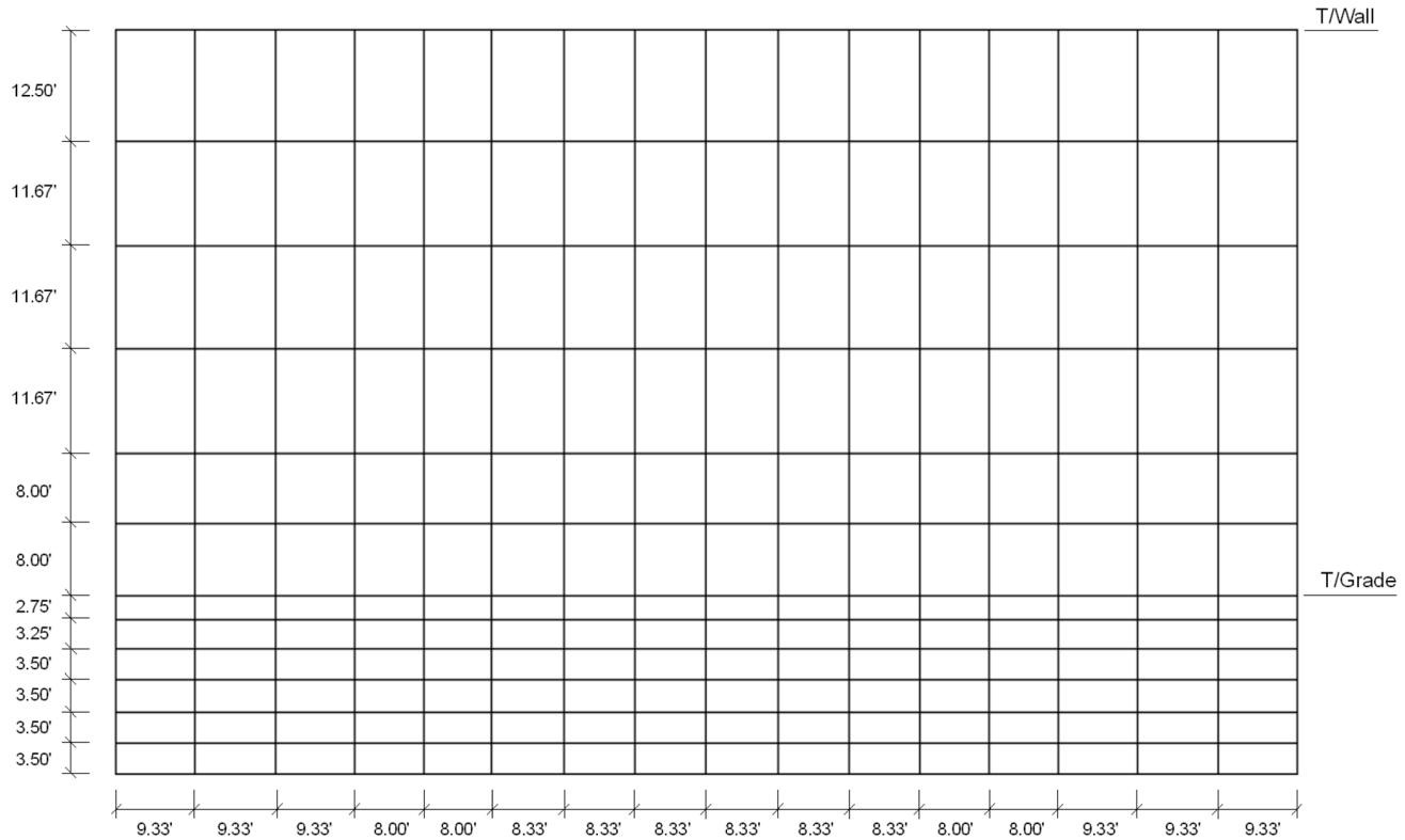
Note: Basin East and West Walls have the same mesh. The mesh is symmetrical about the vertical axis such that the view is the same whether looking at the wall from the inside or outside of the basin.
