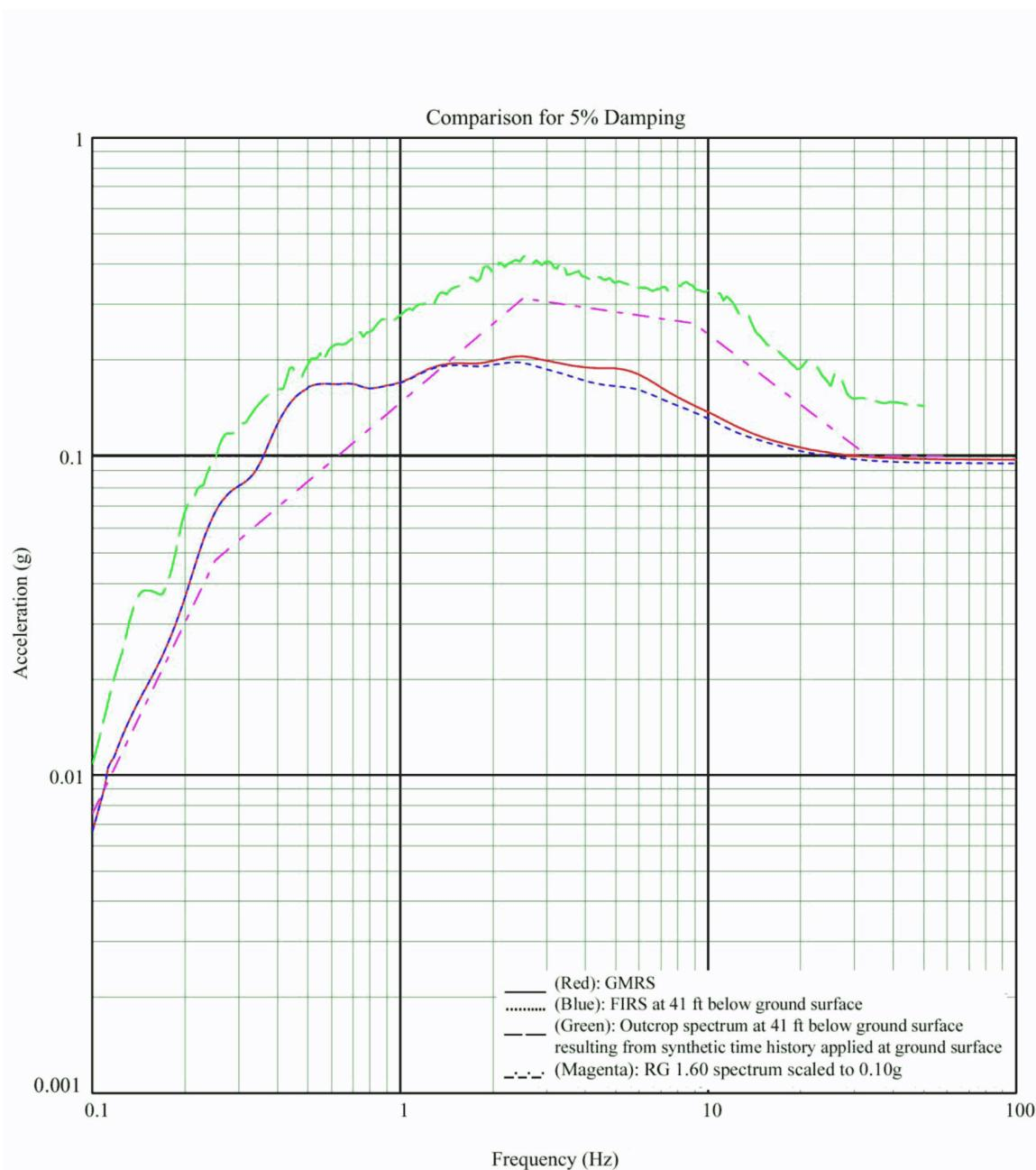
**Figure 3H.6-11g Comparison of Spectra at Foundation of Emergency Diesel Generator Fuel Storage Vault – Mean Soil Properties, N-S Direction**
