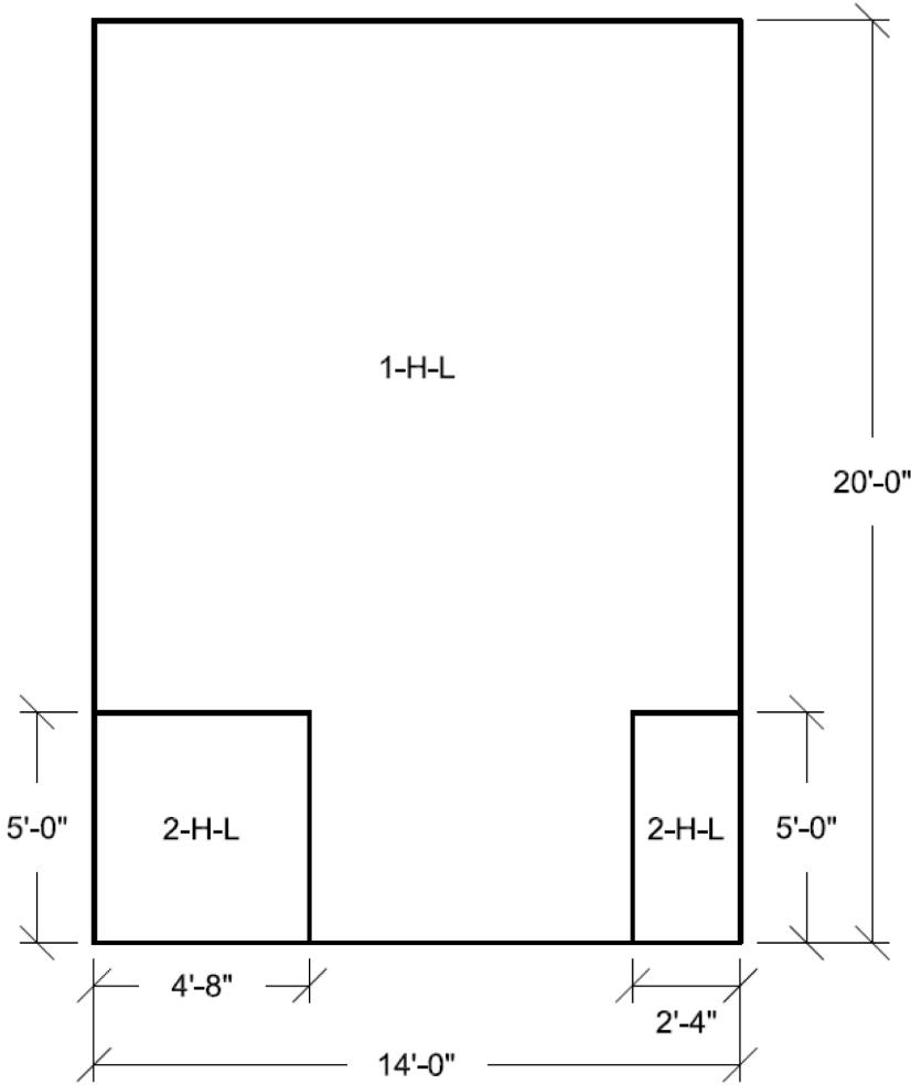
Figure 3H.6-175 Wall 9 Looking From Outside Horizontal Reinforcement Zones Far Side Face
