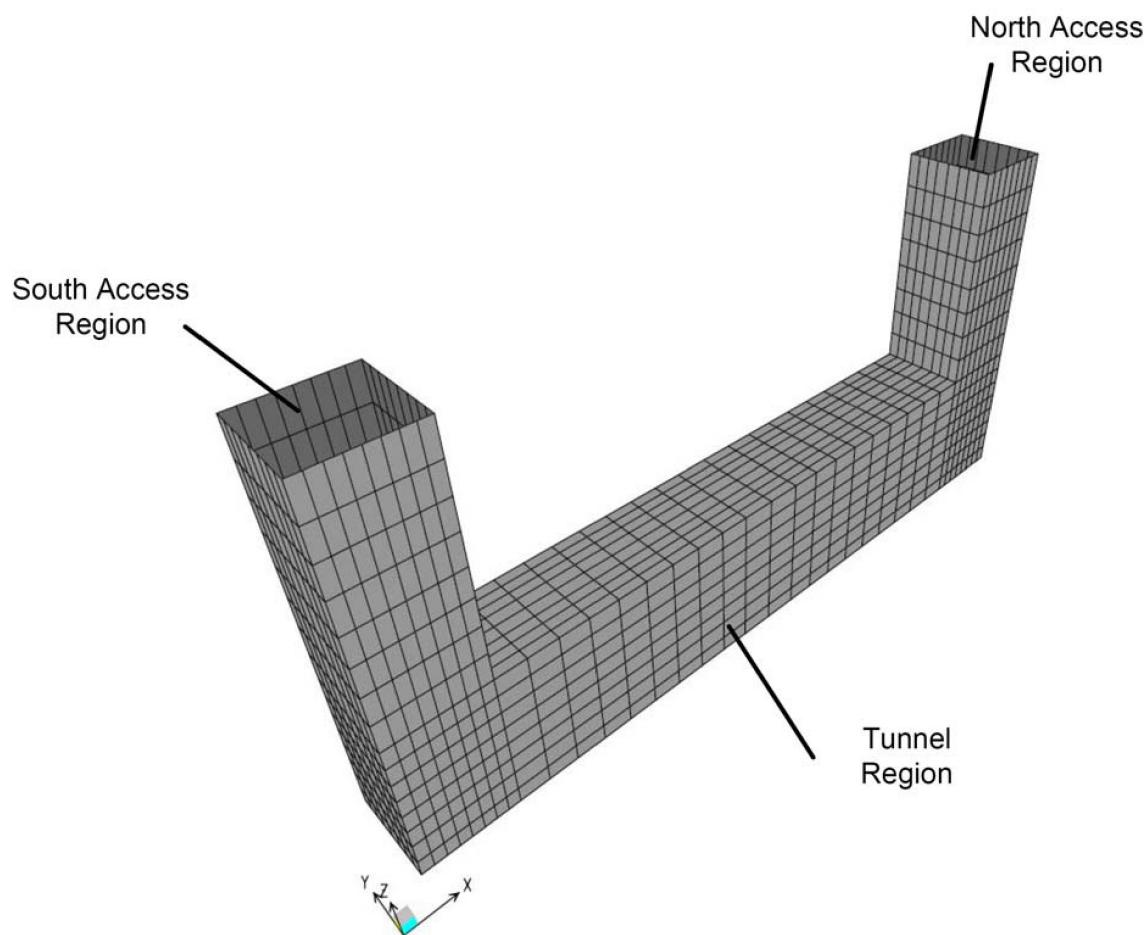
**Figure 3H.7-1 SAP2000 Finite Element Analysis Model for DGFOT**
