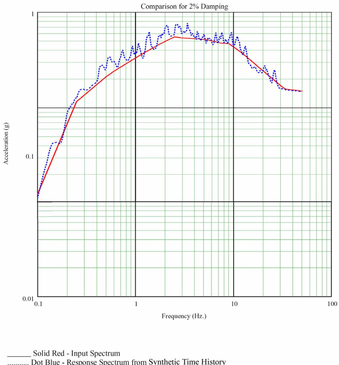
**Figure 3H.6-13a Comparison of Input Spectrum and Spectrum from Synthetic Time History, Horizontal (N-S) – 2% Damping**
