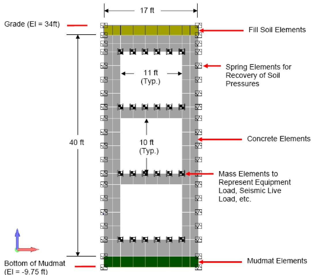
**Figure 3H.6-209 SSI Model of RSW Piping Tunnel**
