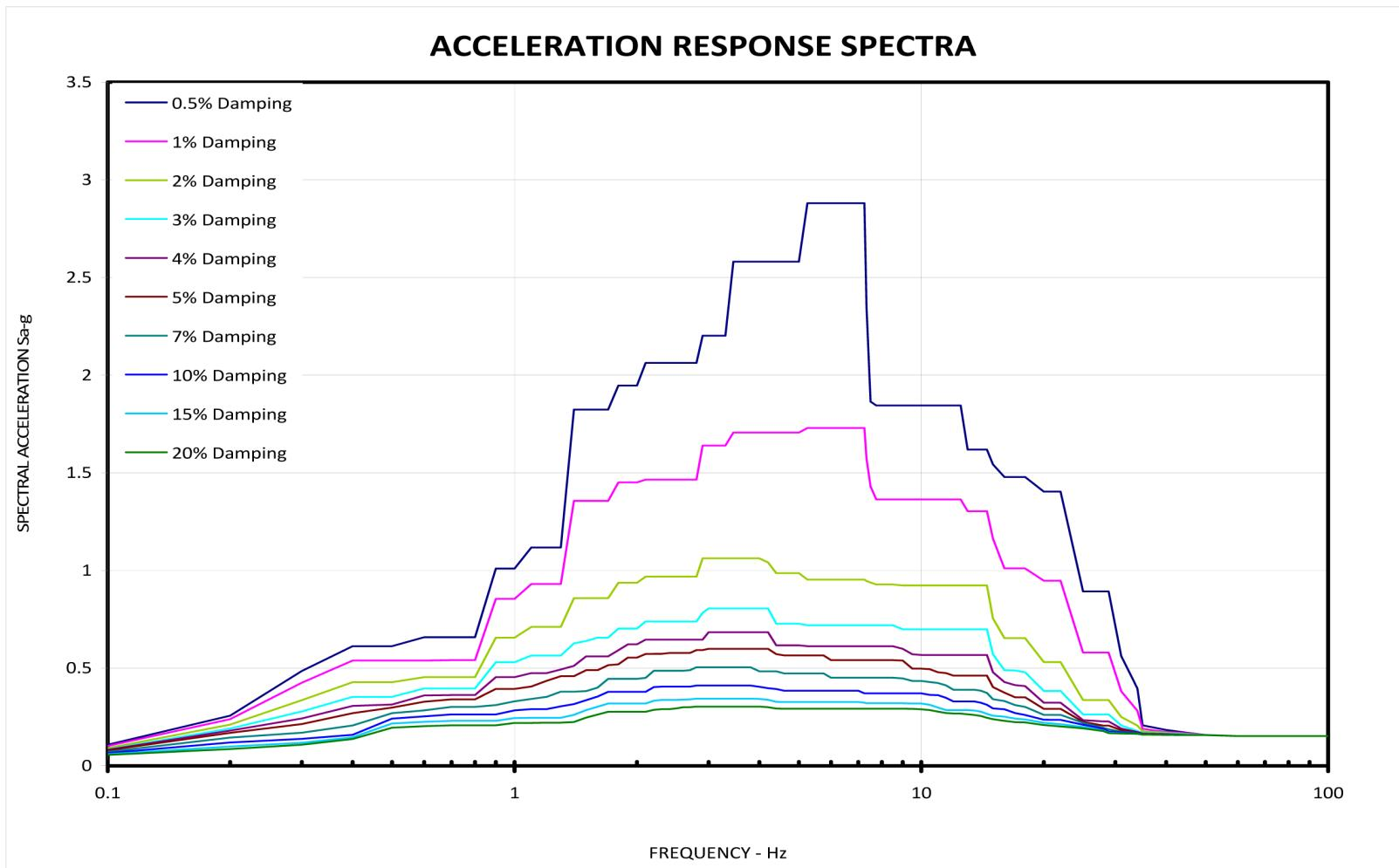
Figure 3H.6-138 RSW Piping Tunnel, Horizontal Response Spectra
