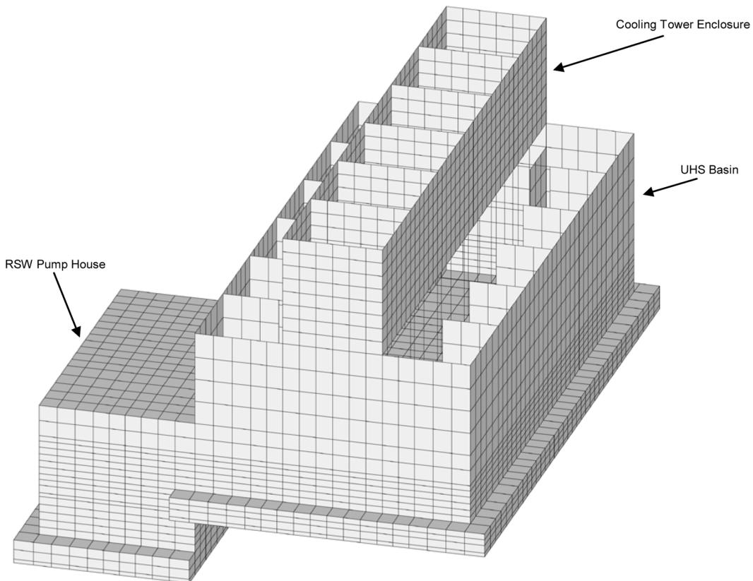
**Figure 3H.6-15a SSI Model (structure only)**
