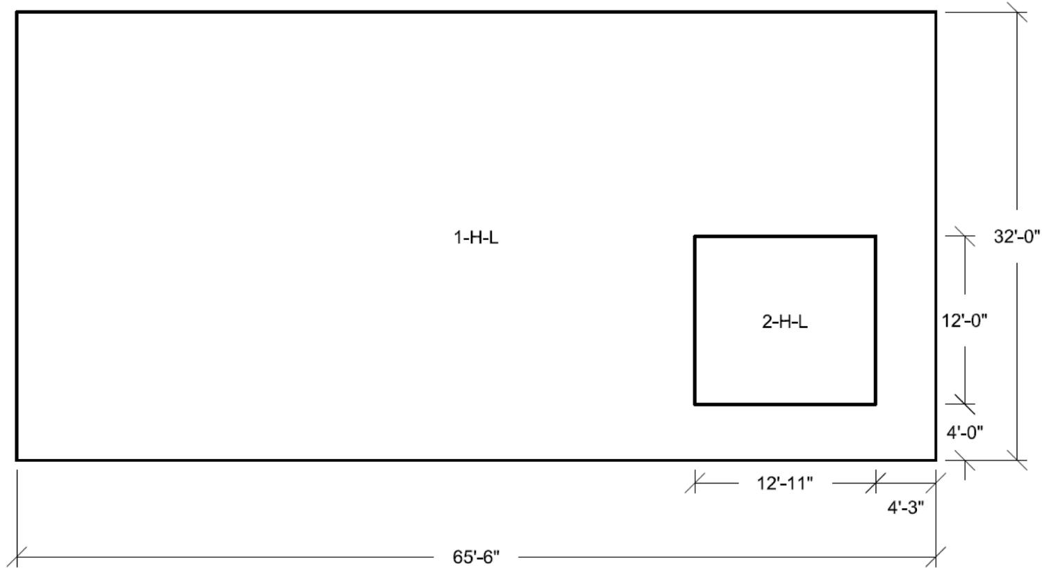
Figure 3H.6-170 Wall 8 Looking From Outside Horizontal Reinforcement Zones Far Side Face
