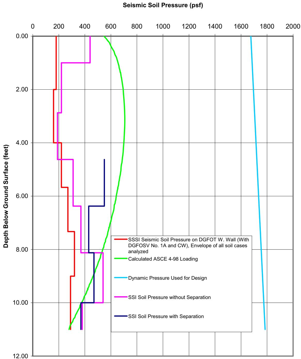
**Figure 3H.7-8 SSI, SSSSI, ASCE 4-98 and Design Lateral Seismic Soil Pressures (psf) on Fuel Oil Tunnel West Wall with Diesel Generator Fuel Oil Storage Vault and Crane Wall**
