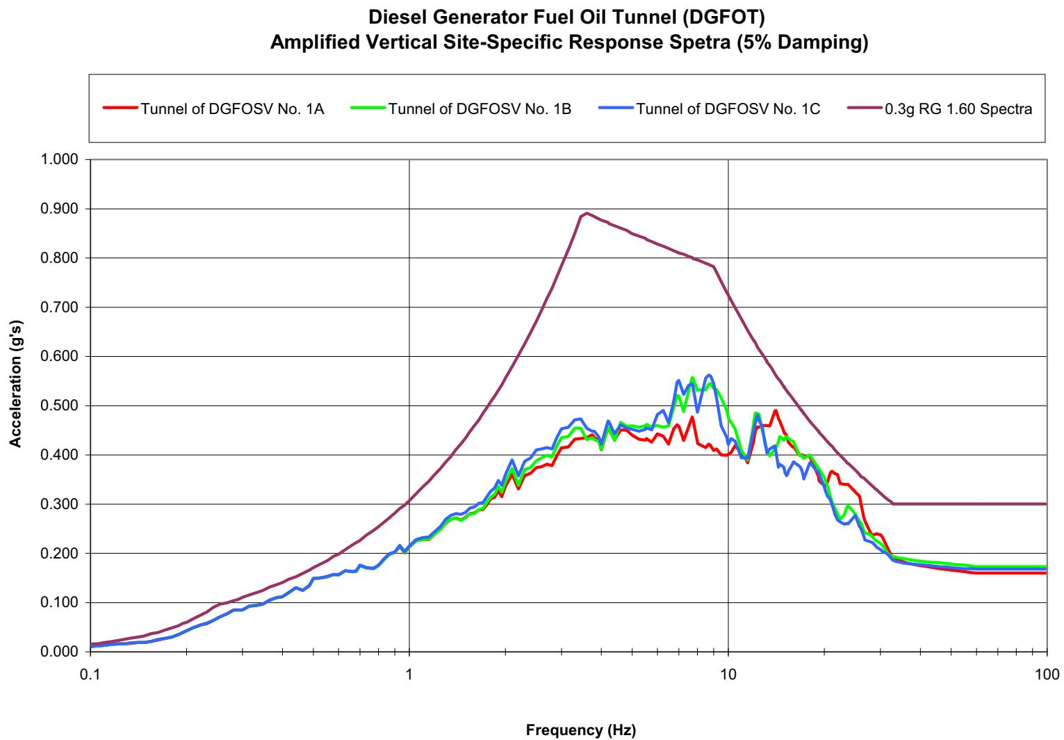
**Figure 3H.7-30c Amplified Vertical Site-Specific Response Spectra
