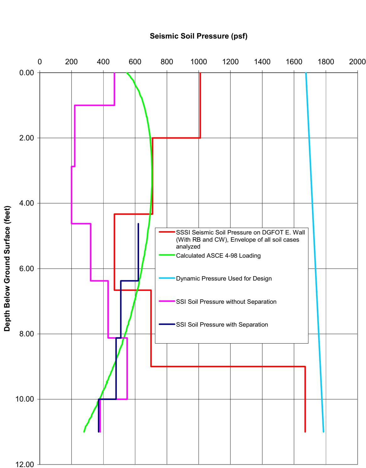
**Figure 3H.7-5 SSI, SSSI, ASCE 4-98 and Design Lateral Seismic Soil Pressures (psf) on Fuel Oil Tunnel East Wall with Reactor Building and Crane Wall**
