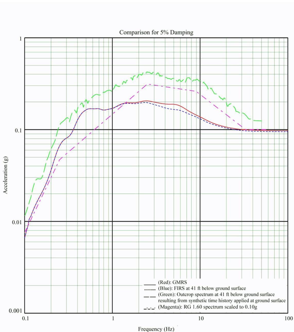
**Figure 3H.6-11d Comparison of Spectra at Foundation of Emergency Diesel Generator Fuel Storage Vault – Mean Soil Properties, E-W Direction**
