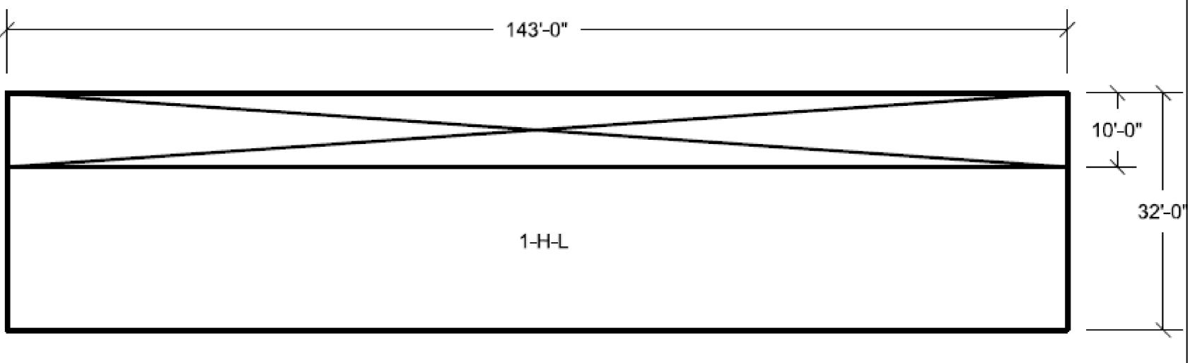
Figure 3H.6-63 Pump House South Wall Looking South Horizontal Reinforcement Zones Far Side Face
