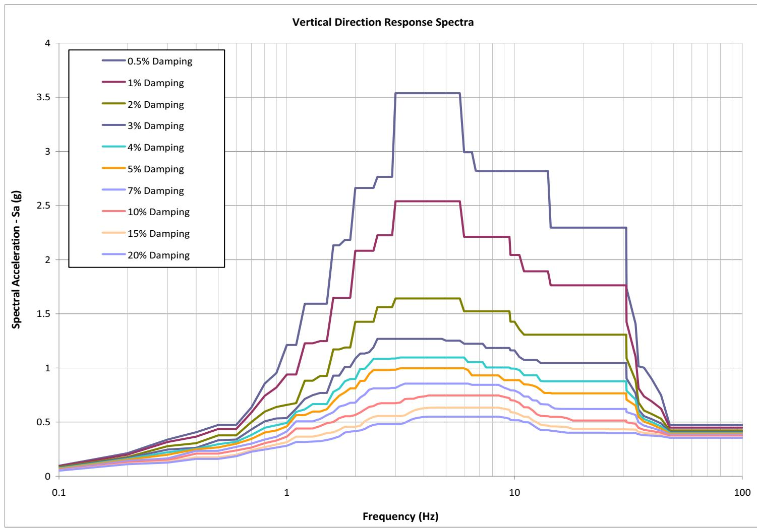
Figure 3H.7-32 Enveloped, Broadened **Horizontal****Vertical** Response Spectra for DGFTs
