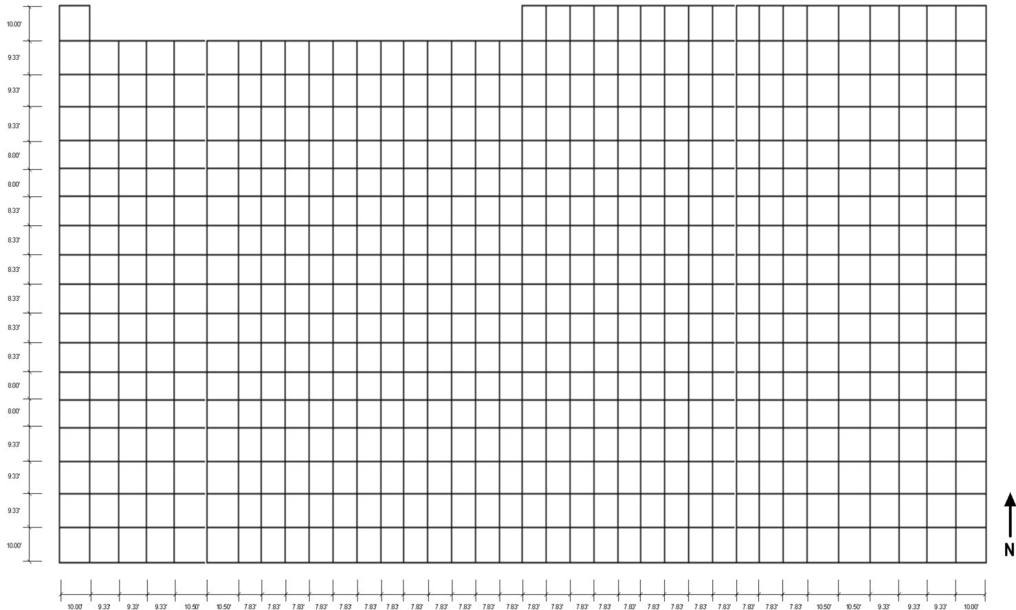
**Figure 3H.6-15f UHS Basin Basemat – SSI Model**
