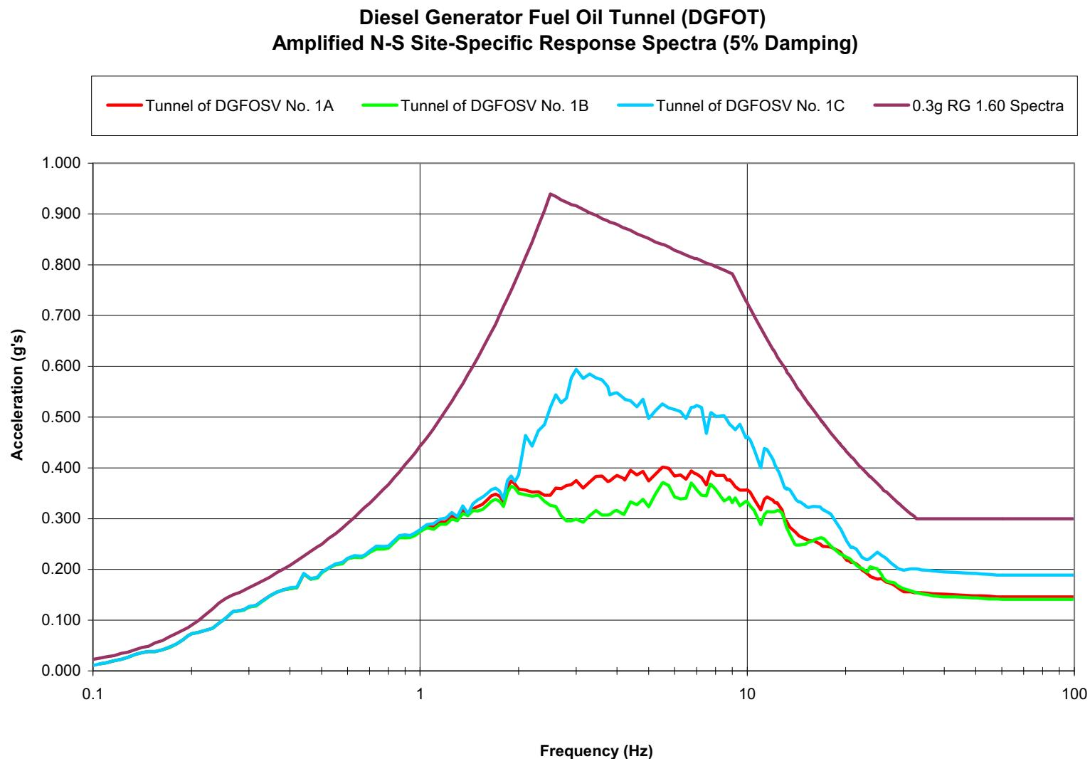
**Figure 3H.7-30a Amplified N-S Site-Specific Response Spectra
