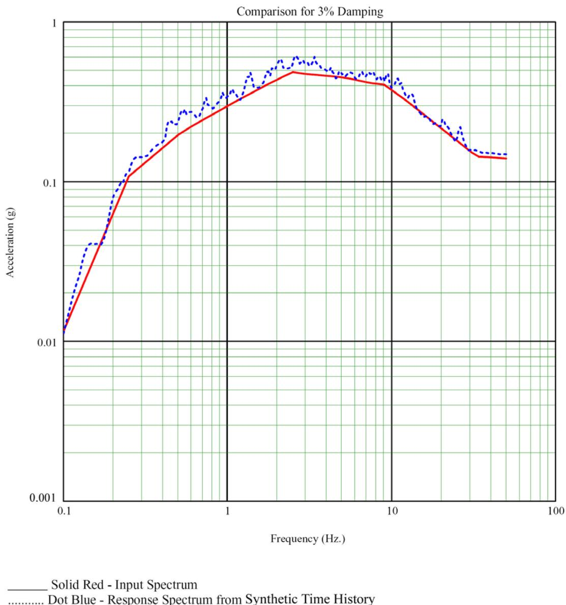
**Figure 3H.6-13b Comparison of Input Spectrum and Spectrum from Synthetic Time History, Horizontal (N-S) – 3% Damping**
