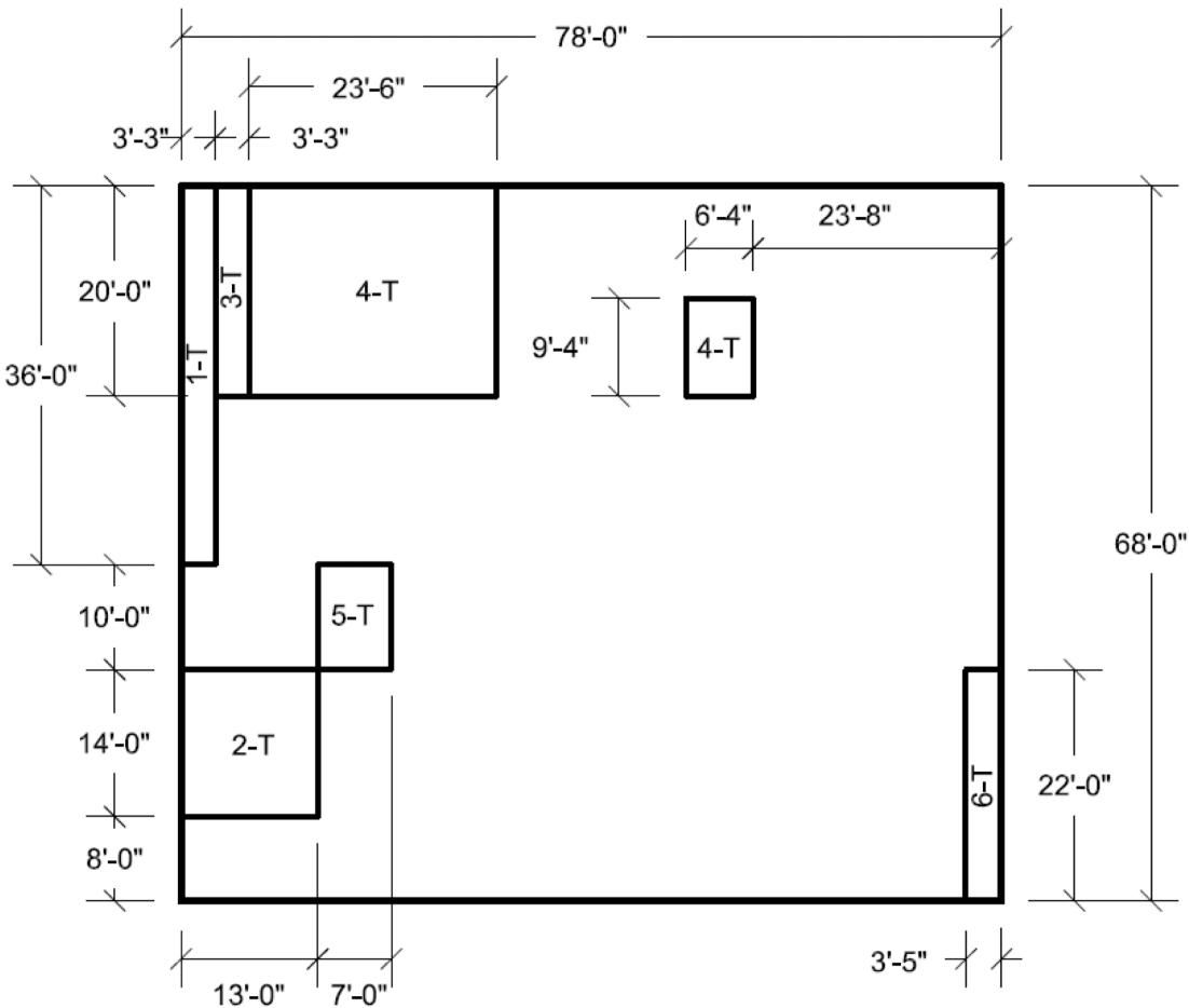
Figure 3H.6-60 Pump House East Wall Looking West **Vertical and Horizontal Transverse** Reinforcement Zones
