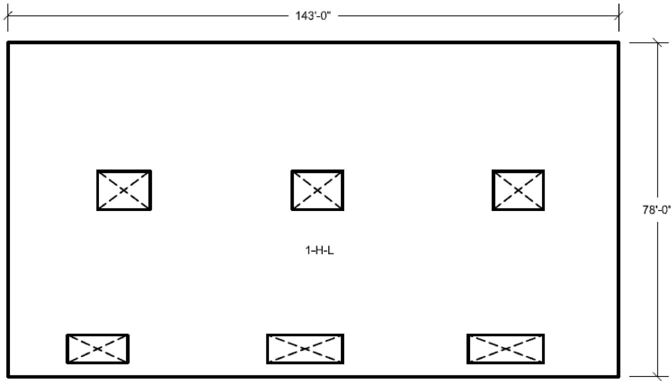
Figure 3H.6-127 Pump House Floor El 15'-2" East/ West Reinforcement Zones Top Face
