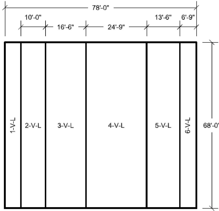
Figure 3H.6-59 Pump House East Wall Looking West Vertical Reinforcement Zones Far Side Face
