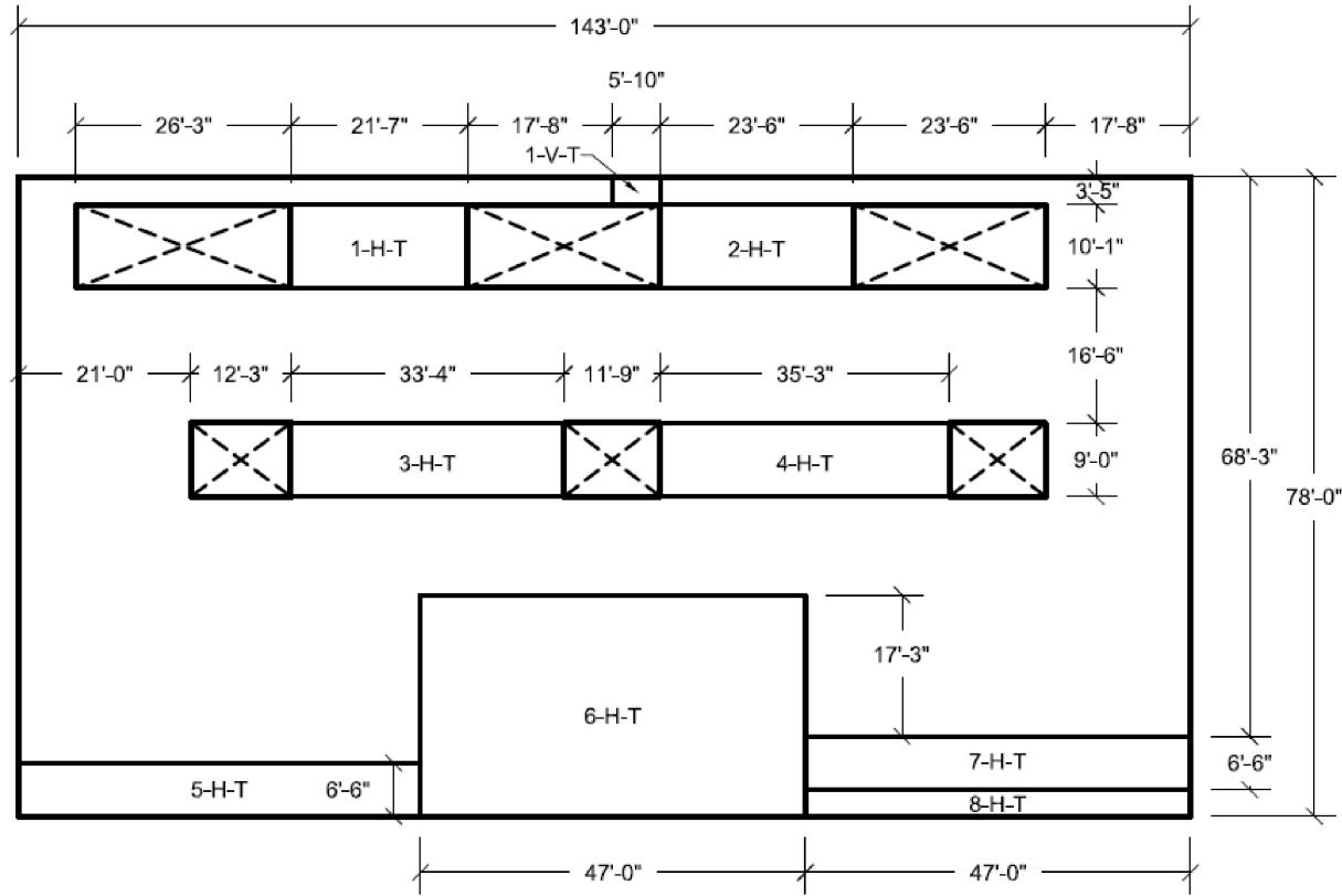
Figure 3H.6-136D Pump House Roof Transverse Vertical and Horizontal Reinforcement Zones
