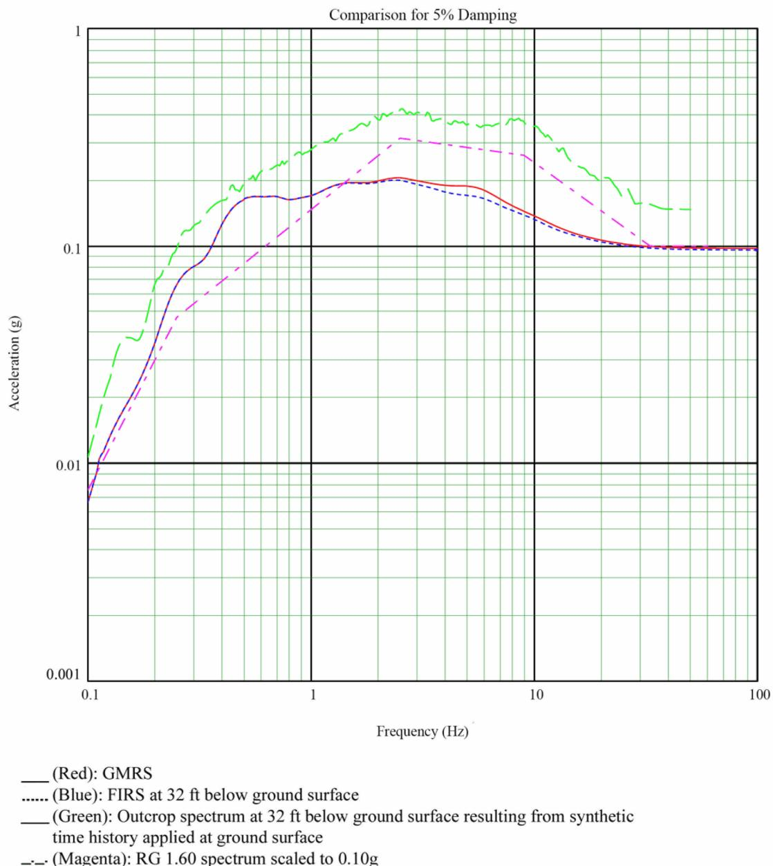
**Figure 3H.6-4c Comparison of Spectra at Foundation of UHS Basin (Lower Bound Soil Properties, N-S Direction)**
