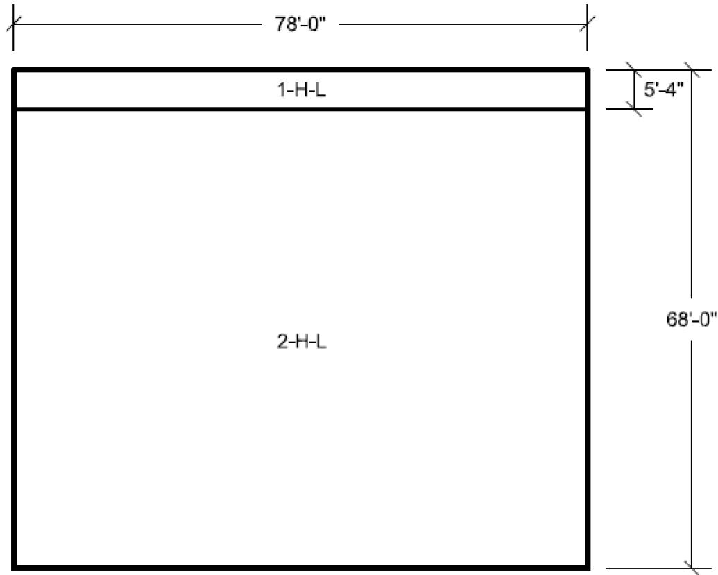
Figure 3H.6-77 Pump House Internal West Wall Looking West Horizontal Reinforcement Zones Far Side Face
