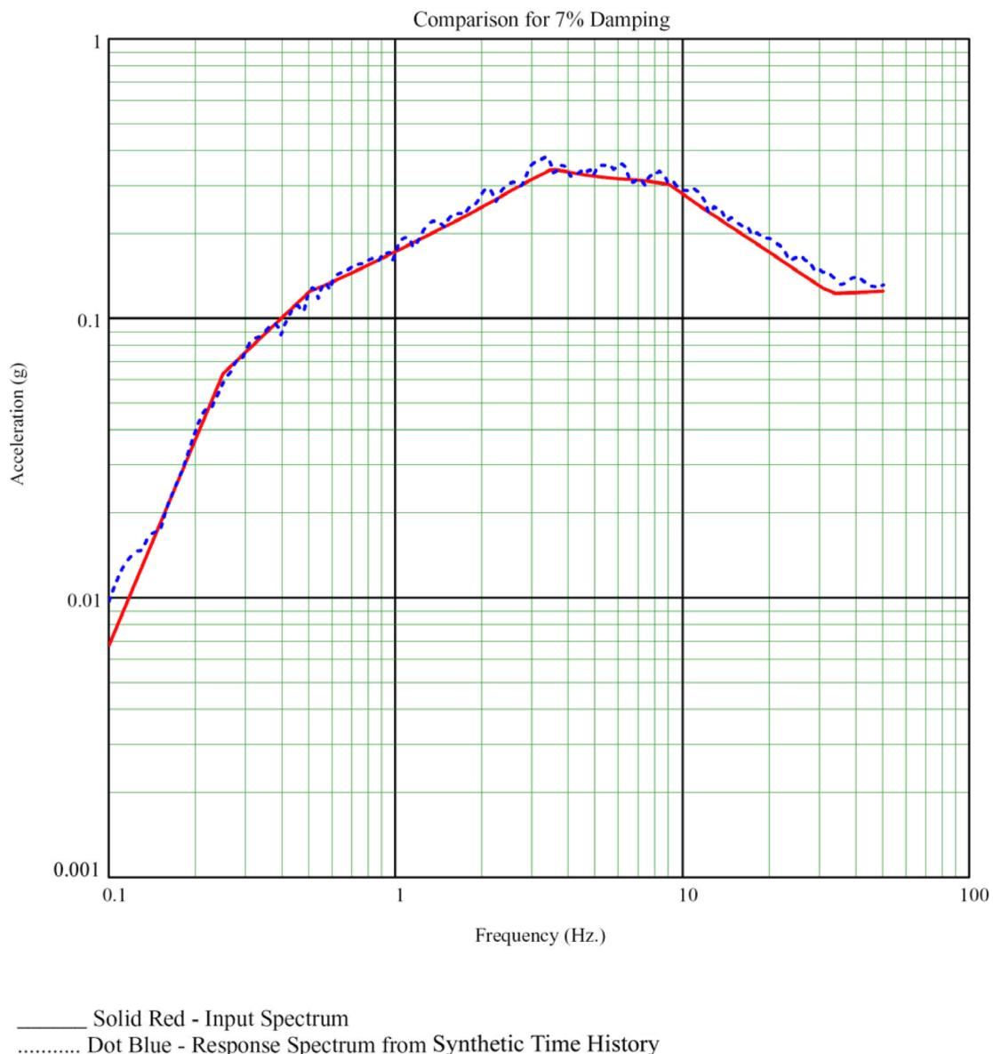
**Figure 3H.6-14d Comparison of Input Spectrum and Spectrum from Synthetic Time History, Vertical – 7% Damping**
