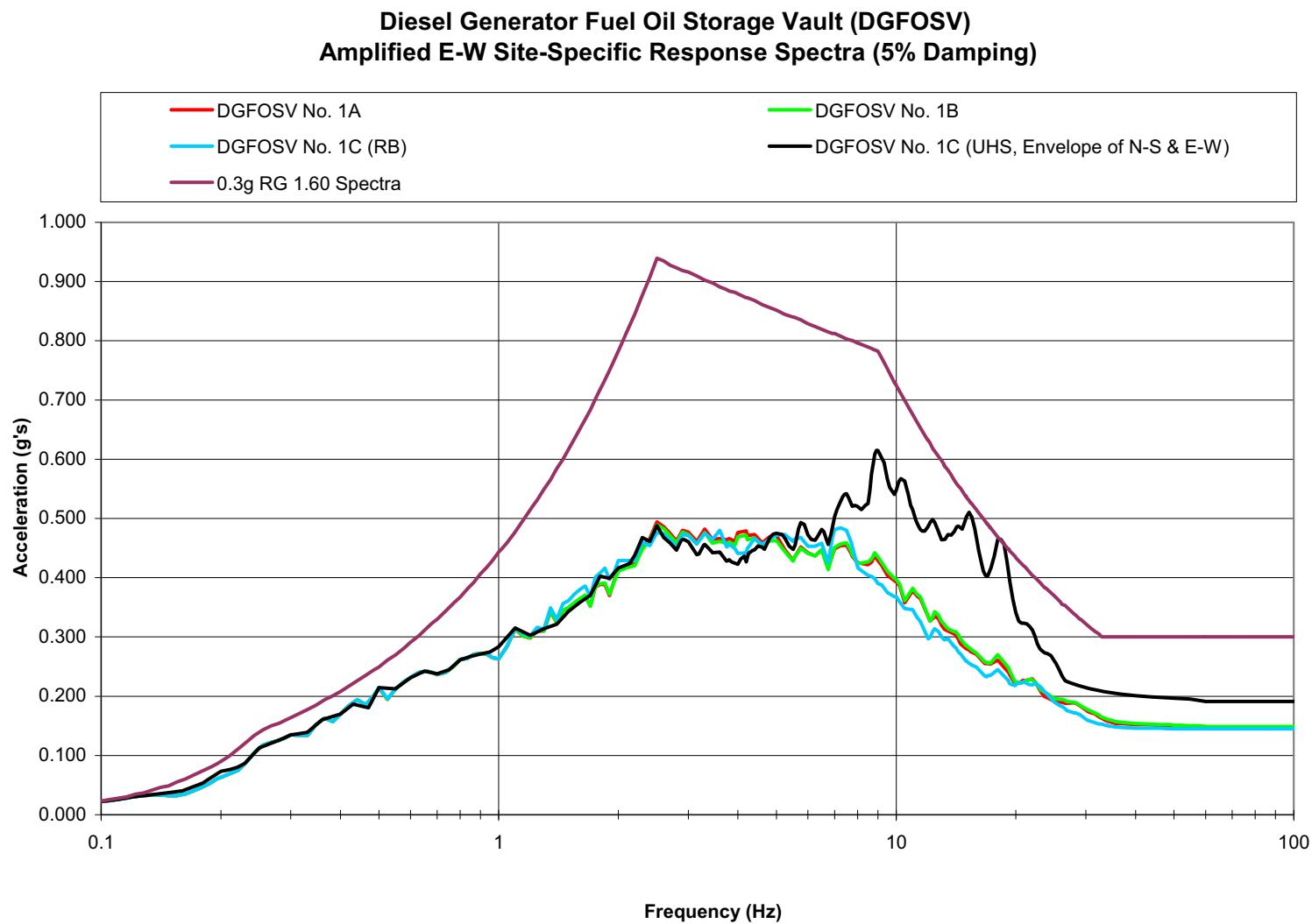
**Figure 3H.6-222b Amplified E-W Site-Specific Response Spectra
