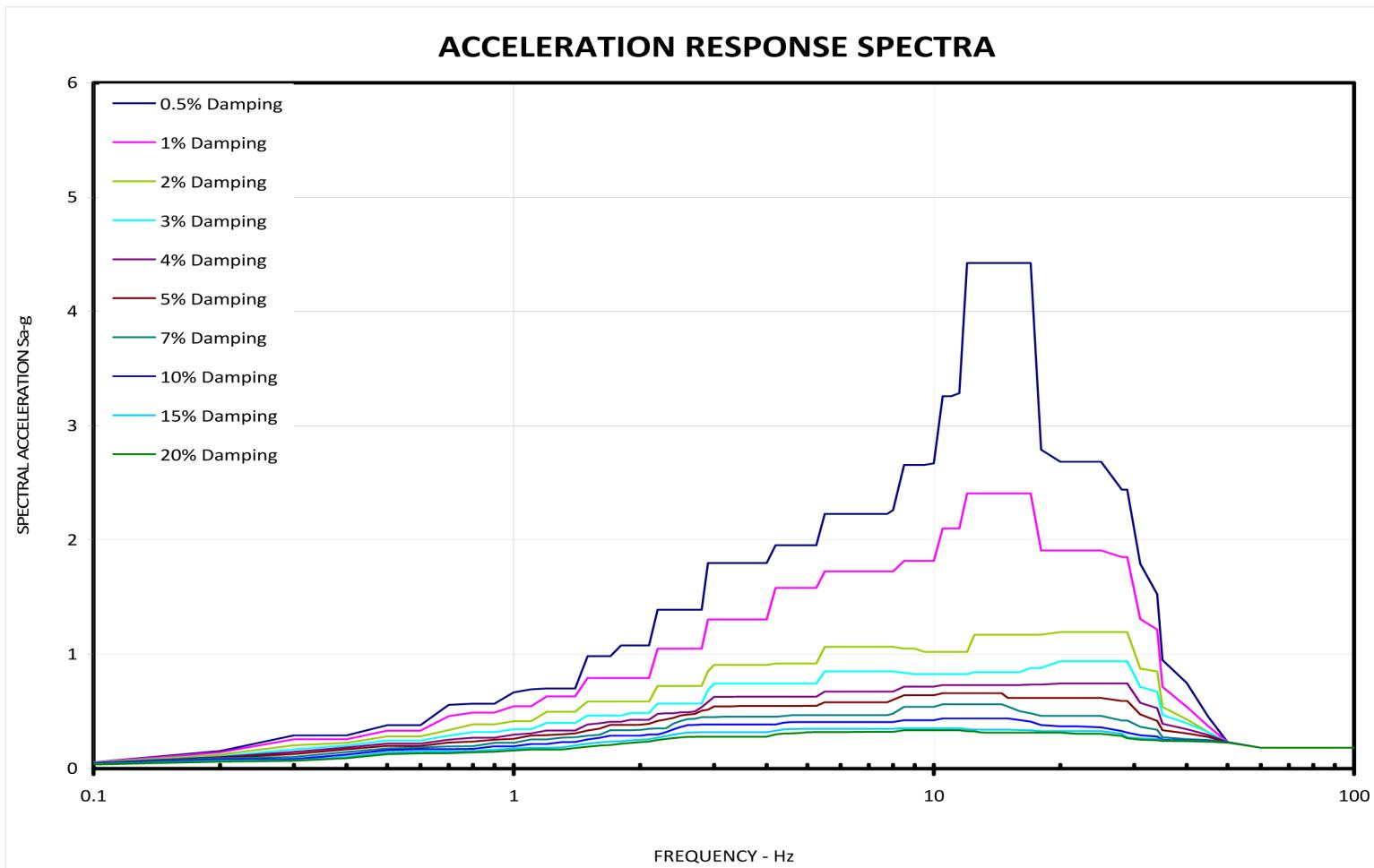
Figure 3H.6-139 RSW Piping Tunnel, Vertical Response Spectra
