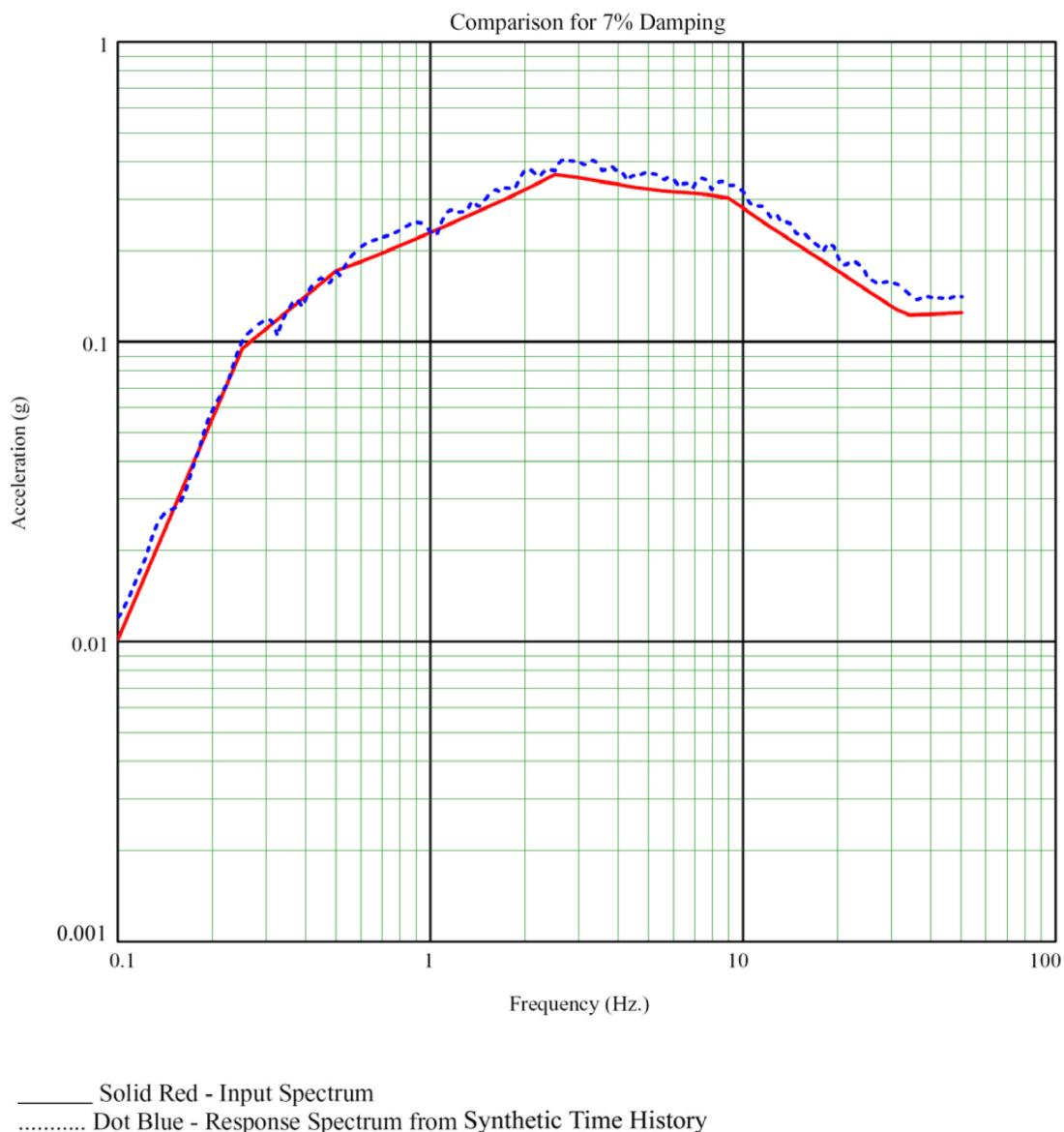
**Figure 3H.6-12d Comparison of Input Spectrum and Spectrum from Synthetic Time History, Horizontal (E-W) – 7% Damping**
