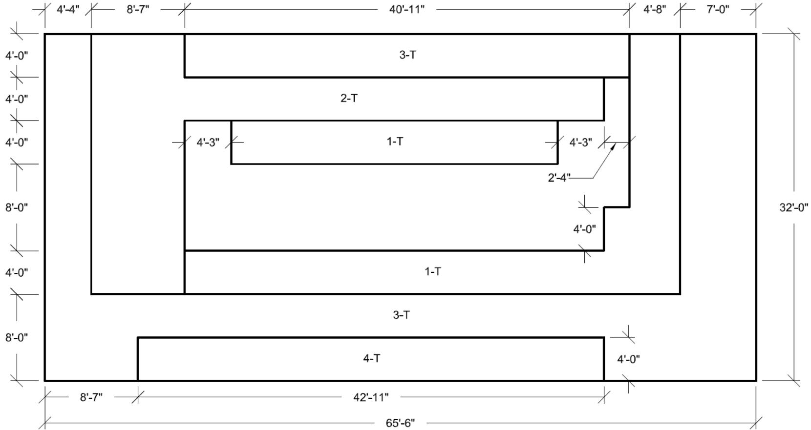
Figure 3H.6-167 Wall 7 Looking From Outside Transverse Reinforcement Zones
