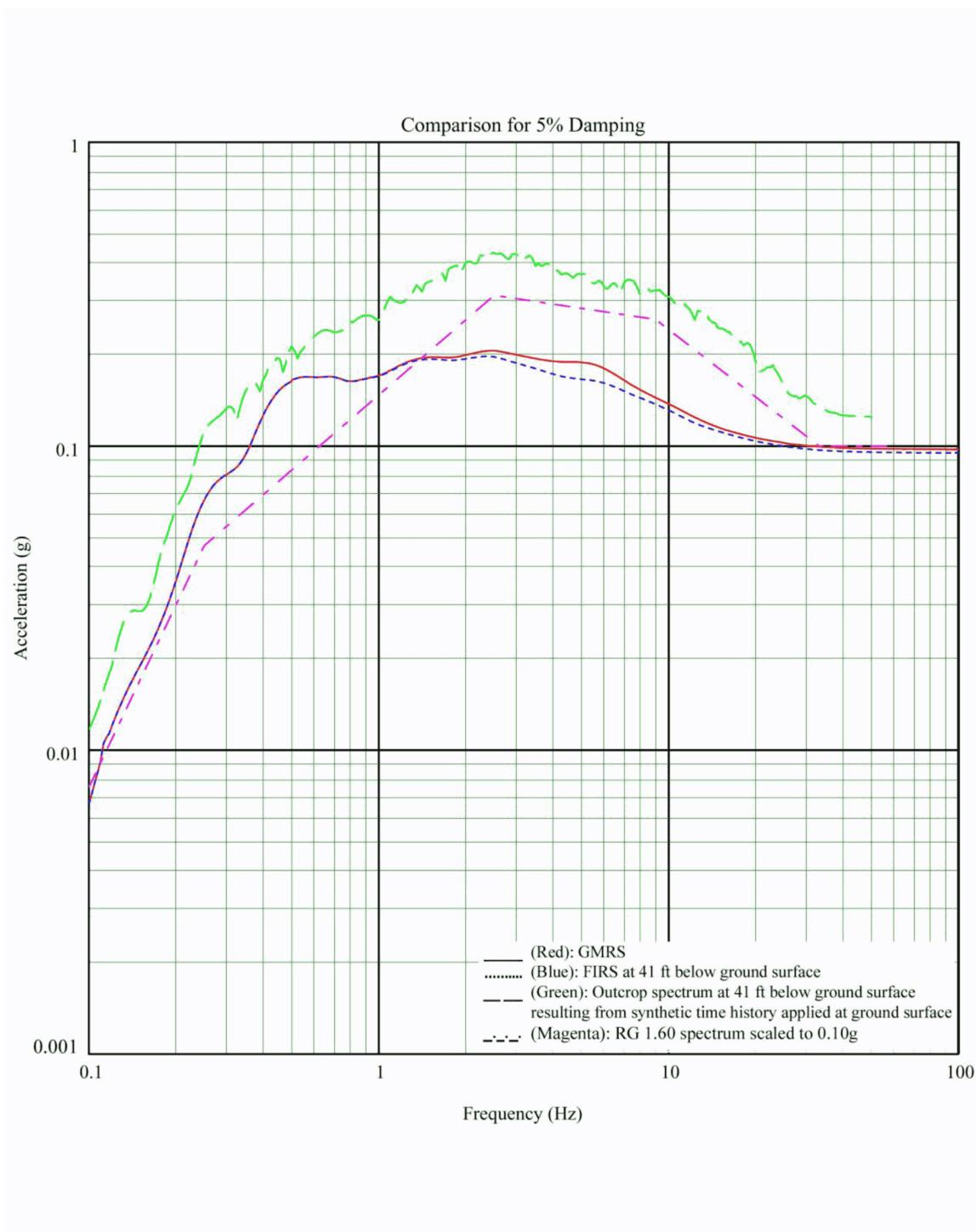
**Figure 3H.6-11e Comparison of Spectra at Foundation of Emergency Diesel Generator Fuel Storage Vault – Upper Bound Soil Properties, E-W Direction**
