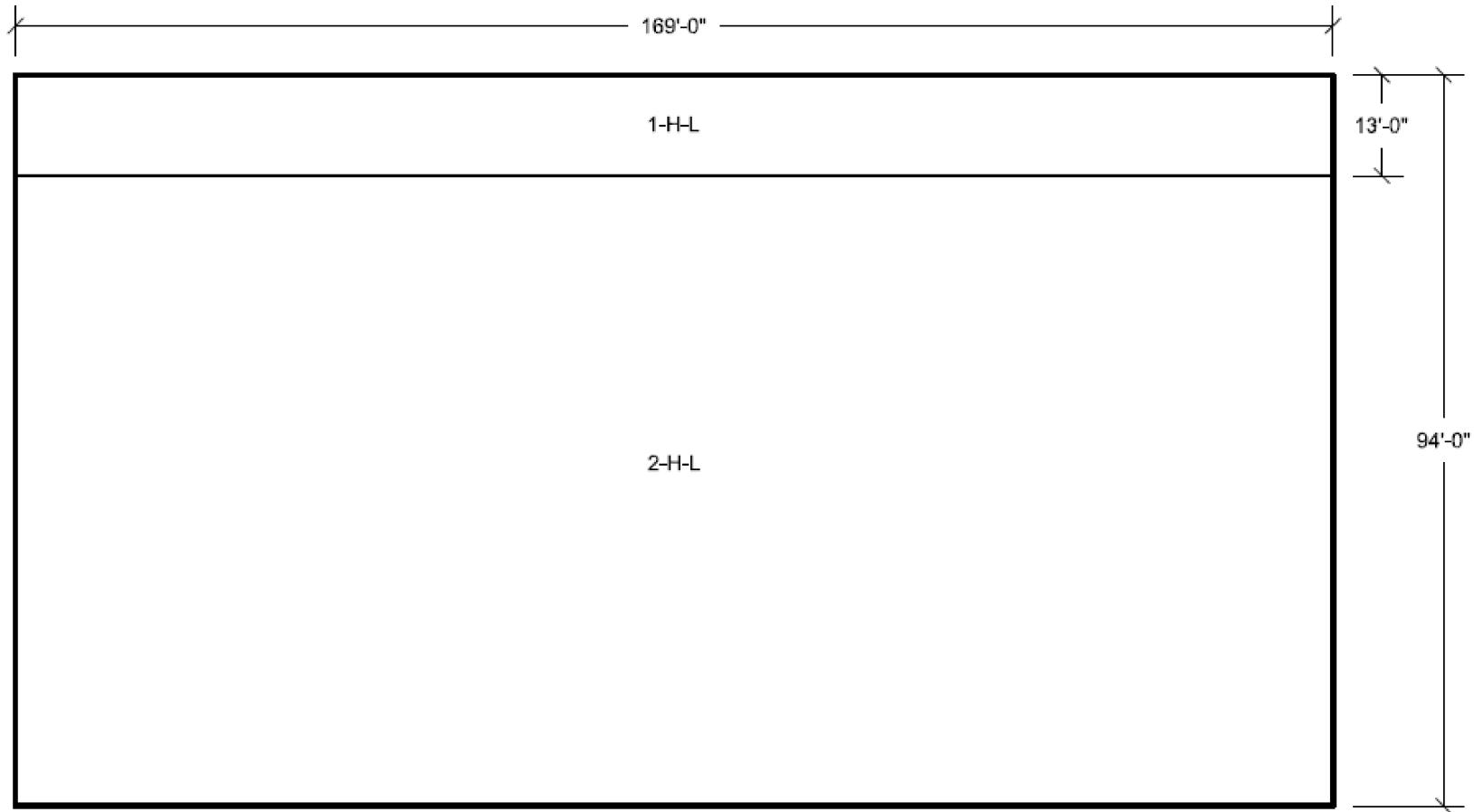
Figure 3H.6-123 Pump House Foundation Mat East/West Reinforcement Zones Top Face
