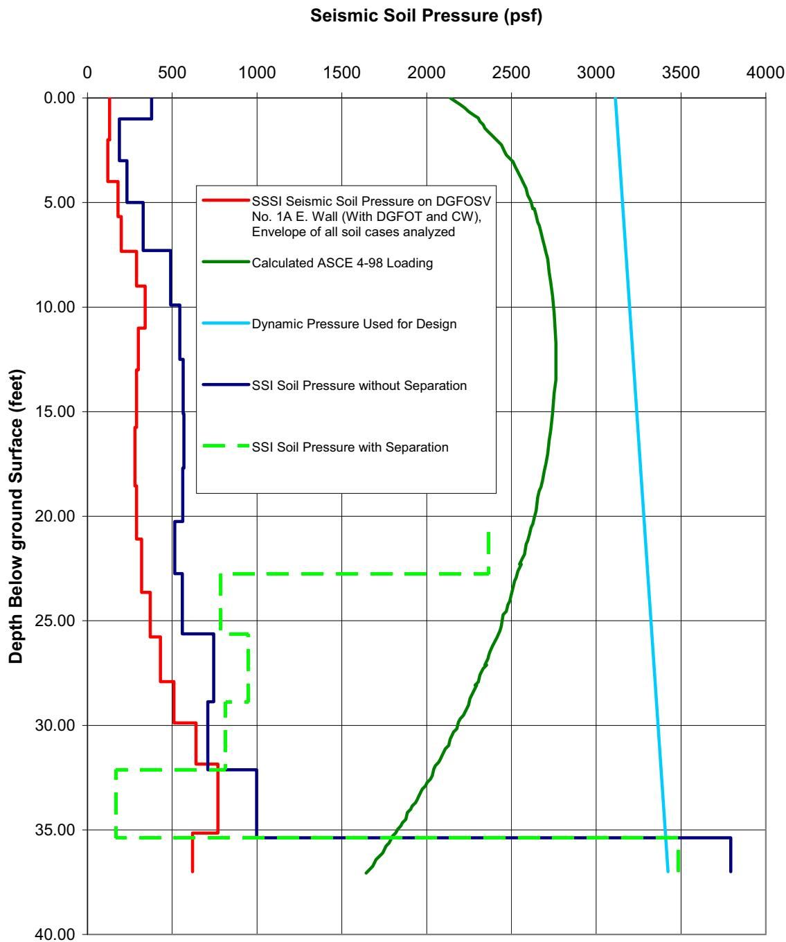
**Figure 3H.6-230 SSI, SSSI, ASCE 4-98 and Design Lateral Seismic Soil Pressures on Diesel Generator Fuel Oil Storage Vault No. 1A East Wall**
