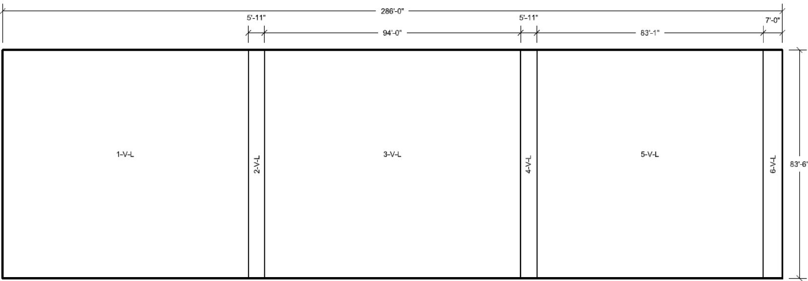
Figure 3H.6-88 UHS Basin South Wall Looking North Vertical Reinforcement Zones Near Side Face
