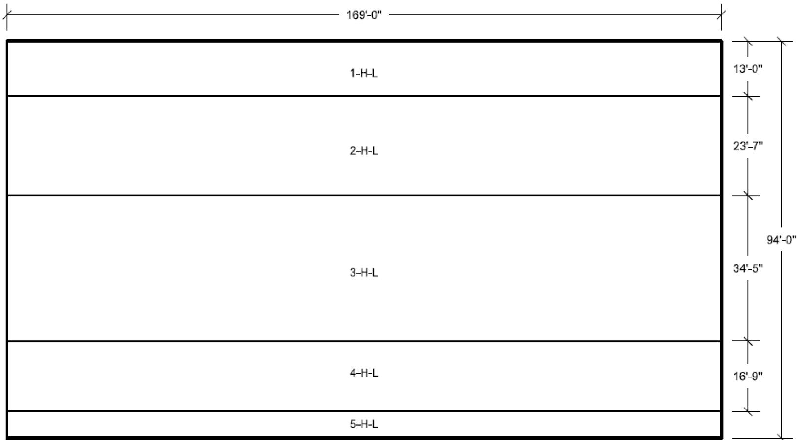
Figure 3H.6-125 Pump House Foundation Mat East/West Reinforcement Zones Bottom Face
