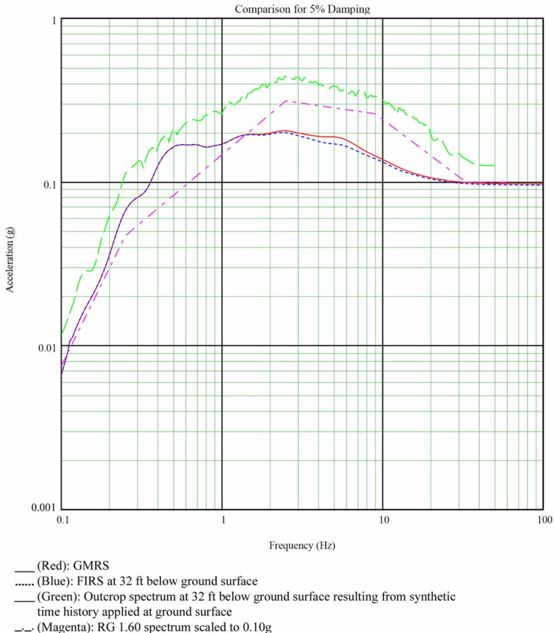
**Figure 3H.6-3b Comparison of Spectra at Foundation of UHS Basin (Upper Bound Soil Properties, E-W Direction)**
