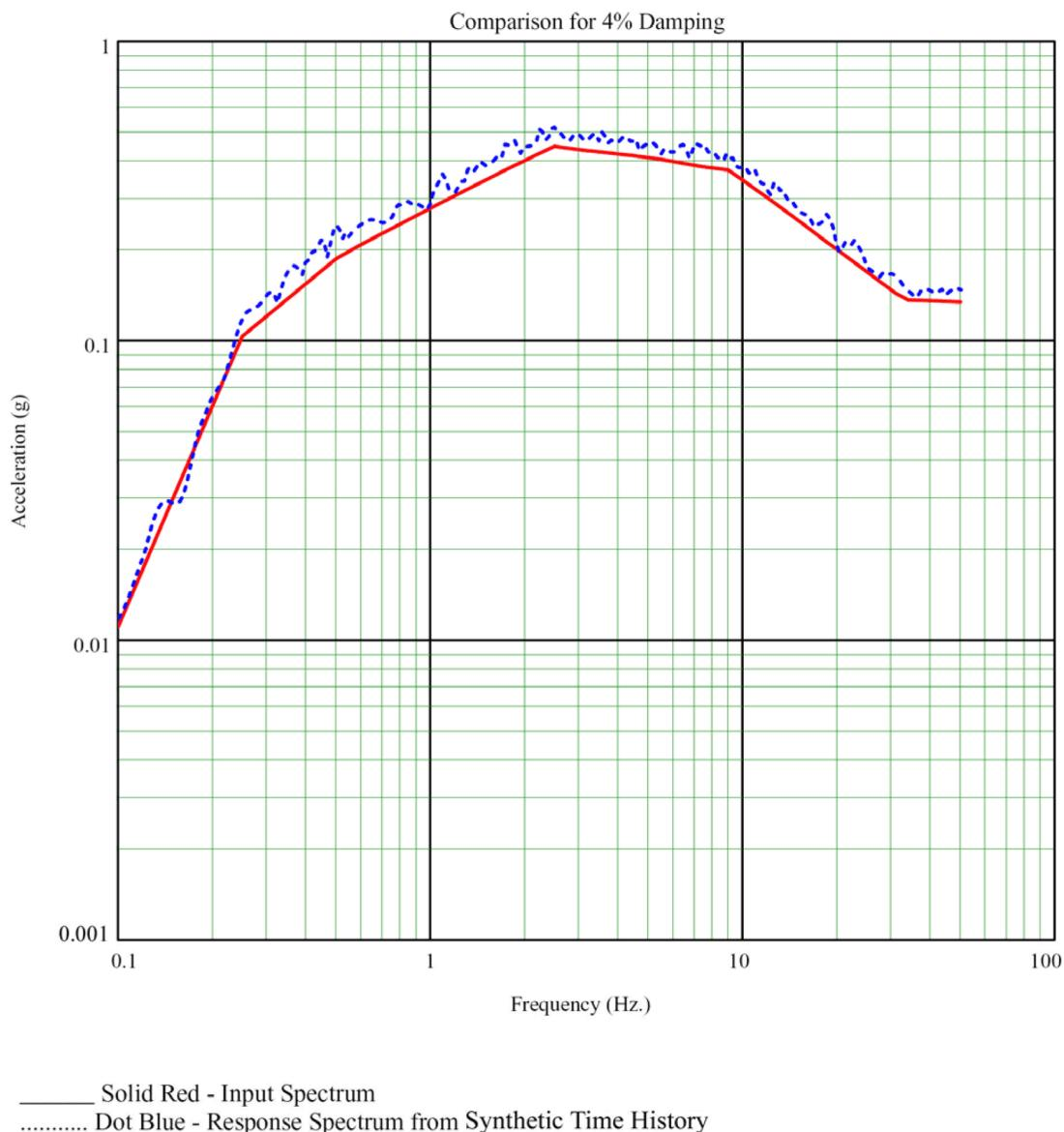
**Figure 3H.6-12c Comparison of Input Spectrum and Spectrum from Synthetic Time History, Horizontal (E-W) – 4% Damping**
