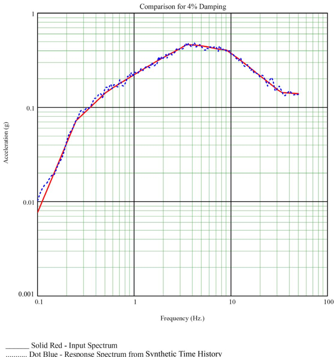
**Figure 3H.6-14c Comparison of Input Spectrum and Spectrum from Synthetic Time History, Vertical – 4% Damping**
