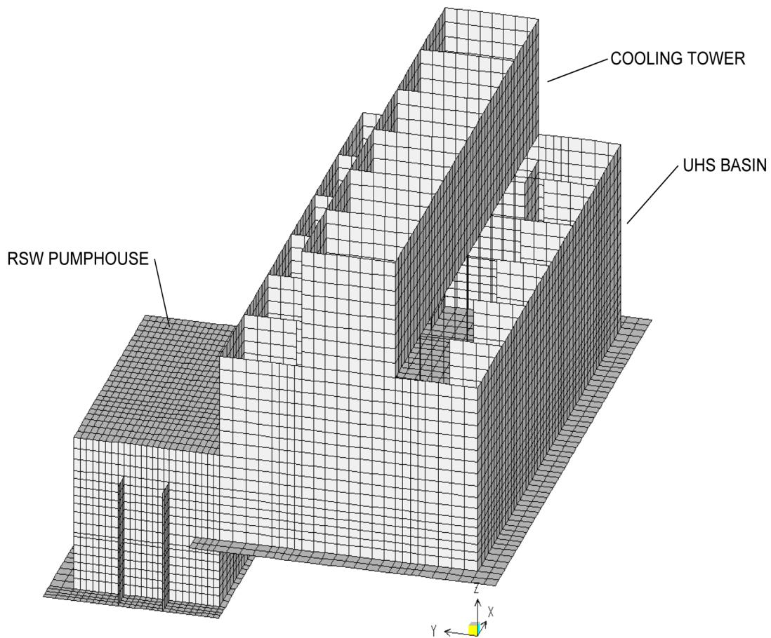
**Figure 3H.6-40 SAP Finite Element Model for UHS and RSW Pump House Design**
