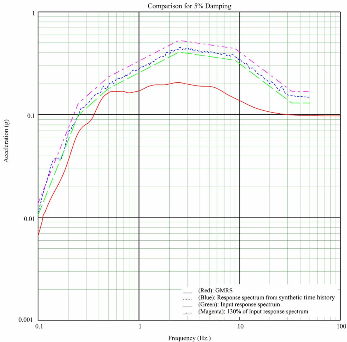
**Figure 3H.6-13 Comparison of Spectrum from Synthetic Time History, Input Spectrum, 130% of Input Spectrum, and GMRS (N-S Direction)**
