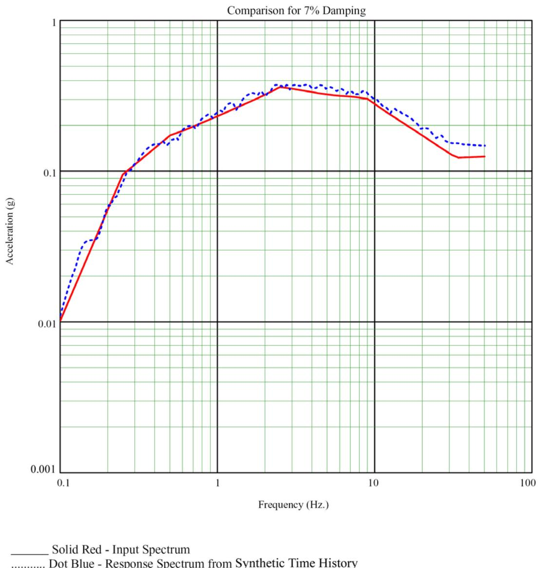
**Figure 3H.6-13d Comparison of Input Spectrum and Spectrum from Synthetic Time History, Horizontal (N-S) – 7% Damping**
