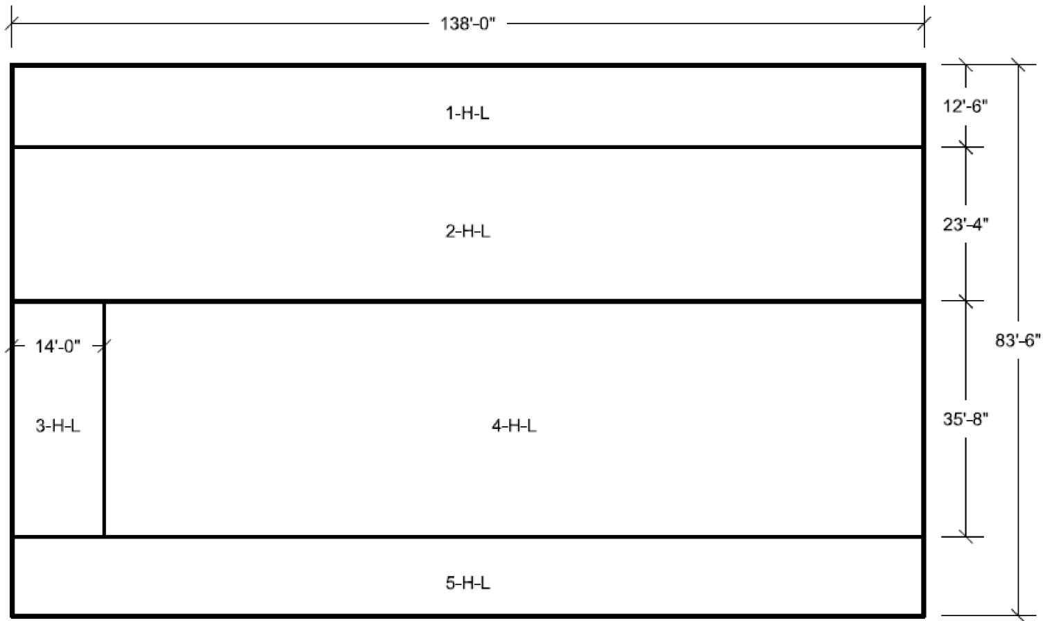
Figure 3H.6-99 UHS Basin West Wall Looking East Horizontal Reinforcement Zones Far Side Face
