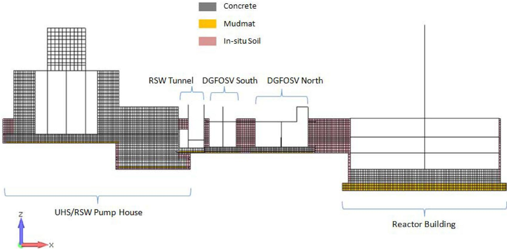
Figure 3H.6-211 2D Model of UHS/RSW Pump House, RSW Piping Tunnel, DGFOSVs and RB
