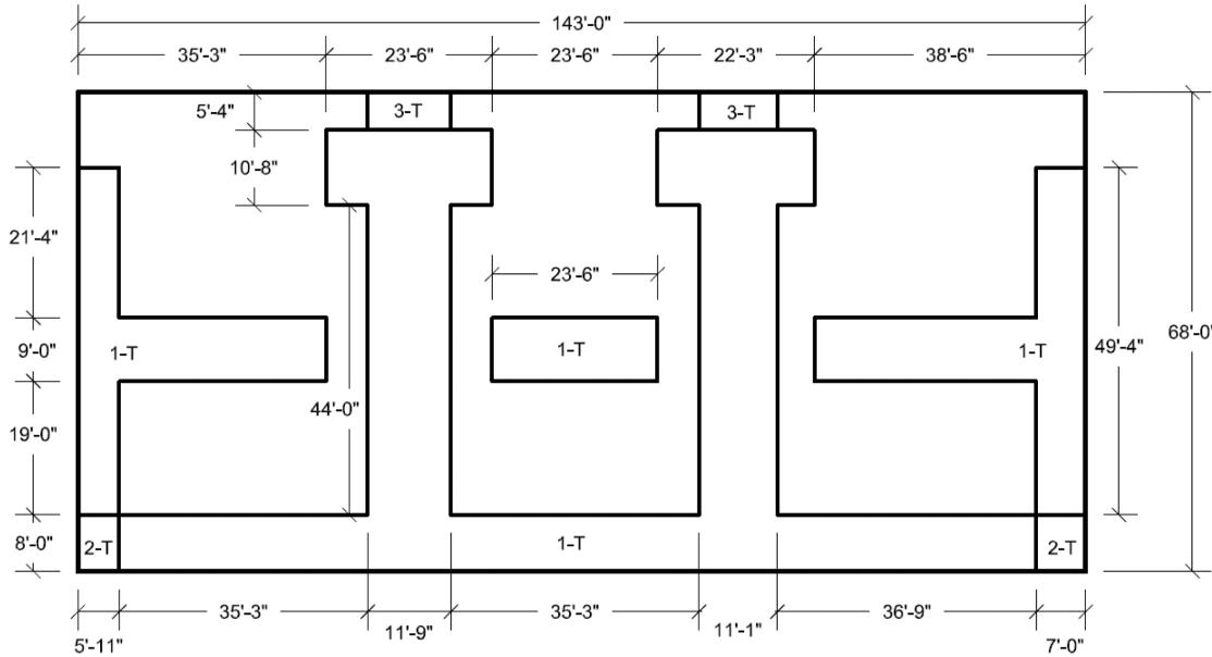
Figure 3H.6-55 Pump House North Wall Looking South Transverse **Horizontal** Reinforcement Zones
