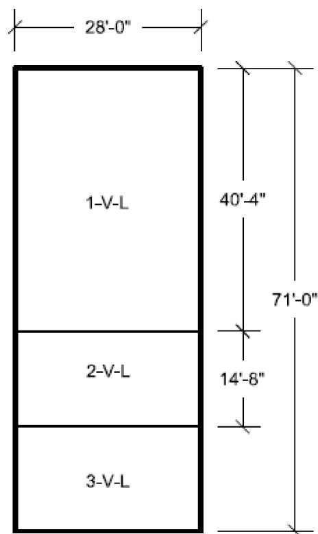
**Figure 3H.6-106 UHS Basin East Buttress Looking North & UHS Basin West Buttress Looking South Vertical Reinforcement Zones Near and Far Side Faces**
