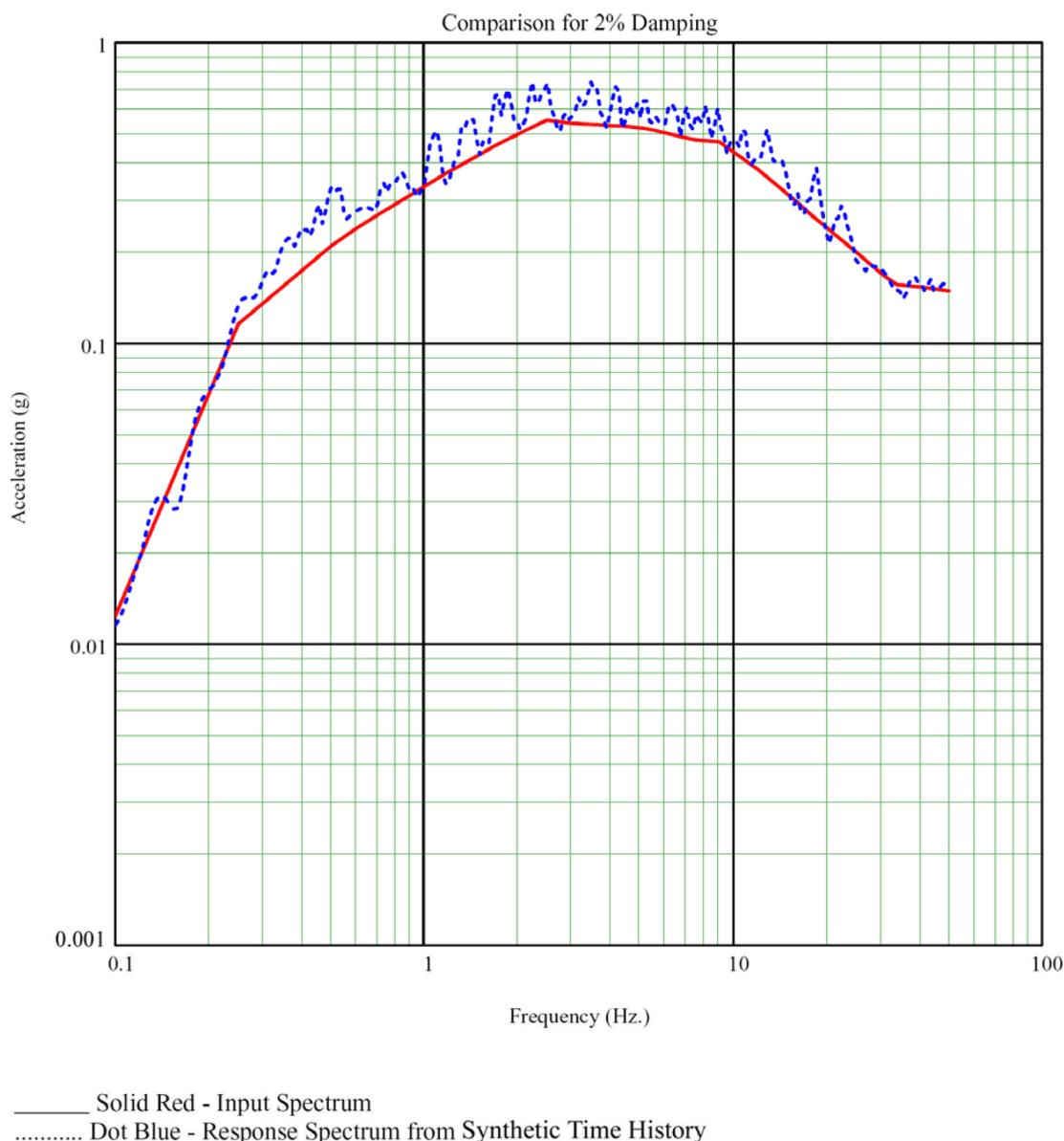
**Figure 3H.6-12a Comparison of Input Spectrum and Spectrum from Synthetic Time History, Horizontal (E-W) – 2% Damping**
