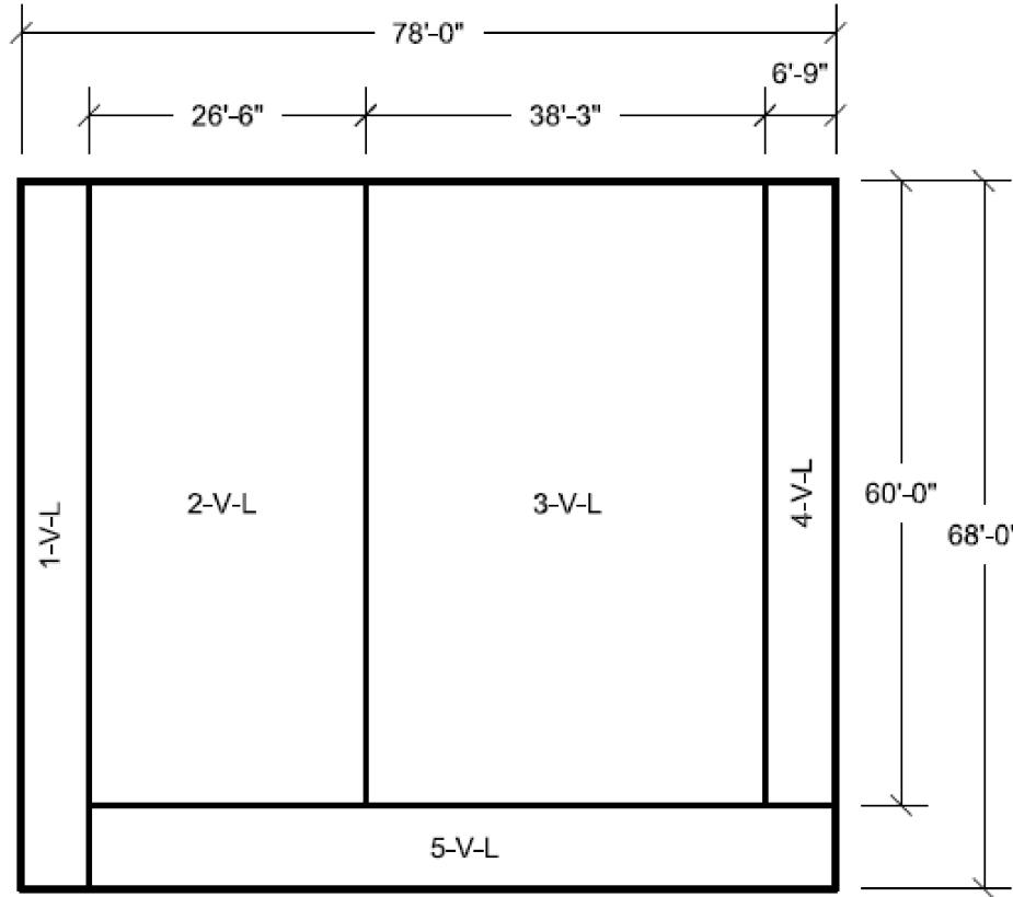
**Figure 3H.6-57 Pump House East Wall Looking West Vertical Reinforcement Zones Near Side Face**
