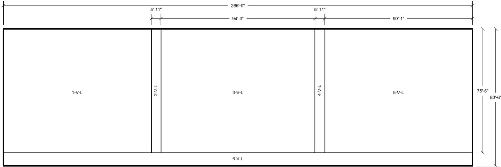
**Figure 3H.6-90 UHS Basin South Wall Looking North Vertical Reinforcement Zones Far Side Face**
