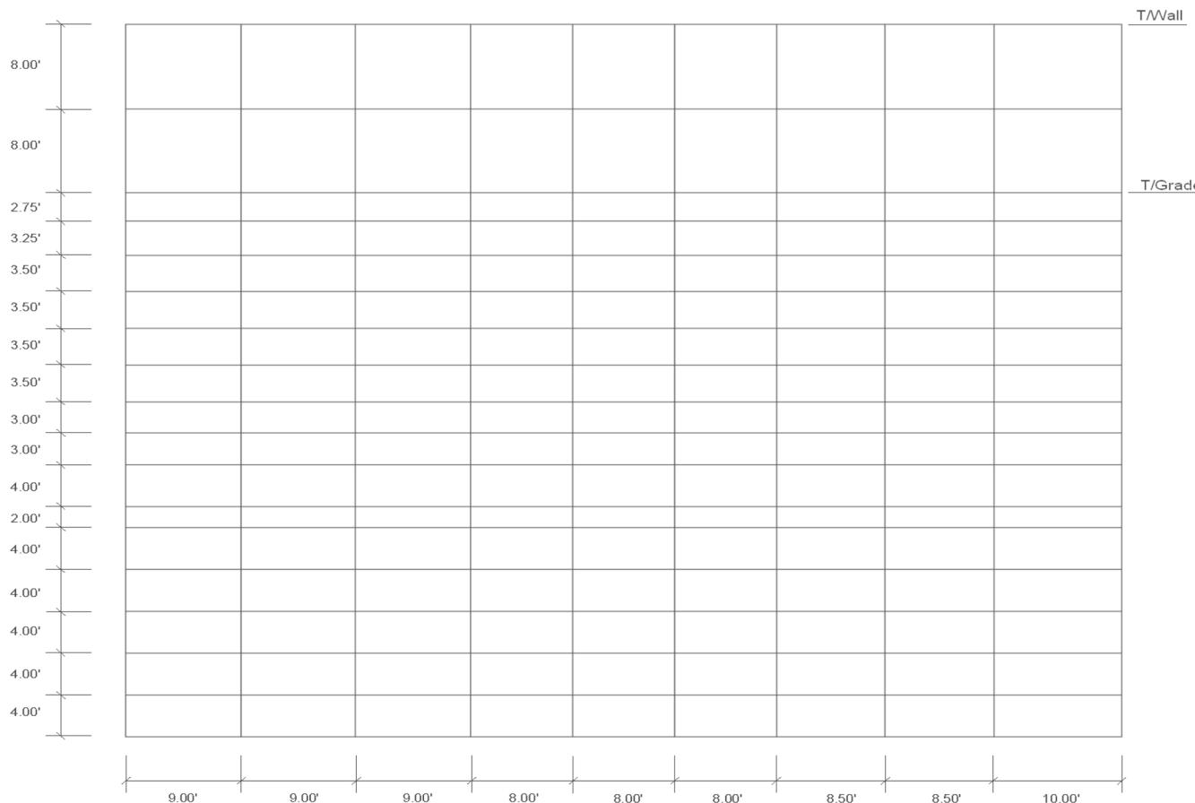
Note: The view above is looking east at the outside face of the RSW pump house west wall. The RSW pump house east wall mesh is the mirror image of the RSW pump house west wall mesh with the same dimensions.
