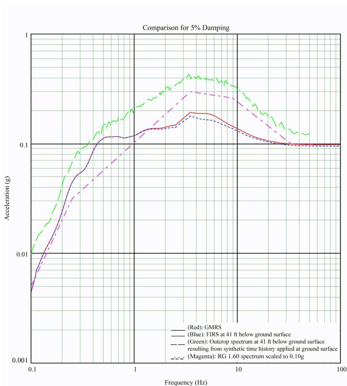
**Figure 3H.6-11j Comparison of Spectra at Foundation of Emergency Diesel Generator Fuel Storage Vault – Mean Soil Properties, Vertical Direction**
