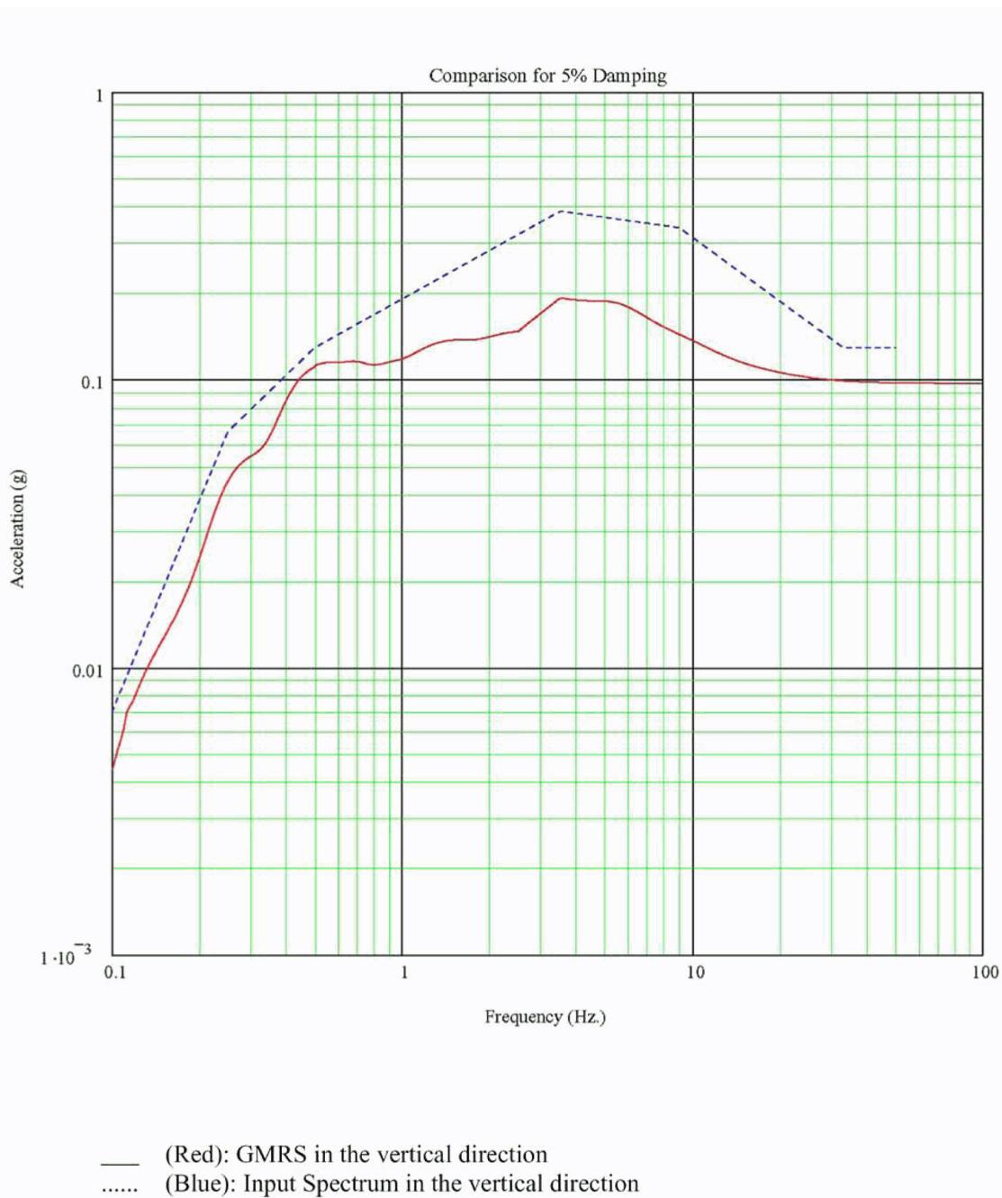
**Figure 3H.6-2 Comparison of GMRS with the Input Spectrum (Vertical)**
