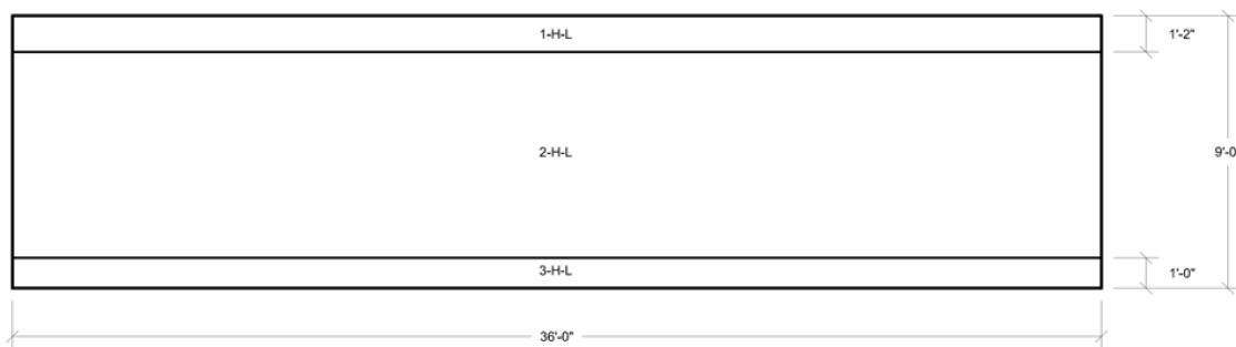
**Figure 3H.7-11 Tunnel Walls Looking From Outside Horizontal Reinforcement Zones Near Side Face**
