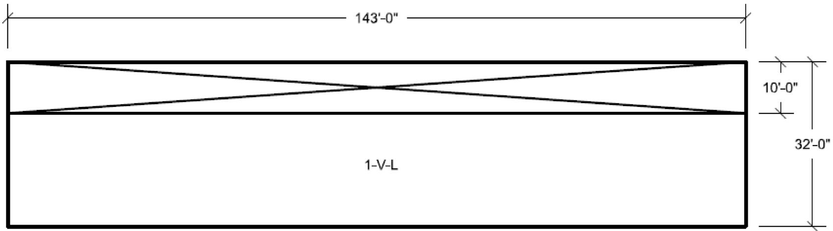
Figure 3H.6-64 Pump House South Wall Looking South Vertical Reinforcement Zones Far Side Face
