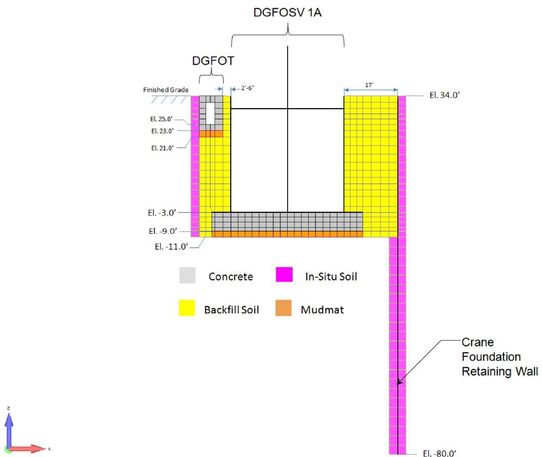
**Figure 3H.6-225 2D SSSI Model of DGFOT, DGFSV and Crane Foundation Retaining Wall**
