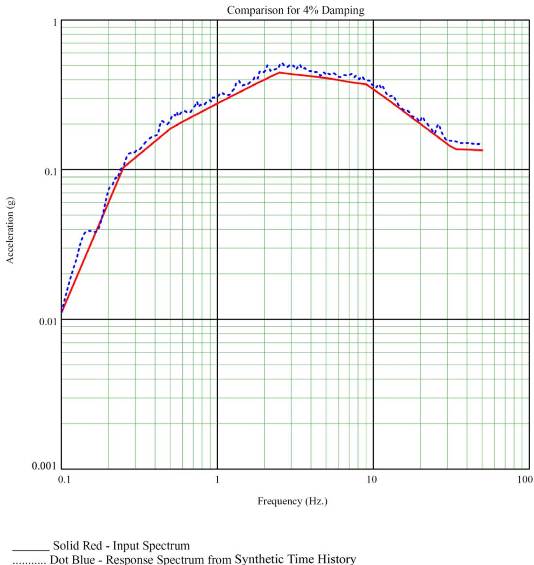
**Figure 3H.6-13c Comparison of Input Spectrum and Spectrum from Synthetic Time History, Horizontal (N-S) – 4% Damping**
