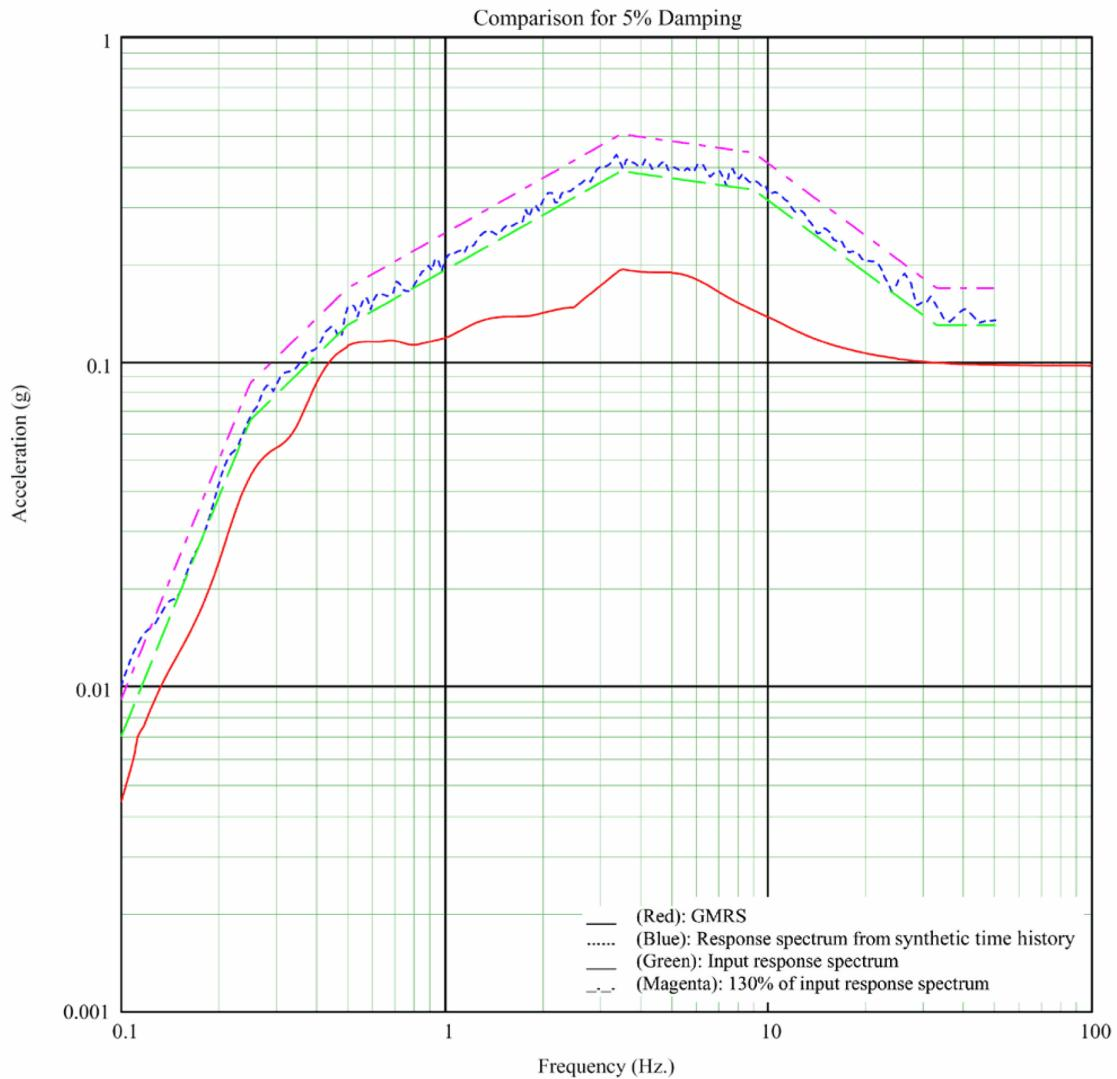
**Figure 3H.6-14 Comparison of Spectrum from Artificial Time History, Input Spectrum, 130% of Input Spectrum, and GMRS (Vertical Direction)**
