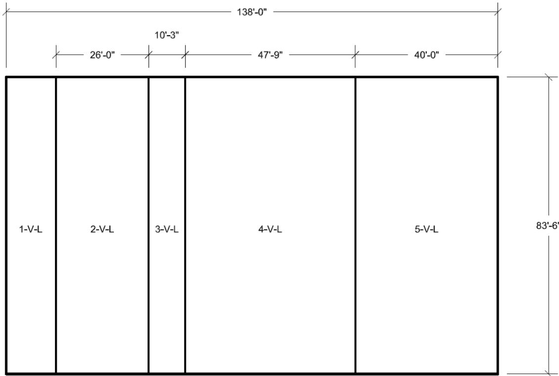
Figure 3H.6-98 UHS Basin West Wall Looking East Vertical Reinforcement Zones Near Side Face
