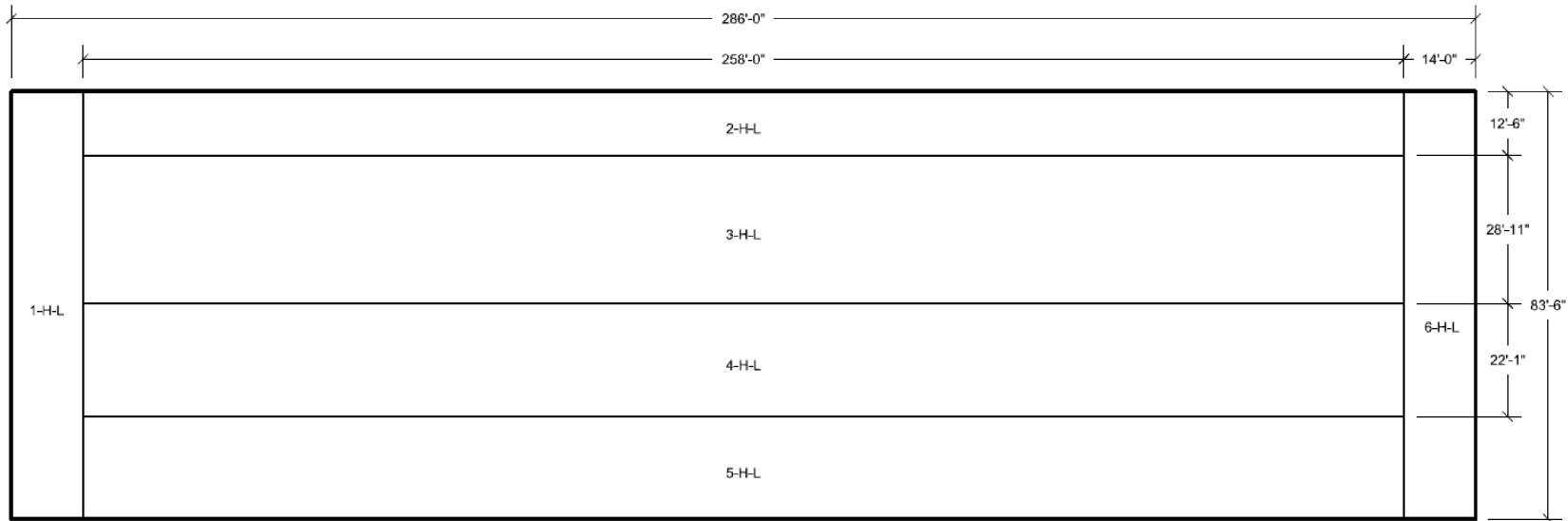
Figure 3H.6-89 UHS Basin South Wall Looking North Horizontal Reinforcement Zones Far Side Face
