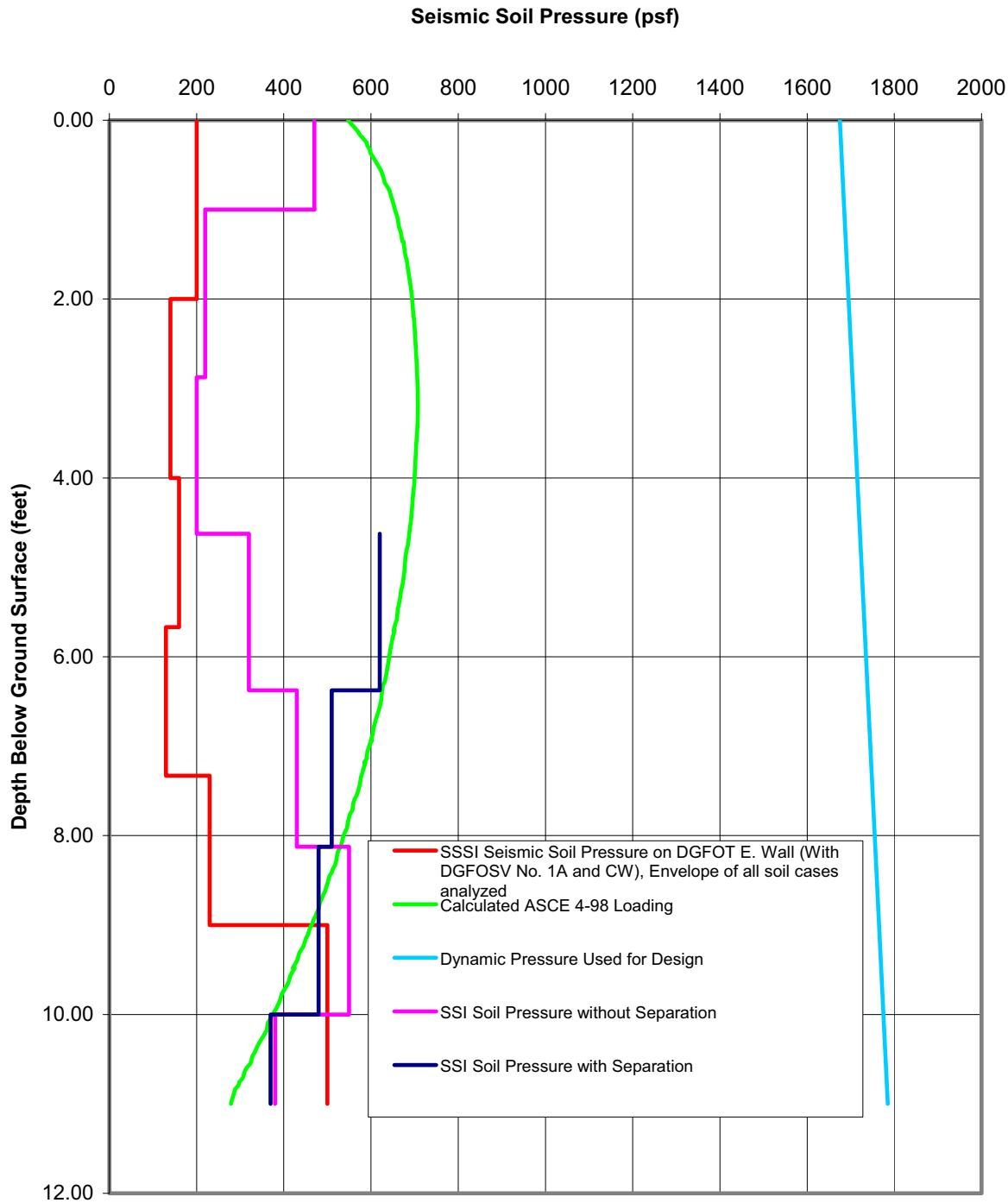
**Figure 3H.7-7 SSI, SSS, ASCE 4-98 and Design Lateral Seismic Soil Pressures (psf) on Fuel Oil Tunnel East Wall with Diesel Generator Fuel Oil Storage Vault and Crane Wall**
