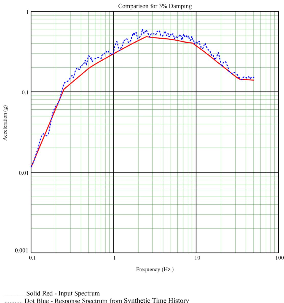
**Figure 3H.6-12b Comparison of Input Spectrum and Spectrum from Synthetic Time History, Horizontal (E-W) – 3% Damping**
