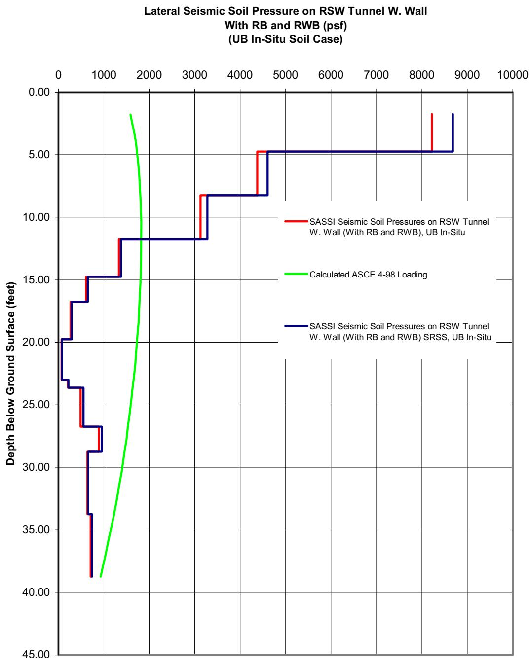
**Figure 3H.6-217 Lateral Seismic Soil Pressures (psf) on RSW Piping Tunnel West Wall For UB In-Situ Soil Case (Main Cross Section of RSW Piping Tunnel, Including Effect of Vertical Excitation)**
