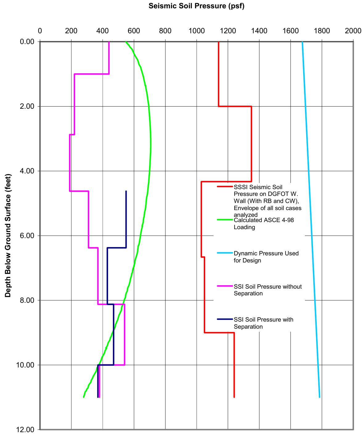
**Figure 3H.7-6 SSI, SSS, ASCE 4-98 and Design Lateral Seismic Soil Pressures (psf) on Fuel Oil Tunnel West Wall with Reactor Building and Crane Wall**
