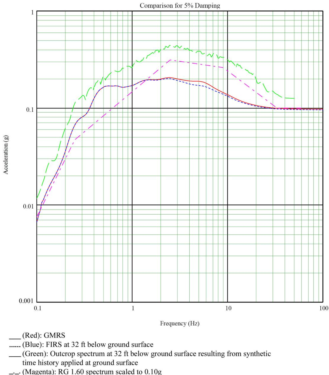
**Figure 3H.6-3c Comparison of Spectra at Foundation of UHS Basin (Lower Bound Soil Properties, E-W Direction)**
