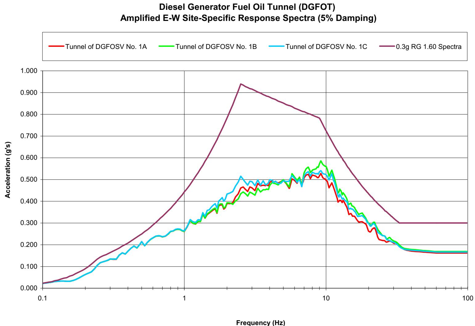
**Figure 3H.7-30b Amplified E-W Site-Specific Response Spectra
