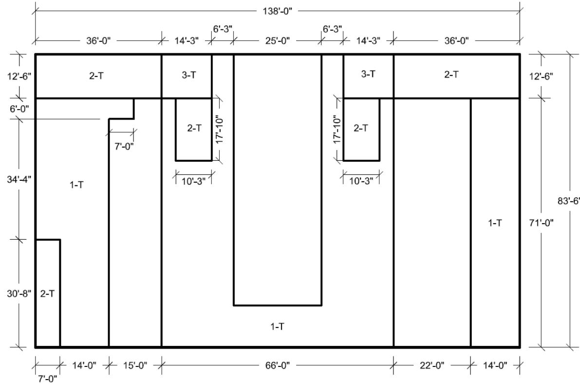
Figure 3H.6-96 UHS Basin East Wall Looking West Transverse **Horizontal and Vertical** Reinforcement Zones
