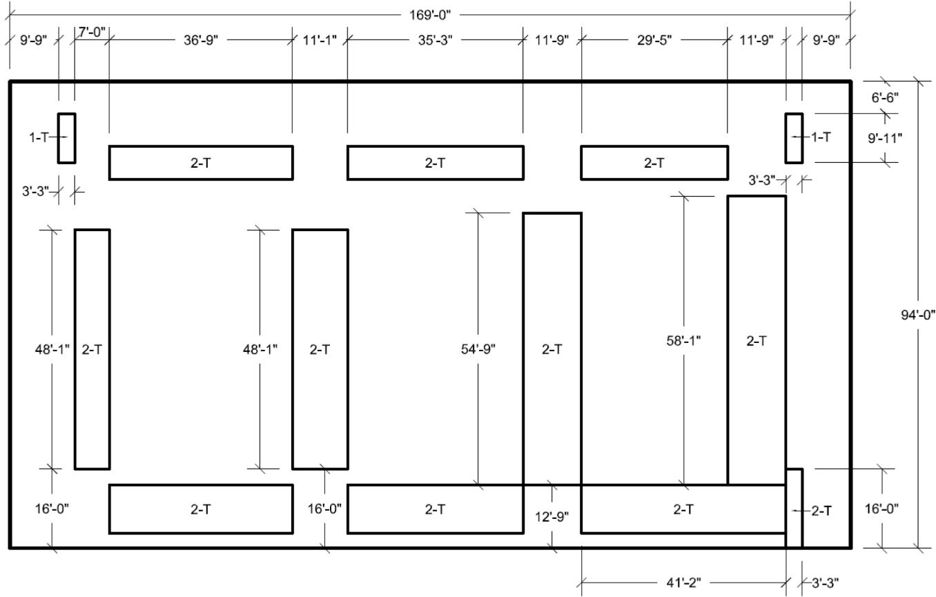
Figure 3H.6-126A Pump House Foundation Mat Transverse Reinforcement Zones
