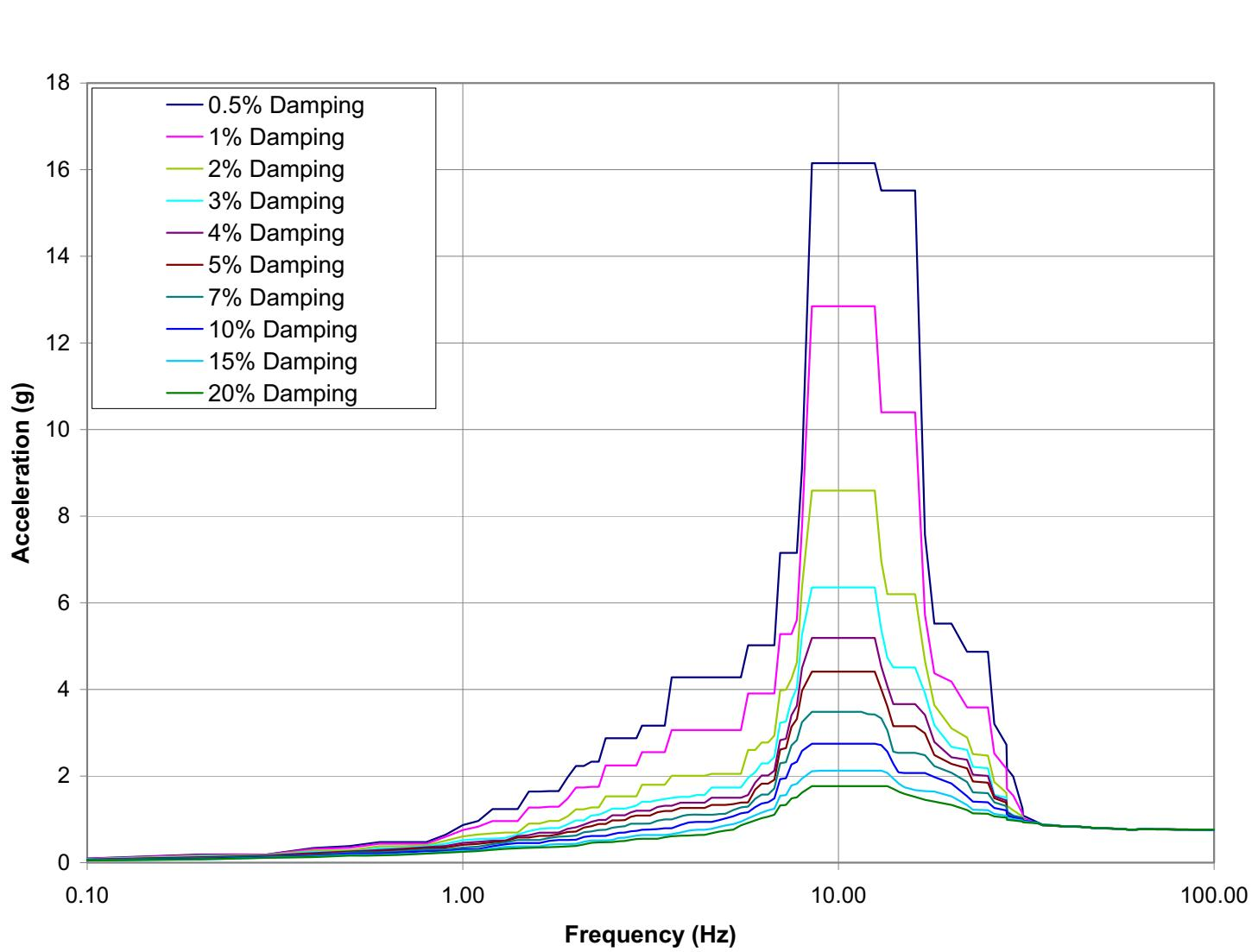
Figure 3H.6-224 Enveloped Broadened Vertical Direction Response Spectra for DGFO SV
