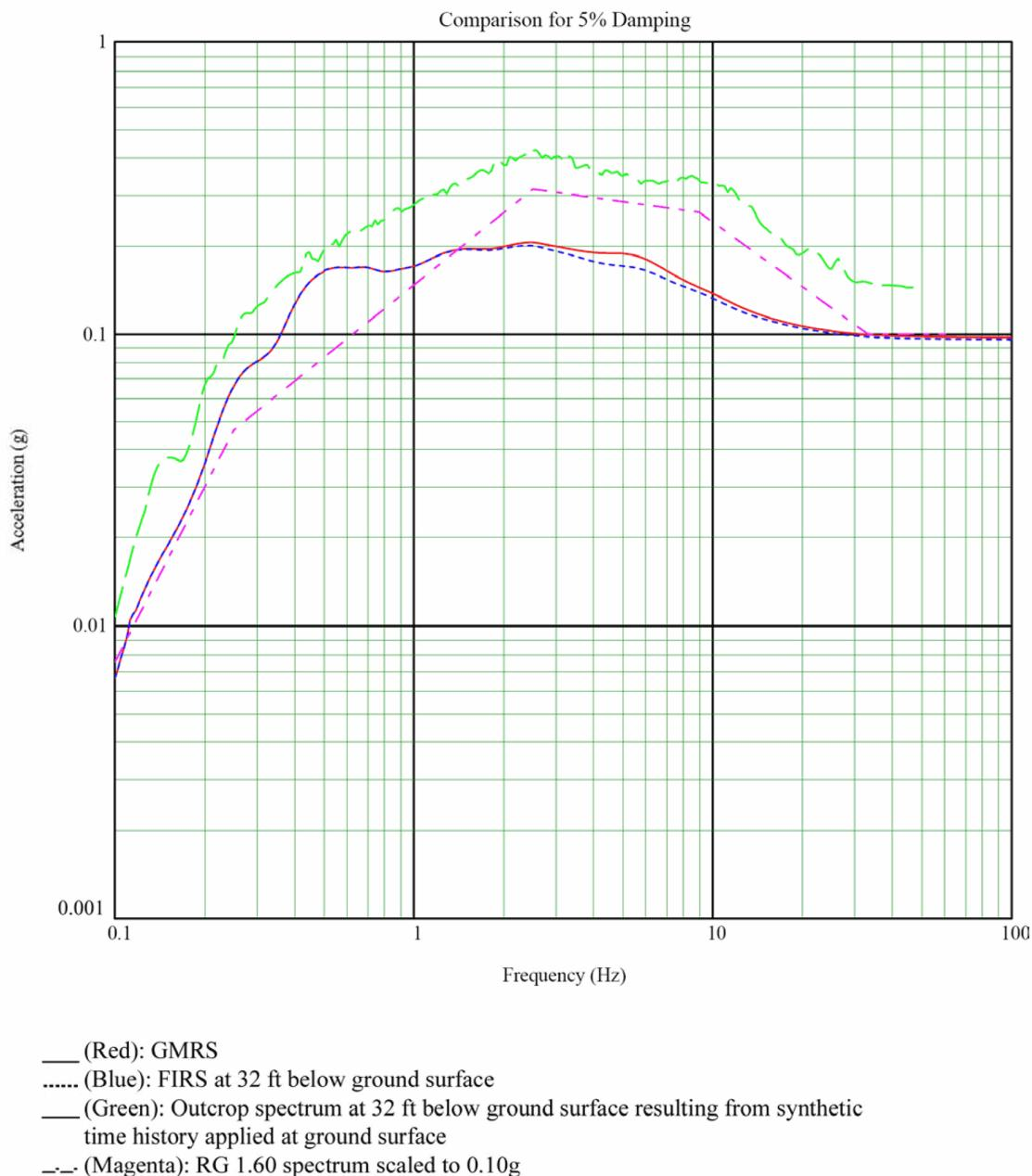
**Figure 3H.6-4a Comparison of Spectra at Foundation of UHS Basin (Mean Soil Properties, N-S Direction)**
