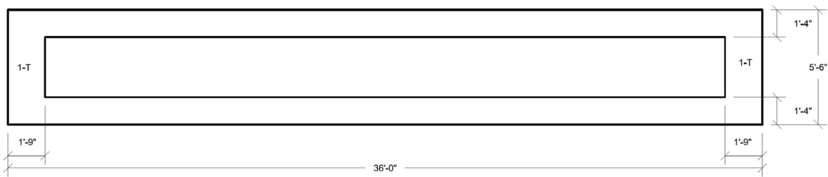
Figure 3H.7-19A Roof of Tunnel Looking Down Transverse Reinforcement Zones
