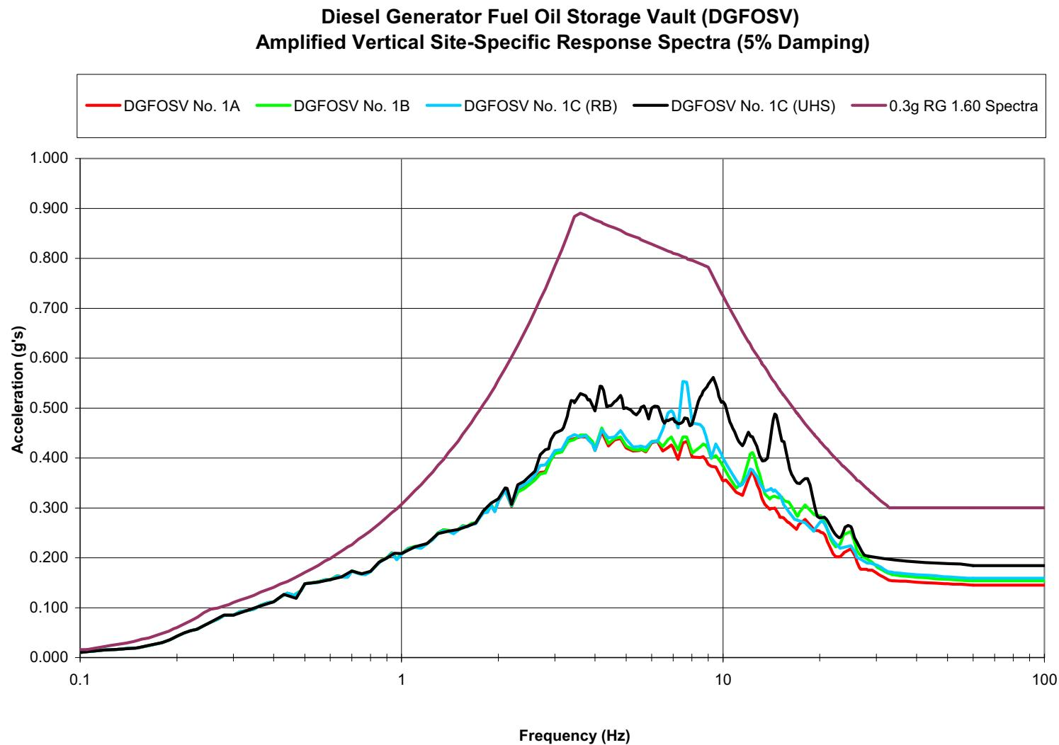
**Figure 3H.6-222c Amplified Vertical Site-Specific Response Spectra
