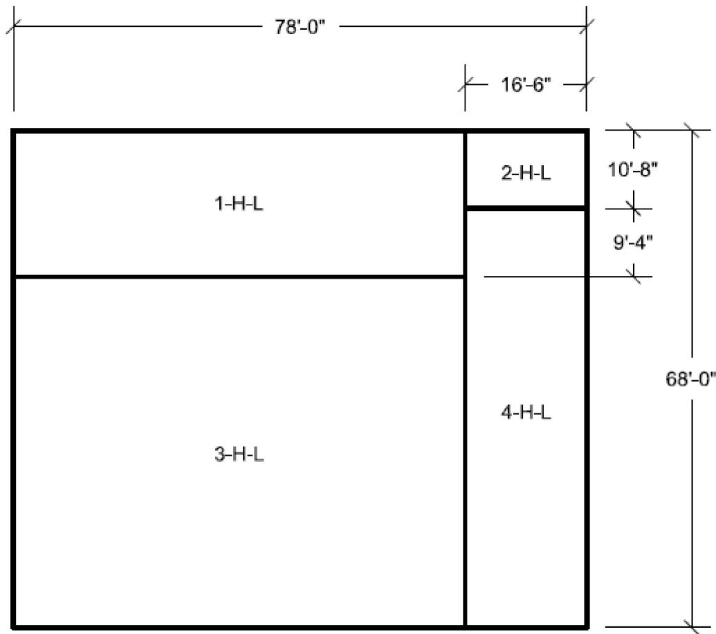
Figure 3H.6-68 Pump House West Wall Looking East Horizontal Reinforcement Zones Far Side Face
