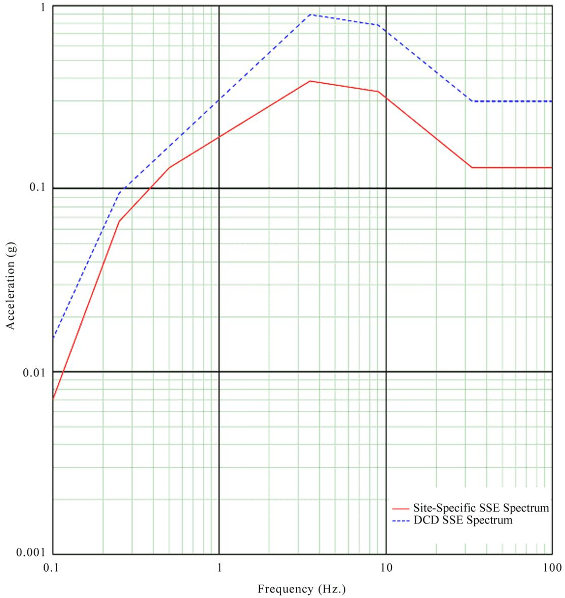
Figure 3A-232a Comparison of Site-Specific SSE Design Spectrum with DCD SSE Spectrum - Vertical (5% damping)
