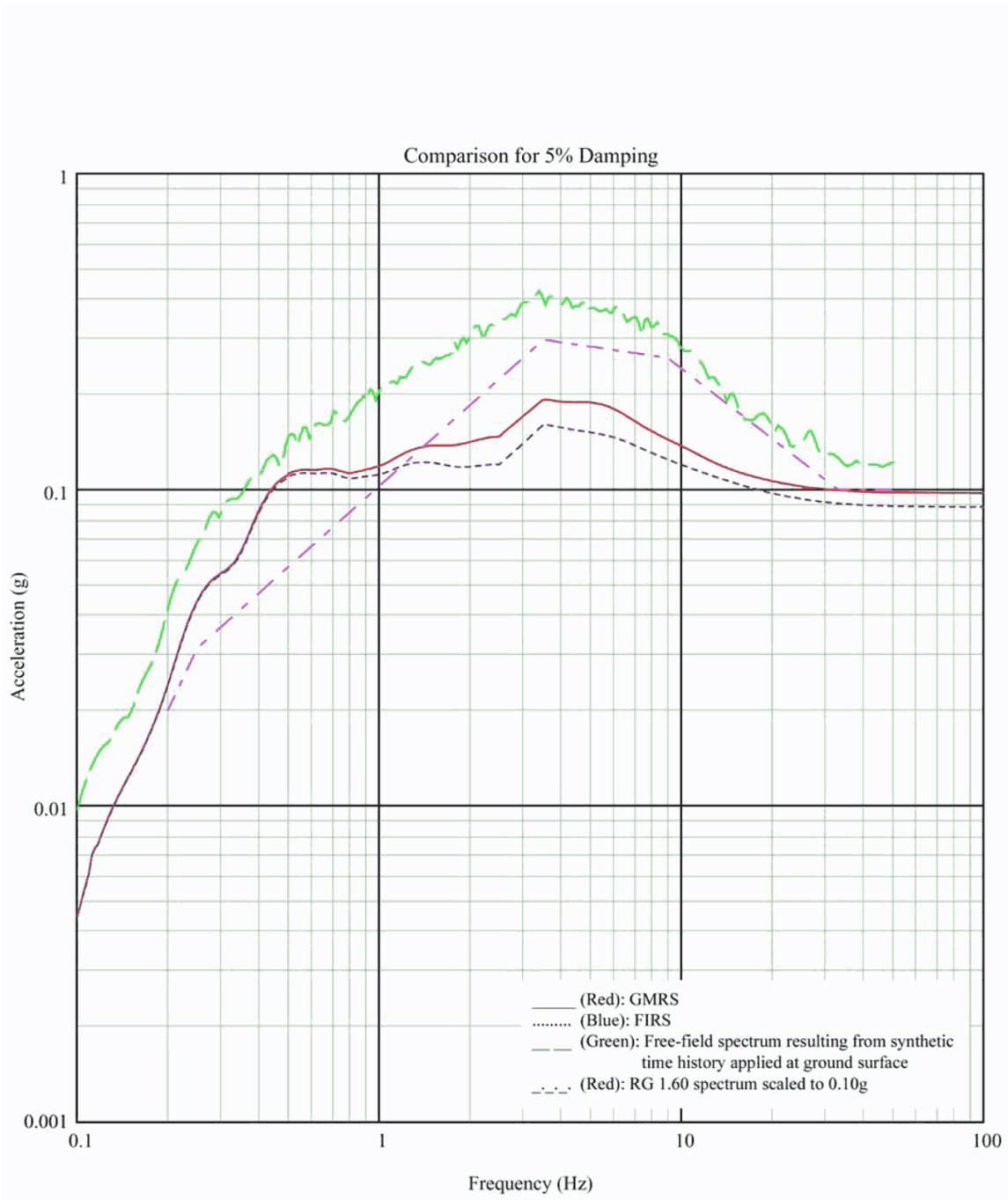
Figure 3A-244 Comparison of Spectra at Foundation of Control Building - Mean Soil Properties, Vertical Direction
