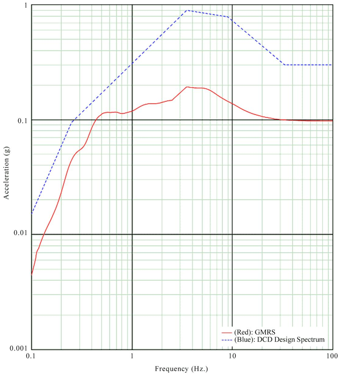
Figure 3A-232 Comparison of GMRS with DCD Design Spectrum (CSDRS) - Vertical (5% damping)
