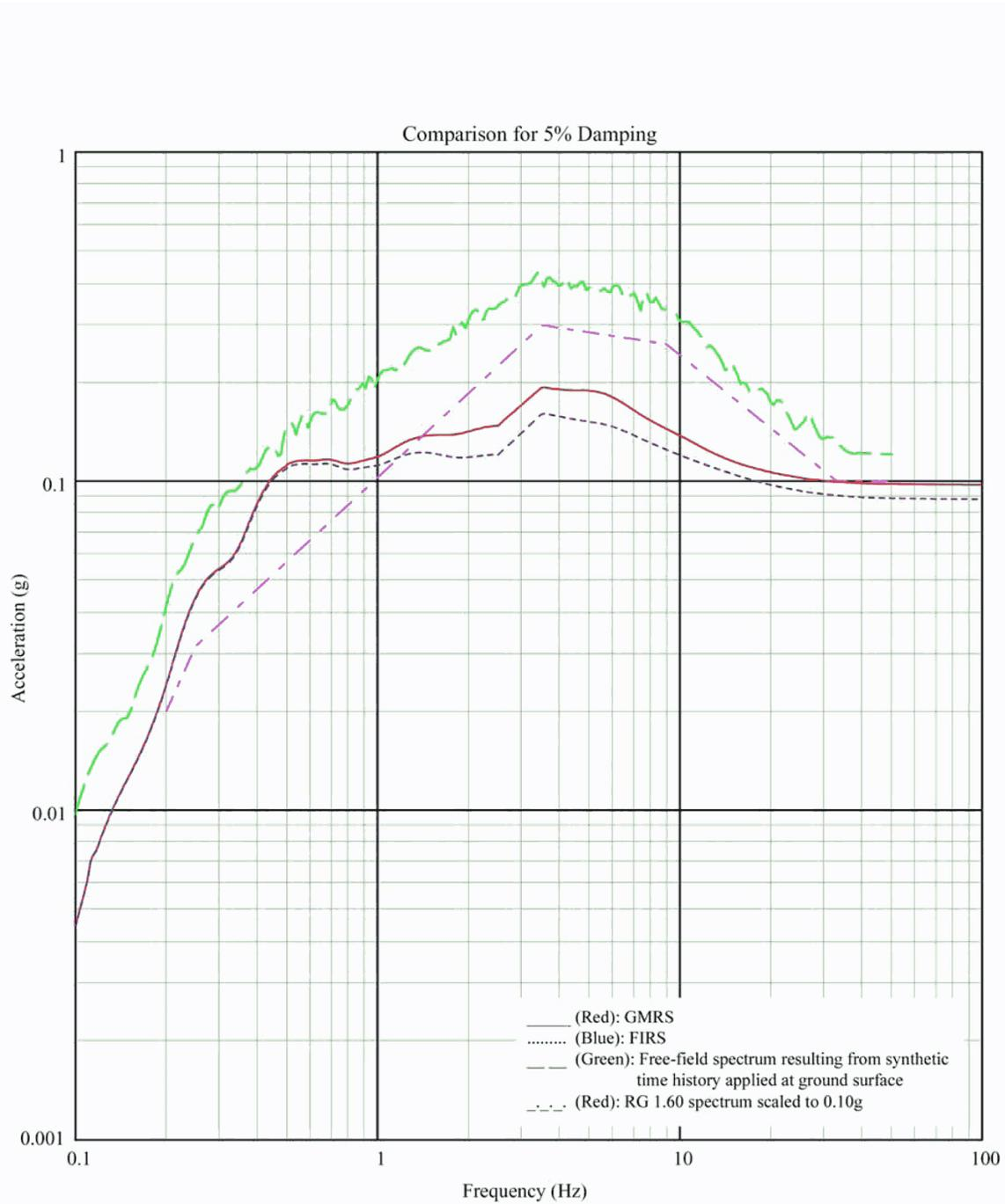
Figure 3A-247 Comparison of Spectra at Foundation of Control Building - Upper Bound Soil Properties, Vertical Direction
