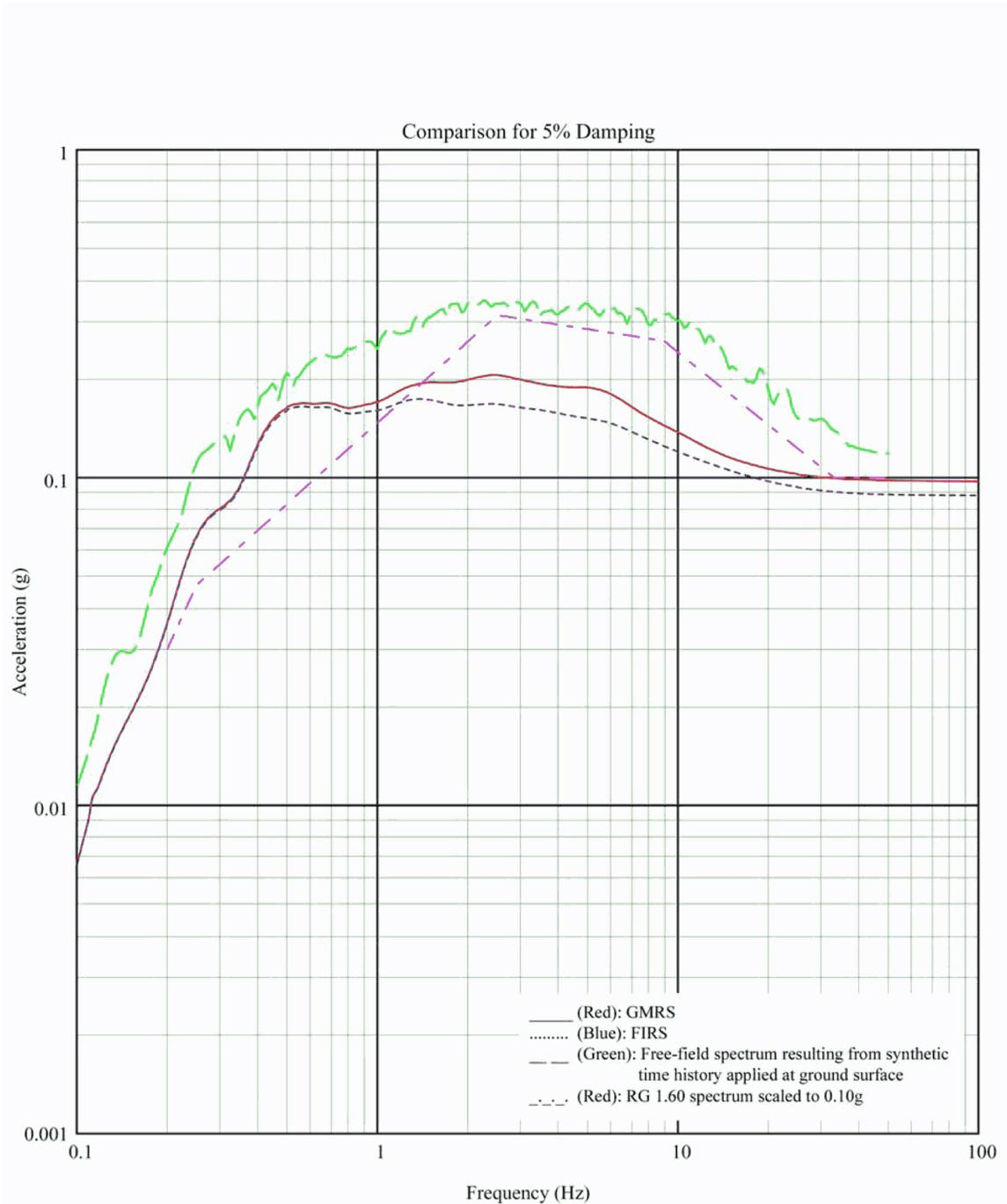
Figure 3A-243 Comparison of Spectra at Foundation of Control Building - Mean Soil Properties, Y Direction
