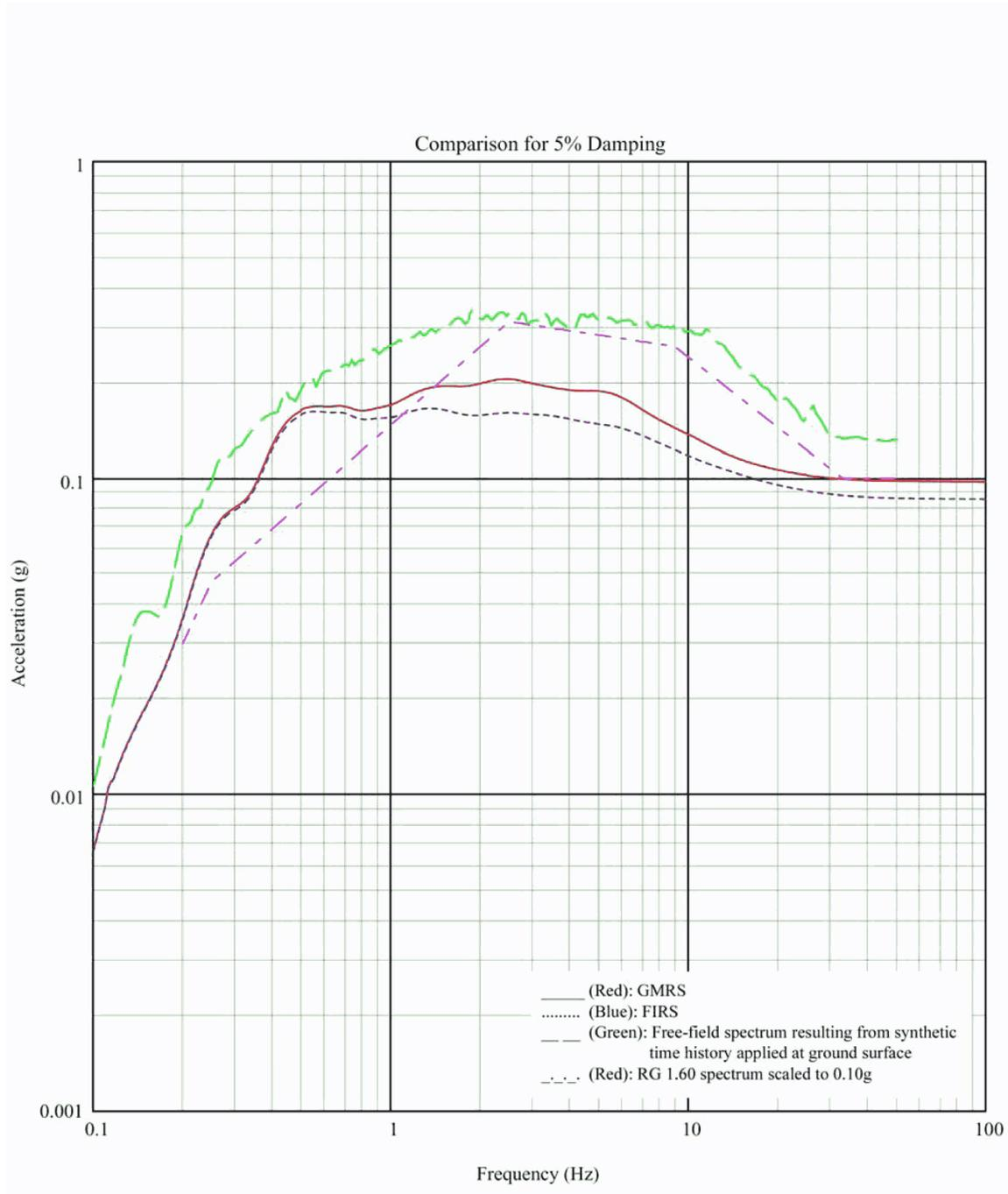
Figure 3A-233 Comparison of Spectra at Foundation of Reactor Building - Mean Soil Properties, X Direction
