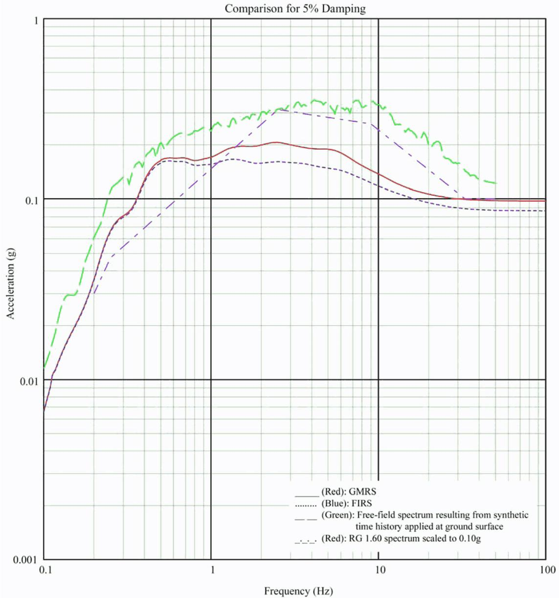
Figure 3A-240 Comparison of Spectra at Foundation of Reactor Building - Lower Bound Soil Properties, Y Direction
