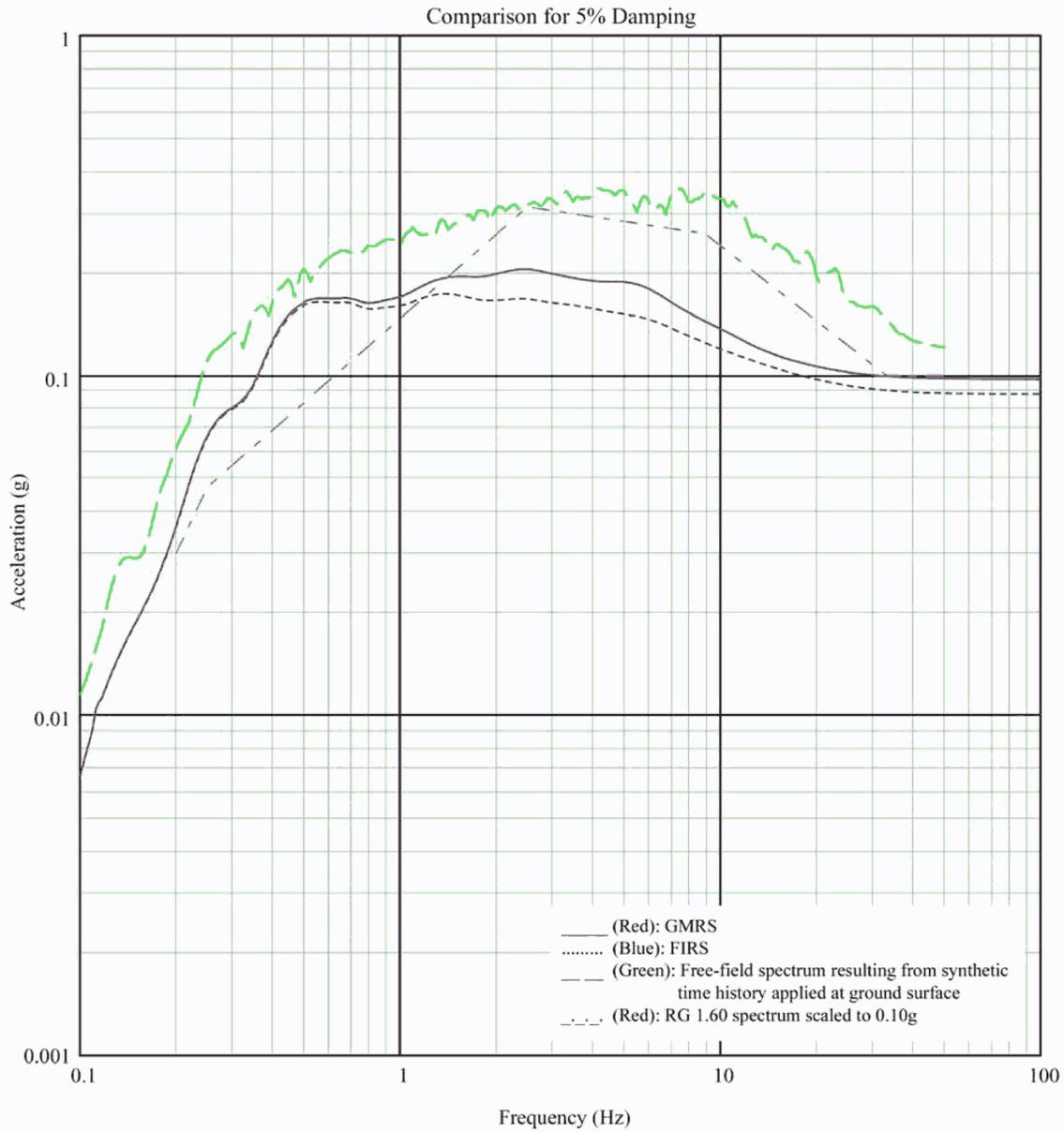
Figure 3A-249 Comparison of Spectra at Foundation of Control Building - Lower Bound Soil Properties, Y Direction
