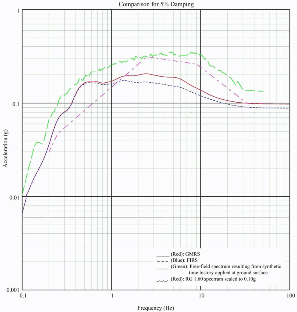
Figure 3A-248 Comparison of Spectra at Foundation of Control Building - Lower Bound Soil Properties, X Direction
