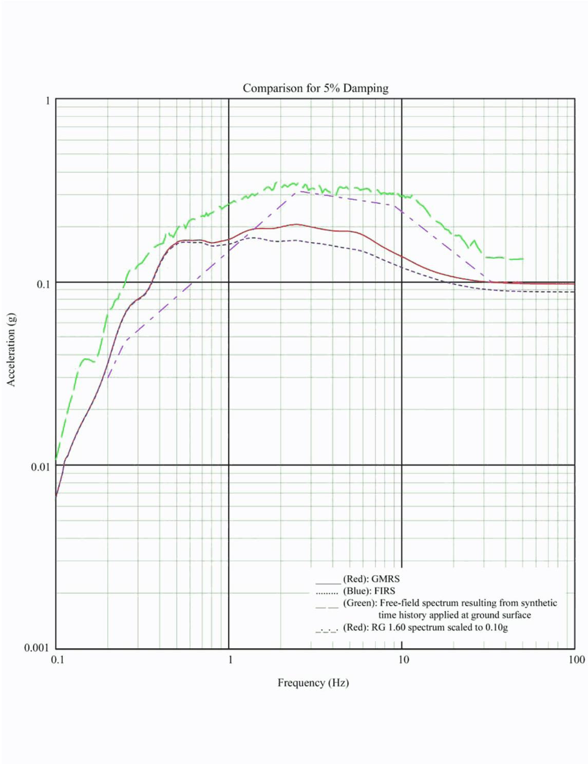
Figure 3A-242 Comparison of Spectra at Foundation of Control Building - Mean Soil Properties, X Direction
