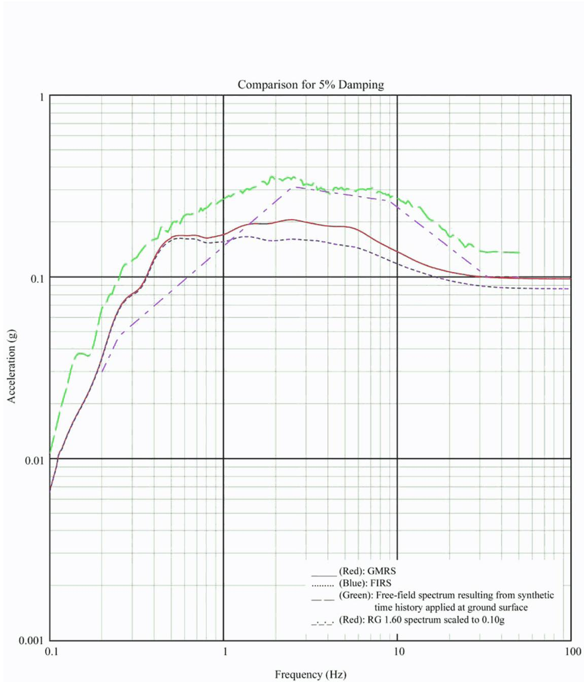
Figure 3A-236 Comparison of Spectra at Foundation of Reactor Building - Upper Bound Soil Properties, X Direction
