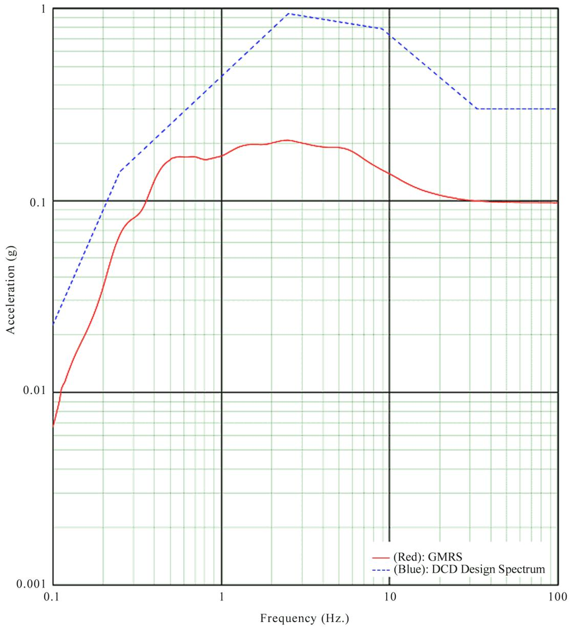
Figure 3A-231 Comparison of GMRS with DCD Design Spectrum (CSDRS) - Horizontal (5% damping)
