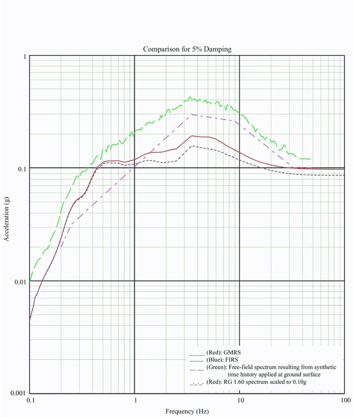
Figure 3A-238 Comparison of Spectra at Foundation of Reactor Building - Upper Bound Soil Properties, Vertical Direction
