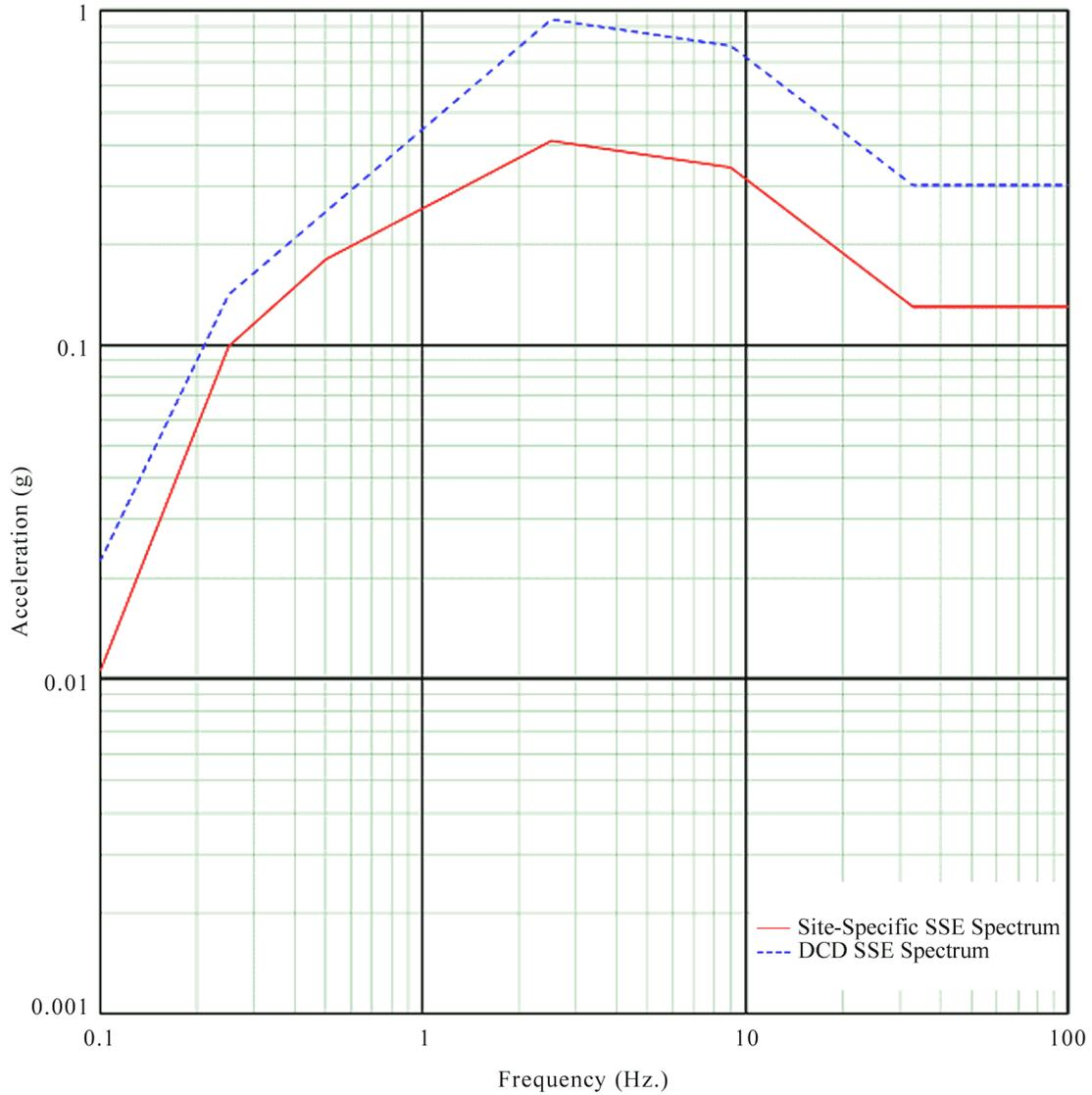
Figure 3A-231a Comparison of Site-Specific SSE Design Spectrum with DCD SSE Spectrum - Horizontal (5% damping)
