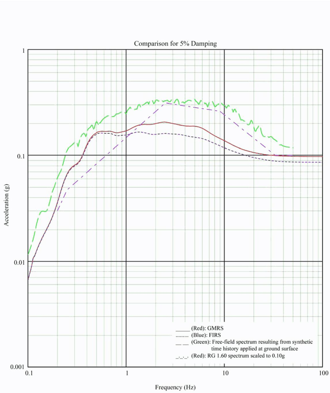
Figure 3A-234 Comparison of Spectra at Foundation of Reactor Building - Mean Soil Properties, Y Direction
