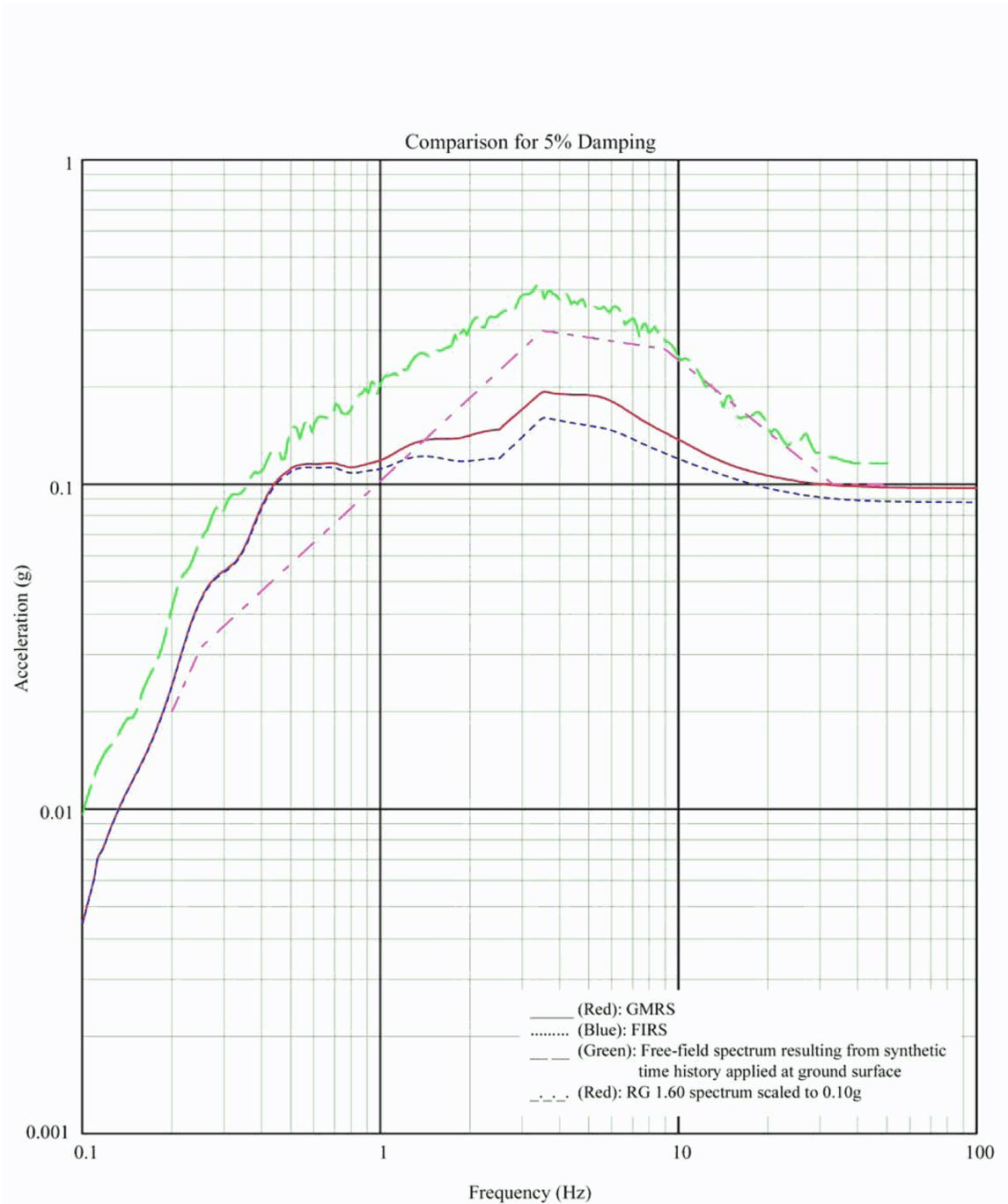
Figure 3A-250 Comparison of Spectra at Foundation of Control Building - Lower Bound Soil Properties, Vertical Direction
